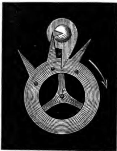
so escapes, and at the same time one of the pins catches the long tooth projecting from the verge, and gives the impulse.
