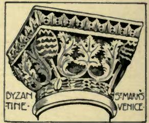
The Byzantine capitals have the square abacus, usually consisting of a simple fillet and chamfer enriched with the billet, dentil or star pattern. The Dossieret, a singular adjunct to the capital, was introduced during this period; it was a cushion-shaped or cubical stone placed upon the abacus of the capital to give additional height (plate 11).
