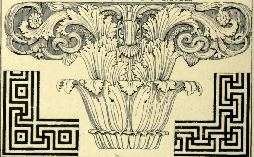
development, was the scroll given on plate 6, which is a fine example from the roof of the monument to Lysicrates. The scrolls, cut with V-shaped sections, spring from a nest of sharp acanthus foliage. This scroll is formed of a series of spirals springing from each other, the junction of the spiral being covered by a sheath or flower; the spiral itself being often broken by a similar sheath.
