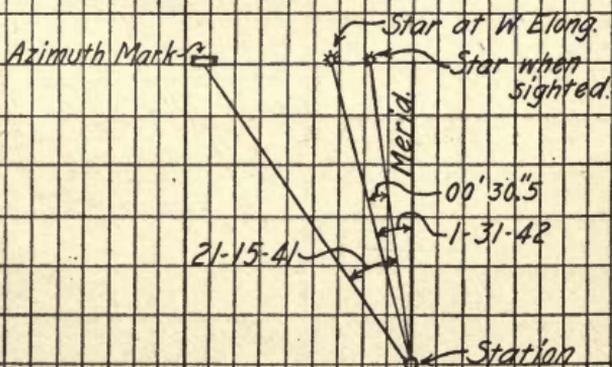
Azimuth by Polaris "at any Hour Angle."
