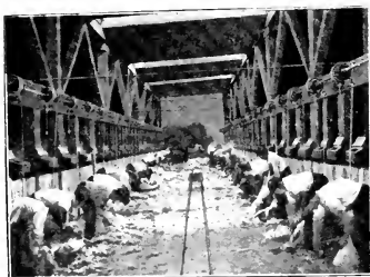
SHEARING PLANT, USING STEWART SHEAR. Made by Chicago Flexible Shaft Co., Chicago.
