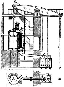
Fig. 101.—Cornish Pumping-Engine, 1878. Section.
