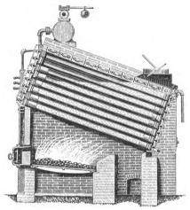
Fig. 113.-Root Sectional Boiler.
