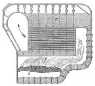
Fig. 142.-Marine Fire-tubular Boiler. Section.
