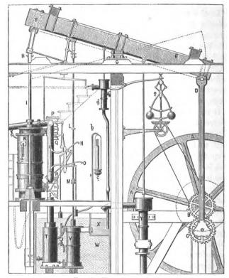
Fig. 27.-Watt's Engine, 1781.
