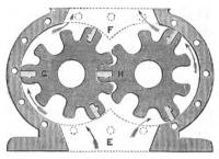
Fig. 124.-Rotary Pump.
