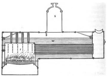
Fig. 109.—Stationary "Locomotive" Boiler.
