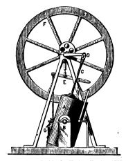
Fig. 86.—Murdoch's Oscillating Engine, 1785.
