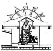
Fig. 181.—Oscillating Engine and Feathering Paddle-Wheel,
