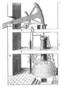
Fig. 20.—Beighton's Valve-Gear, A. D. 1718.
