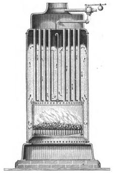
Fig. 108.—Bahcock & Wilcox's Vertical Boiler.
