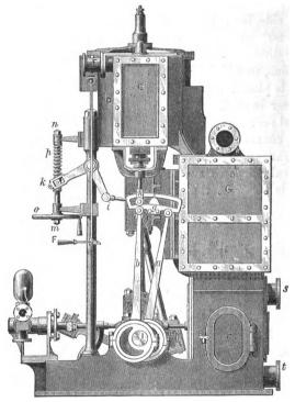
Fig. 187.-Compound Marine Engine. Side Elevation.
