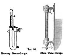
To determine the height of water in his boiler, Watt added to the gauge-cocks already long in use the "glass water-gauge," which is still seen in nearly every well-ar-
