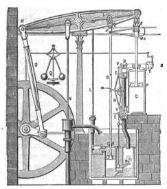
Fig. 81.—Boulton & Watt's Double-Acting Engine, 1784.
