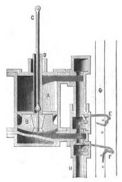
Fig. 88 .- Watt's Half-Trunk Engine, 1784,
