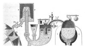
Fig. 18.—Papin's Engine and Water-Wheel, A. D. 1707.
