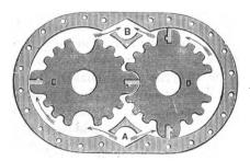
Fig. 128.-Rotary Steam-Engine.
