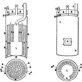
Fig. 73,-Read's Boiler in Section, 1788,
