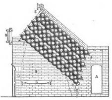
Fig. 111.—Harrison's Sectional Boiler.
