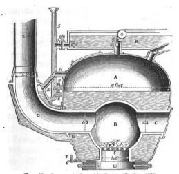
Fig. 28.—Smeaton's Portable-Engine Boiler, 1765.
