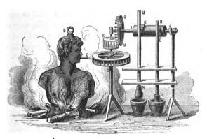
Fig. 6.—Branca's Steam-Engine, A. D. 1629.
