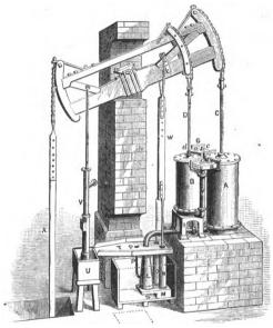
Fig. 87.—Hornblower's Compound Engine, 1781.
