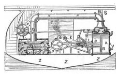
Fig. 186.-Horizontal, Direct-acting Naval Screw-Engine.
