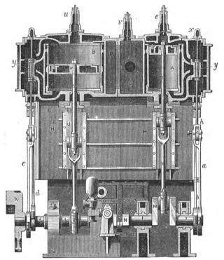
Fig. 138.—Compound Marine Engine. Front Elevation and Section.
