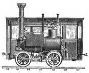
Fig. 125.—Tank-Engine, New York Elevated Railroad.
