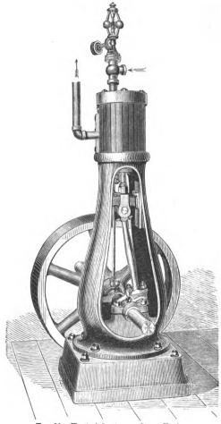
Fig. 93.-Vertical Stationary Steam-Engine.
