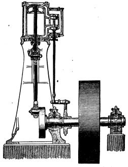
Fig. 94.—Vertical Stationary Steam-Engine. Section.
