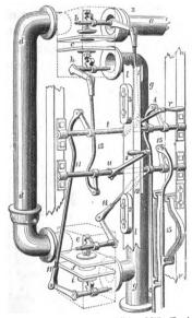
Fig. 32.—Valve-Gear of the Albion Mills Engine.
