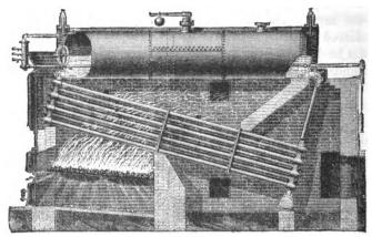
Fig. 112.—Babcock and Wilcox's Sectional Boiler.
