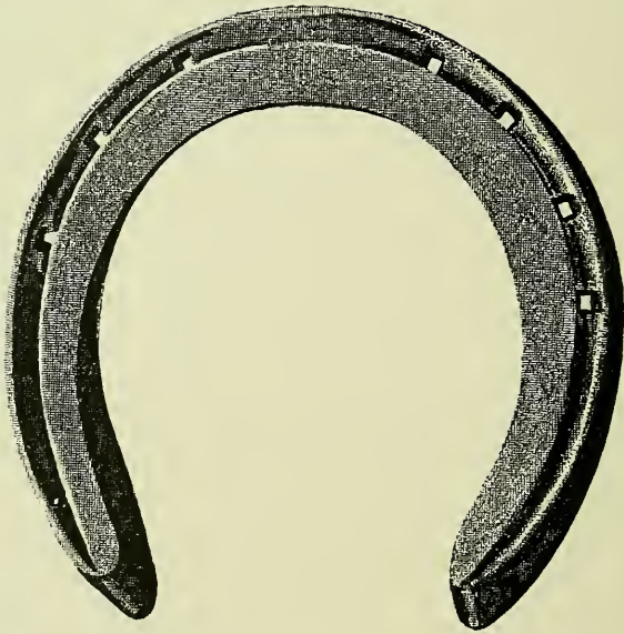
FIG. 211.—Fullered seated fore shoe with thick heels. Made of \frac{7}{8} \times \frac{5}{8} inch iron.
