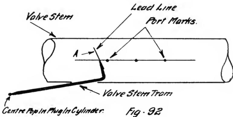
All dead centres can be found with the use of a tram in this manner and can be relied upon, providing the crosshead is moved to the end of its travel, the position of which corresponds with the dead centre being found and the line through centre of crosshead wrist pin being scribed to suit each dead centre as before detailed in the example just given.
