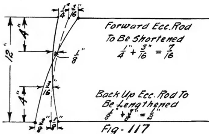
Determine the link lifter length adjustment required to equalize the hook up valve travels last figured.
