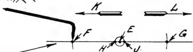
Port Marks As They Occur When Valve Is In Position Above Shown
