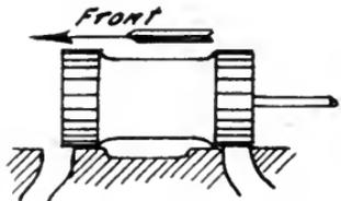
Inside Admission Valve Exhaust Clearance Given Valve On Point Of Release Or Exhaust Cut Off At Back Port.
