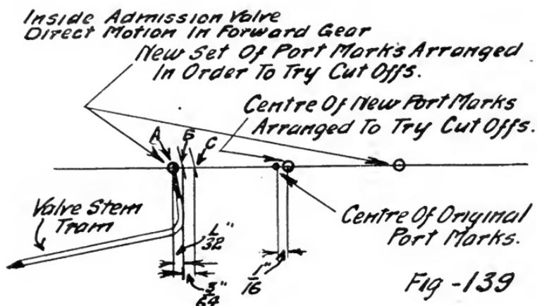
Move drivers around again in a forward direction until another  $5/8$ " is tacked onto the back cut off in forward gear, then stop. The crosshead is now  $23-7/8$ " from the beginning of its stroke.
