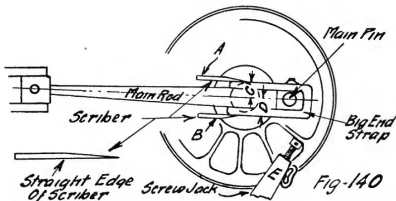
Measure the distance "C" to see if it equals the distance "D." If not, apply a jack (to slip the driving wheels) as shown at "E" until "C" equals "D," both being measured from the centre of driving axle.
