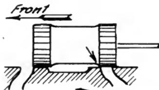
Inside Admission Valve On Point Of Admission Or Point Of Cut Off At Back Port.
