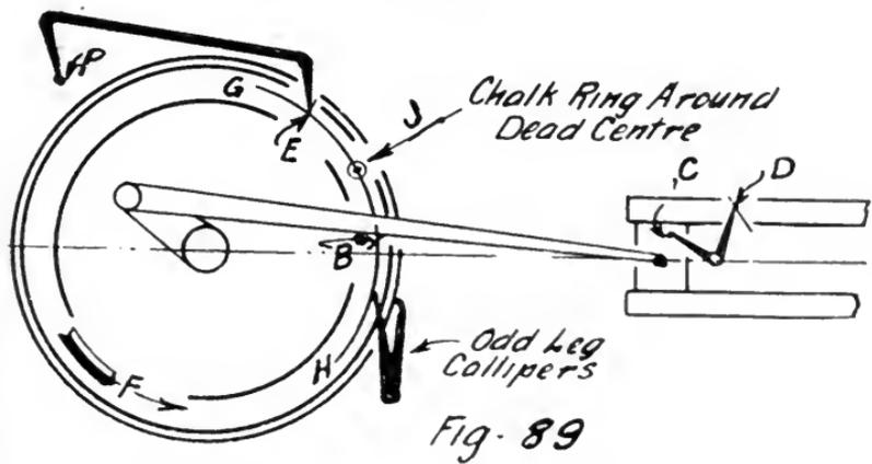
a better opportunity to keep an eye on anybody attempting to or actually moving reverse lever from the proper notch in its rack without notifying the valve setter. Movement of a reverse lever will often cause a false reading to be taken. The position of a reverse lever in its rack does not matter when finding dead centres. It is, however, of great importance to have the reverse lever in the corner notches when catching dead centres to take lead lines.
