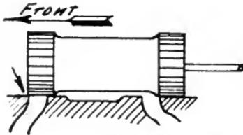
Outside Admission Valve On Point Of Admission Or Point Of Cut Off At Front Port.
