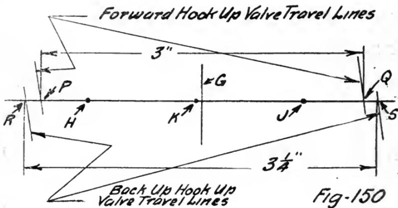
If we consider an inside admission valve the motion is direct in forward gear which means the eccentric rod would have to be lengthened in our example.
