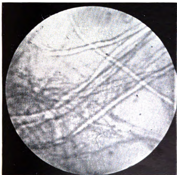
FIG. 12.—MANILLA AND COTTON \times 122 .
