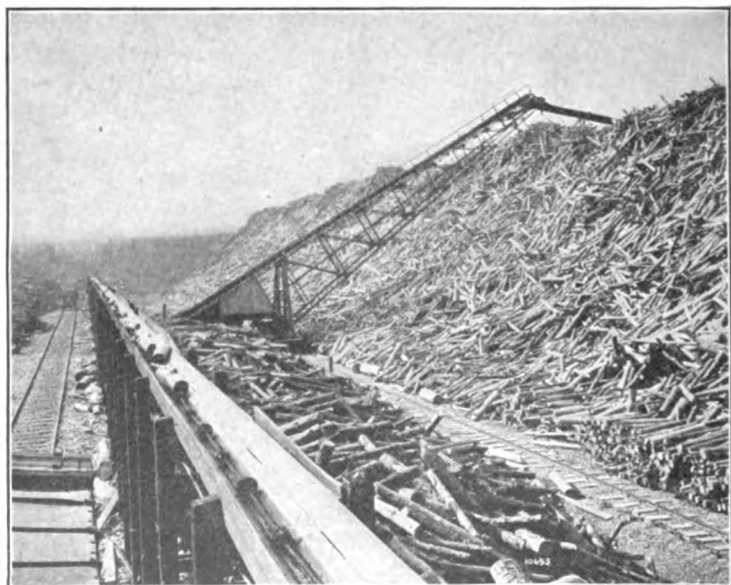
Fig. 25. —Another view of a portable pulp wood stacker showing barked wood stored and unbarked wood waiting to be barked.
