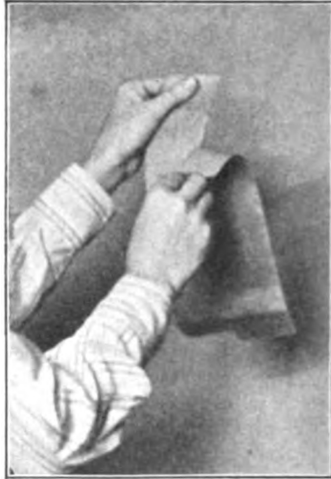
Fig. 187.—Photograph showing manner in which fibres peel when a sheet of wrapping paper is torn naturally by the hands.
