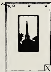
2. Tracing reversed and fastened to block by thumb tacks. Pin in X. Lower corner creased up showing slanting register mark, which is scratched into block. Paper is shown slightly smaller than block.
