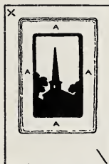
3. Block after cutting. All white parts are hollowed out. All printing parts are left standing. A margin space about \frac{3}{4} " wide, is hollowed out. Note X and slanting register marks.
