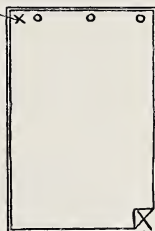
4. Sheet of paper on block ready for printing. Pin locates upper register mark. Lower corner is creased over and slanting line on block marked on paper. Upper edge of paper then fastened with tacks. Paper is shown slightly smaller than block.
