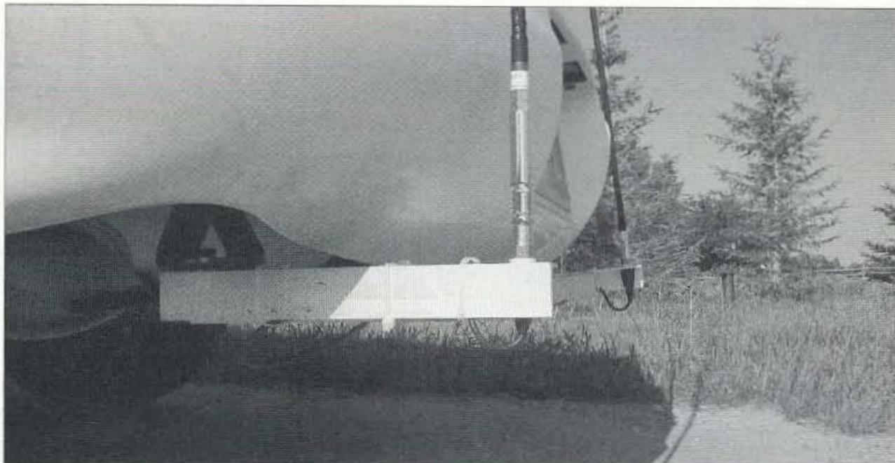
**Photo B.** When faced with a tall antenna and a plastic bumper, one option is to construct an extension that mounts to the automobile frame and extends just beyond the bumper. The extension here is mounted to the support normally used to connect to the jack used to change tires. The cable ties keep the coax in place.
