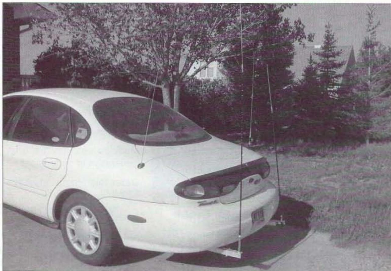
**Photo A.** Fashion experts say that the multiple antenna look is "in" this year. Besides the 2-meter/440-MHz antennas glass-mounted and on the trunk, there's an Iron Horse 6-meter antenna on the right and a matching 20-meter antenna on the left.
