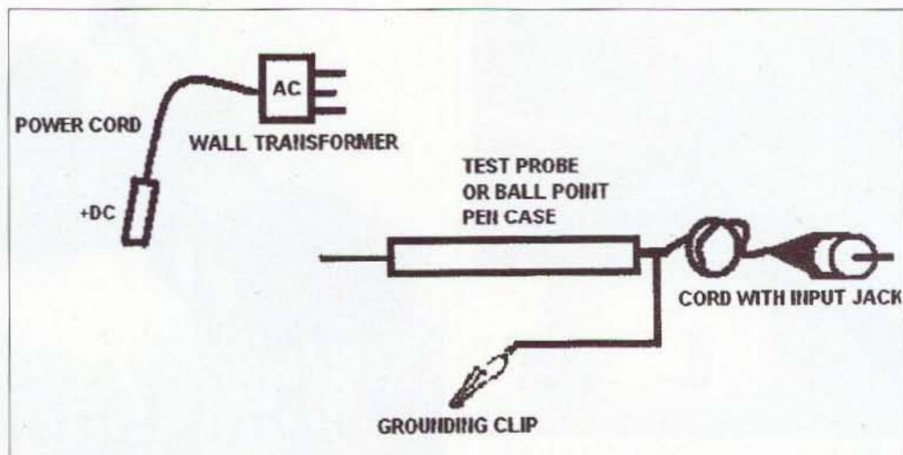
Fig. 2. Attachments, DC power source and modified audio cable with test probe attachment.
