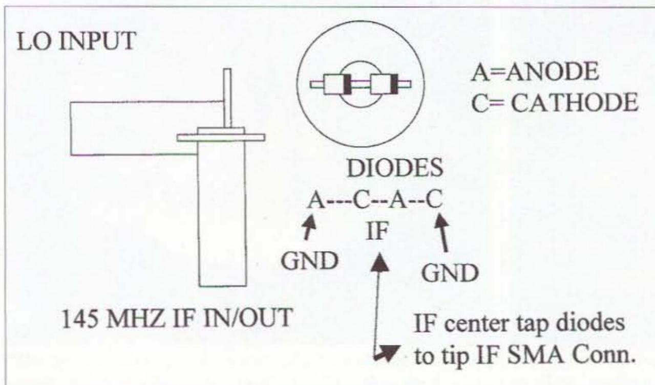
Fig. 1. Showing mixer construction/placement of microwave diodes on back of SMA bulkhead connector. Use shortest possible lengths. Used bare mixer for demo on 47 GHz for short SSB contact at club meeting SDMG San Diego Microwave Group.
