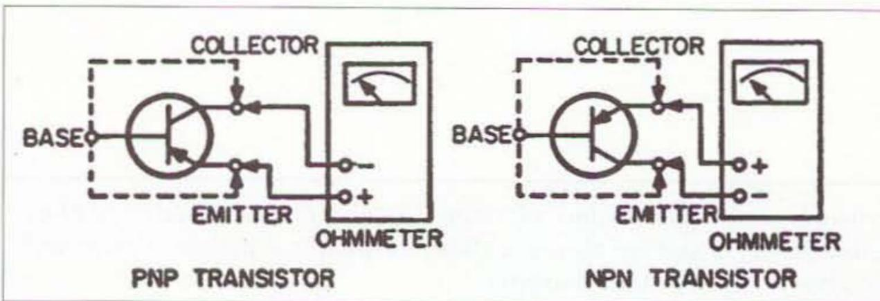
Fig. 3. With ohmmeter in  $R \times 100$  scale (assuming that the meter uses a 1-1/2 volt battery), a good transistor will be indicated by a decrease in resistance when the base lead is touched to the collector and a small increase in resistance when the base lead is touched to the emitter.
