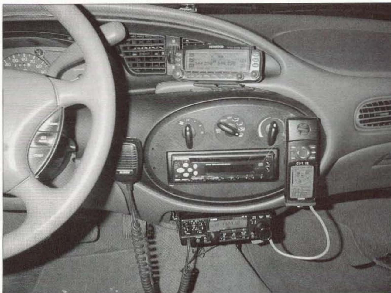
*Photo A. With the new HF rig installed, I have access to the “low bands” for DX as well as 6 meters, just for fun. The ashtray mount was almost a perfect fit for the Alinco DX-70T.*
