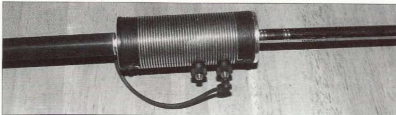
Photo D. The Buddipole's large loading coil.
