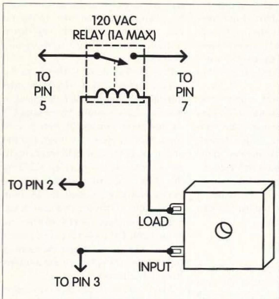
Fig. 2. Simplified wiring scheme. Pin 2 and Pin 3 refer to socket K202.
