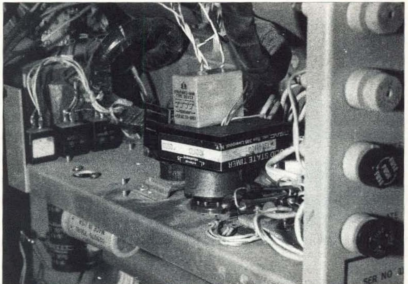
**Photo A.** A view of the replacement time delay module. Note the module overhang above the diodes. You'll need clearance for K203 (barely visible) to the rear of the timer package. The wires above the 120 VAC [see text note in column 1 re 120 VAC] ice cube-type relay are connected to a second set of normally open contacts on the relay and will eventually control voltage to the two bulbs behind the plate and antenna tune dials. See text for details.
