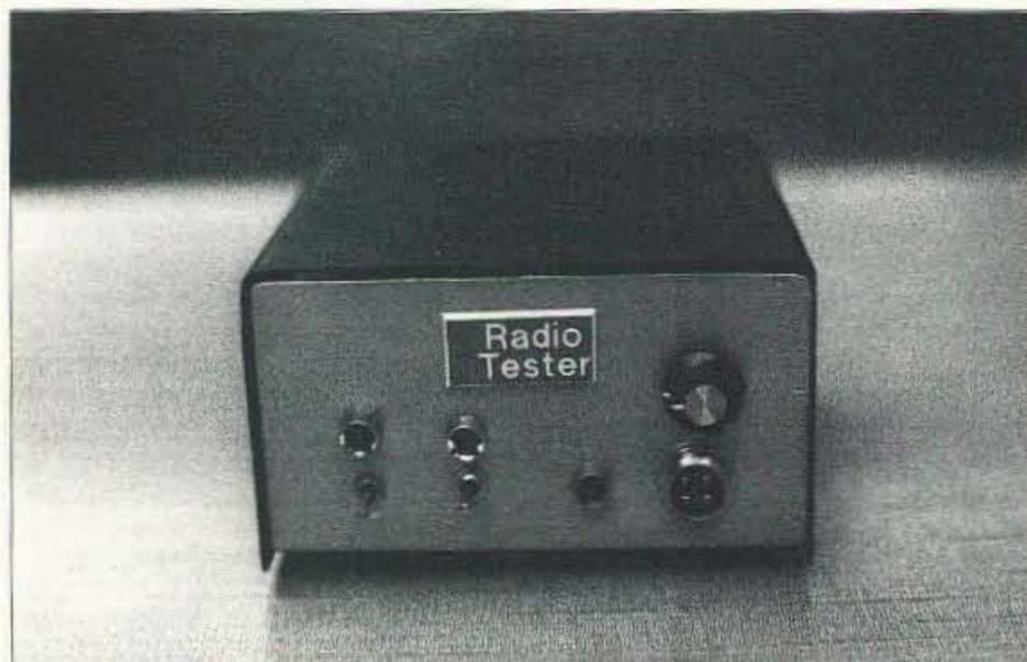
**Photo A.** The final version of the radio tester. The switch on the far left is the power switch; S1 and S2 on the schematic have been combined to a center-off switch (3P3T). The speaker jack is on the side; cable to the transceiver comes out the rear, with the power cable.
