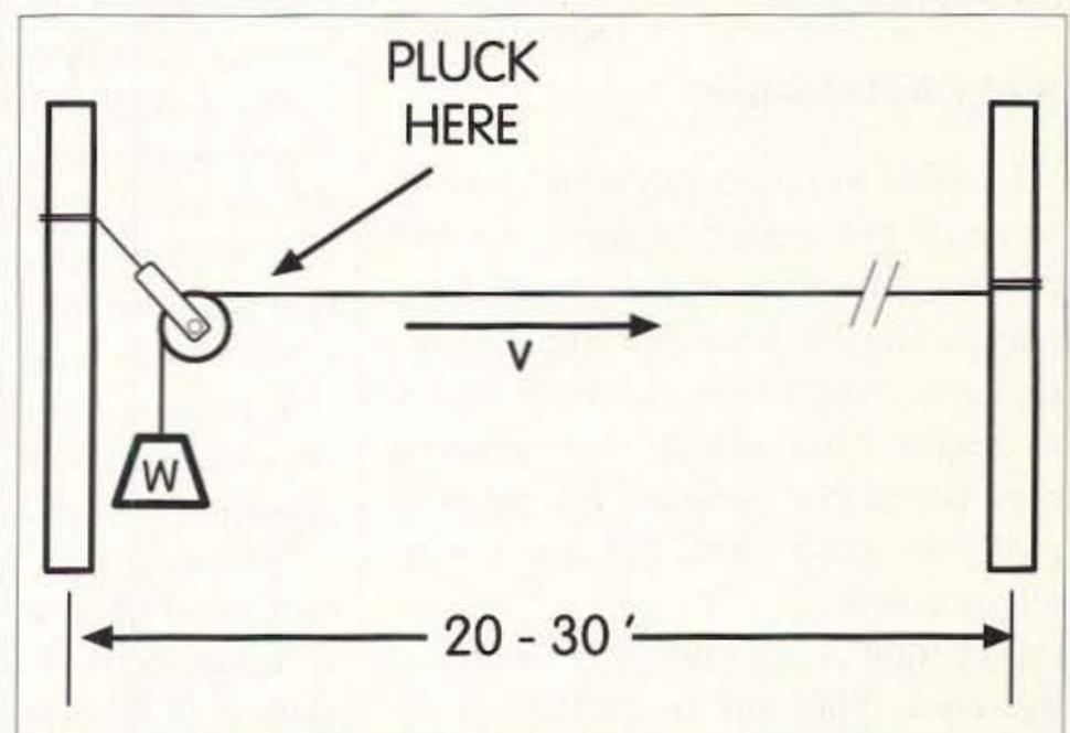
Fig. 1. Traveling waves. Wave velocity is  $\sqrt{(T/W)}$  meters/sec, where  $T$  = tension in newtons and  $W$  = mass of cord in kg/m.
