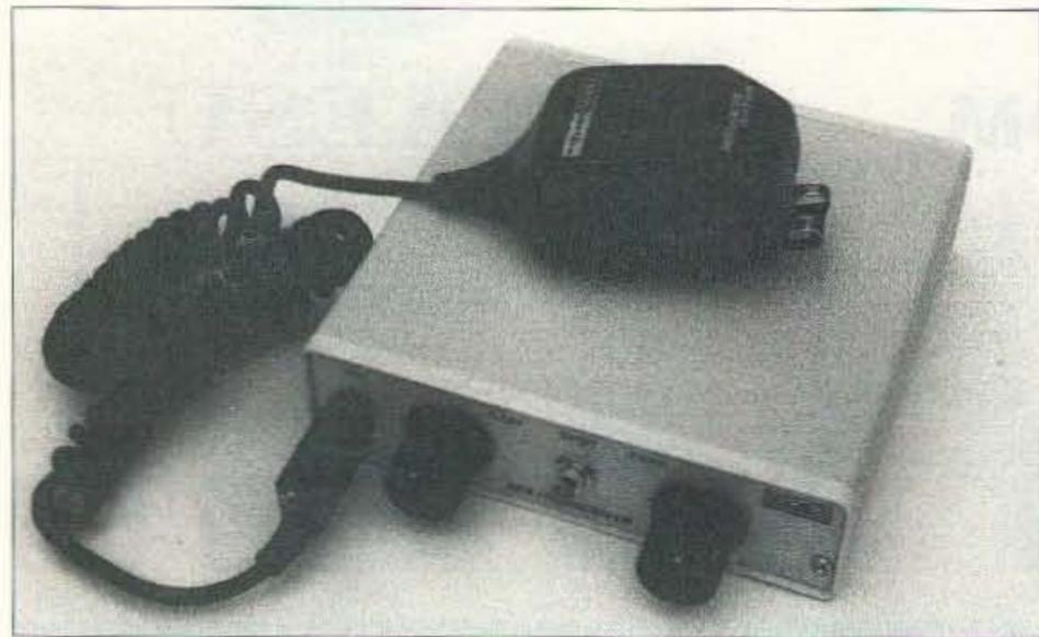
Photo B. The finished WM-20 SSB transceiver.
