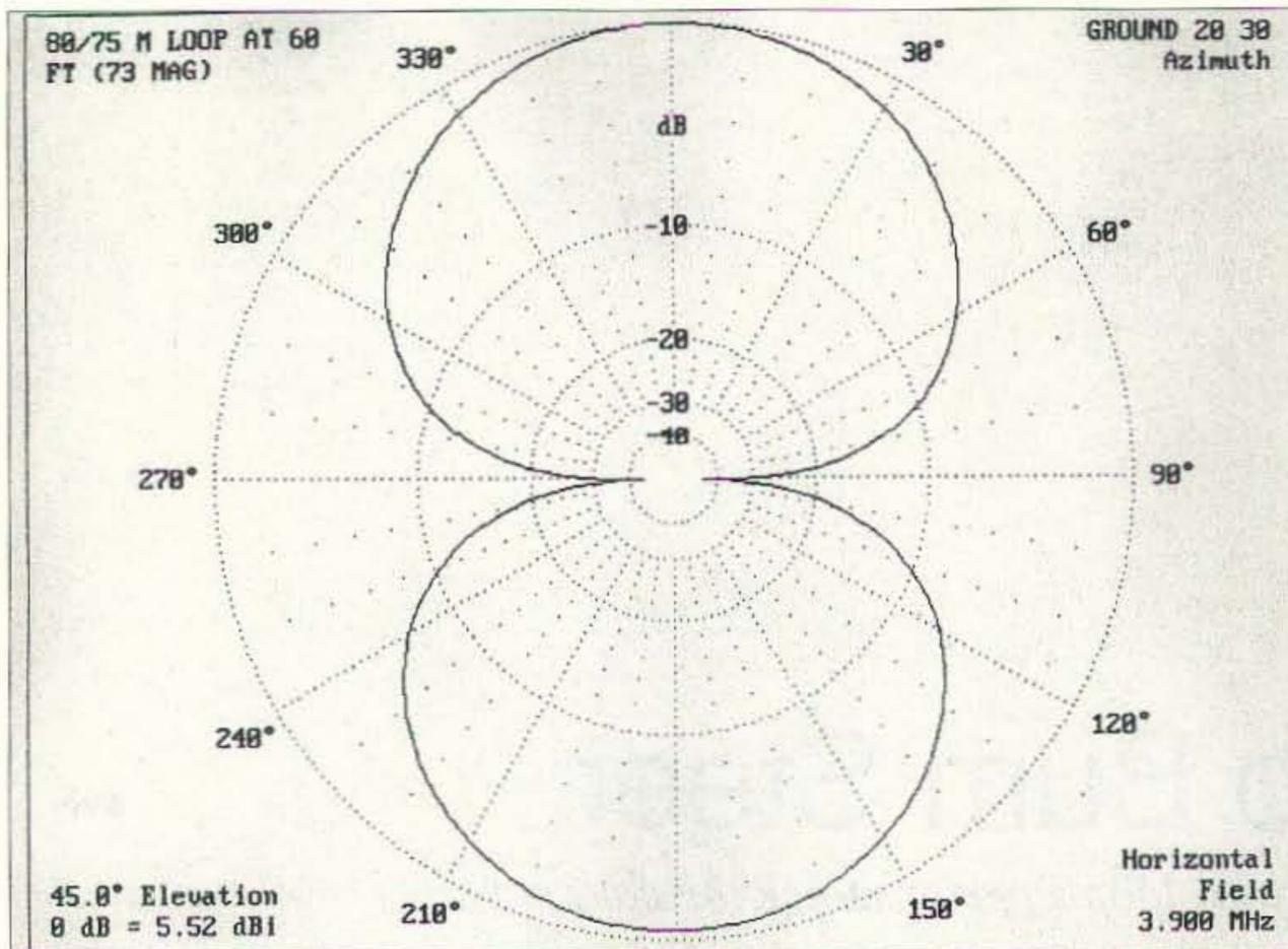
Fig. 2. Loop fed at A or C.
