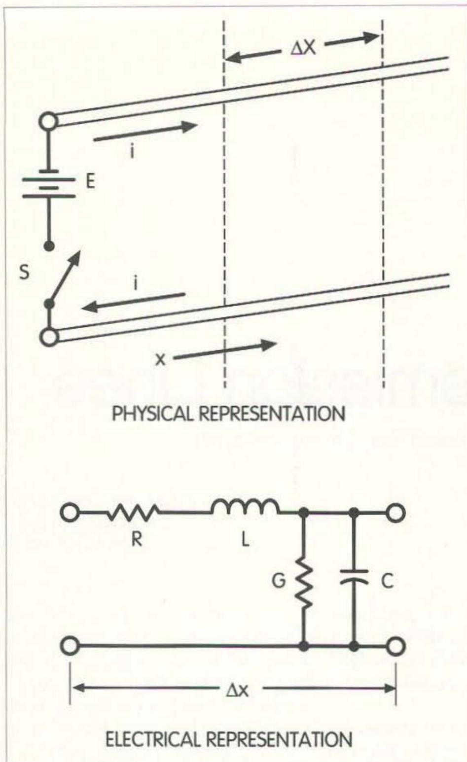
Fig. 2. Physical and electrical representations of an infinitely long electrical line consisting of two parallel conductors.  $R$  = resistance in ohms per unit length.  $L$  = inductance in henrys per unit length.  $G$  = conductance in siemens (reciprocal ohms) per unit length.  $C$  = capacitance in farads per unit length.
