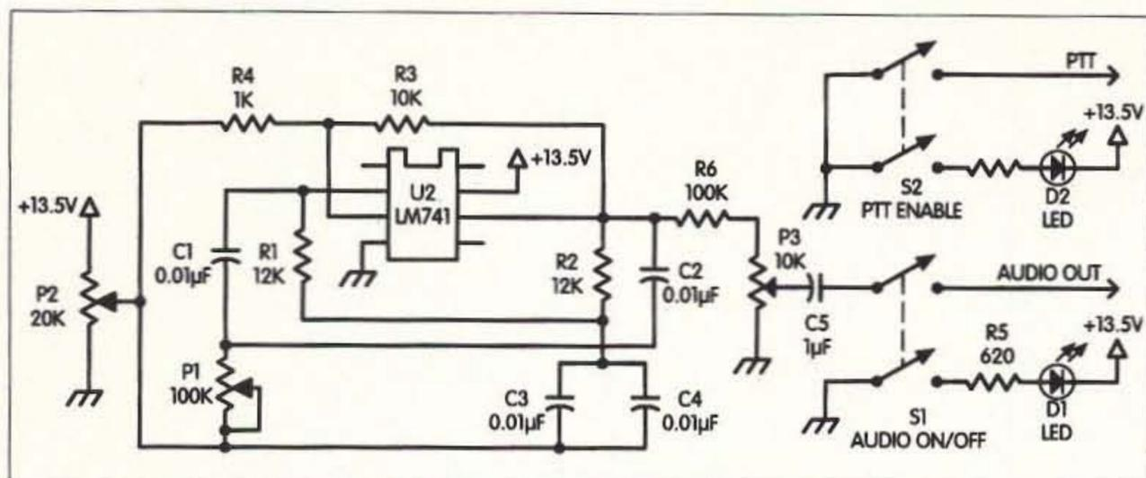
Fig. 1. Transmitter tester. Unlabeled resistor near S2 is R7, 620 ohms.
