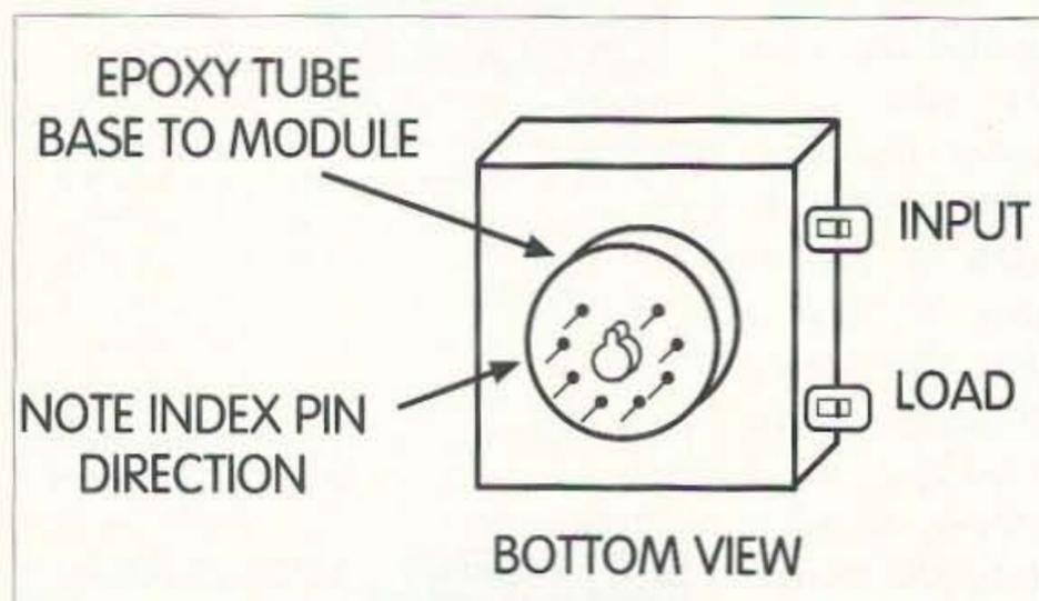
**Fig. 4.** Location of hollowed out octal tube base prior to bonding to timer module with epoxy. Positioning is vital to ensure clearances on relay shelf. Note the position of the indexing pin with respect to the fast-on connectors on the module.
