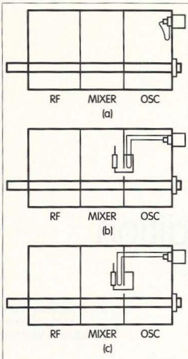
**Fig. 5.** Typical locations for sense loop trials when this scheme is used. (a) Shows a short loop placed in the I field close to a wall. (b) The pickup loop is extended and placed next to or over the diode injection loop. (c) The extended pickup loop is placed close to/over the diode.
