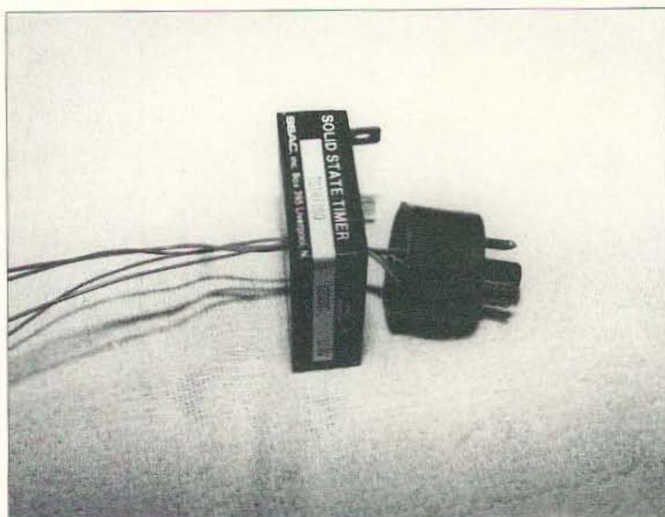
**Photo C.** Two pair of color-coded wires have been soldered to the appropriate pins of the socket. After passing the lengths of wire through the hole in the center of the timer module, epoxy the socket in place. See the instructions for correct positioning to ensure clearances.
