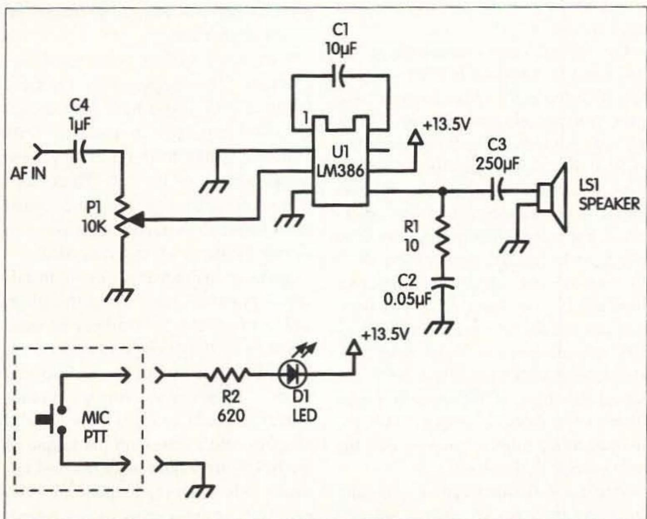
Fig. 2. Microphone tester.
