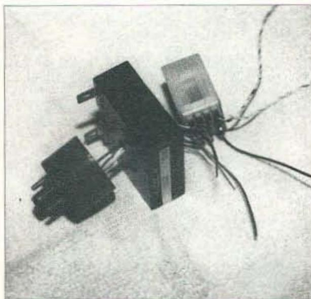
**Photo D.** An "exploded" view of the component parts. Note the two fast-on connectors. Epoxy the socket base and relay to the module. The pair of striped wires in the upper right will control the two bulbs behind the plate and antenna tune dials.
