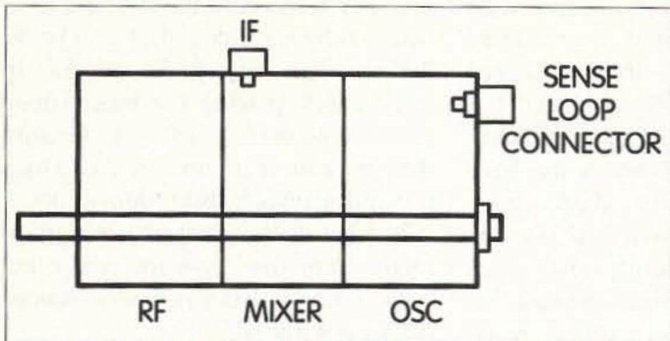
Fig. 2(a). Suggested mounting location of the sense loop connector.
