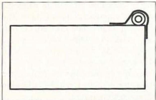
Fig. 2(b). Increasing the mechanical rigidity of the connector by soldering a wire over the mounting portion.
