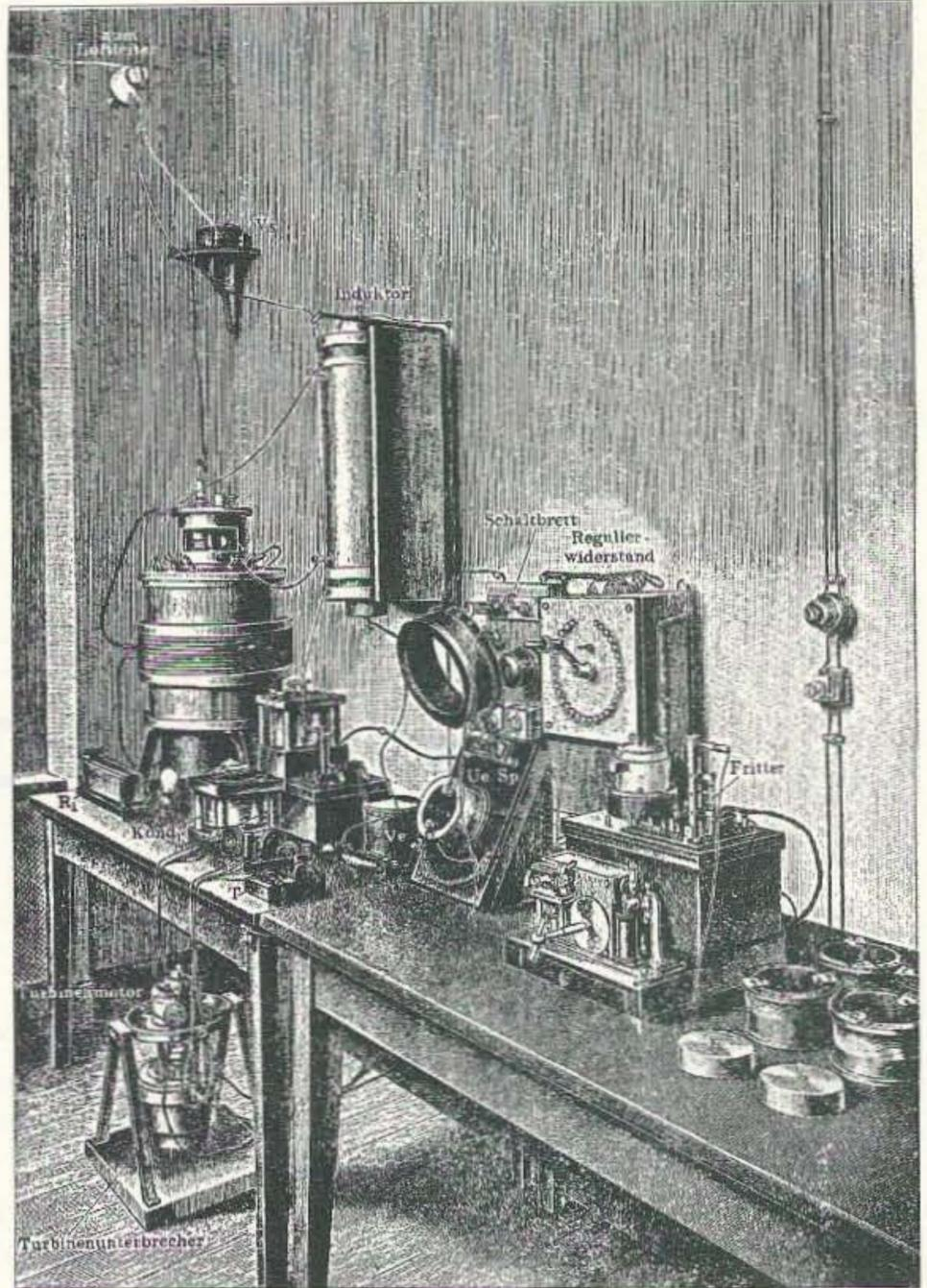
**Photo E.** The "ideal" amateur station in 1920, consisting of one transmitter and two receivers. One receiver uses an electrolytic detector and telephone set. The transmitter utilizes a mercury interrupter and an open core transformer.
