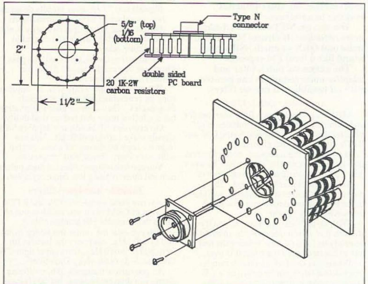
Figure 2. (b) Construction detail of the radial dummy.
