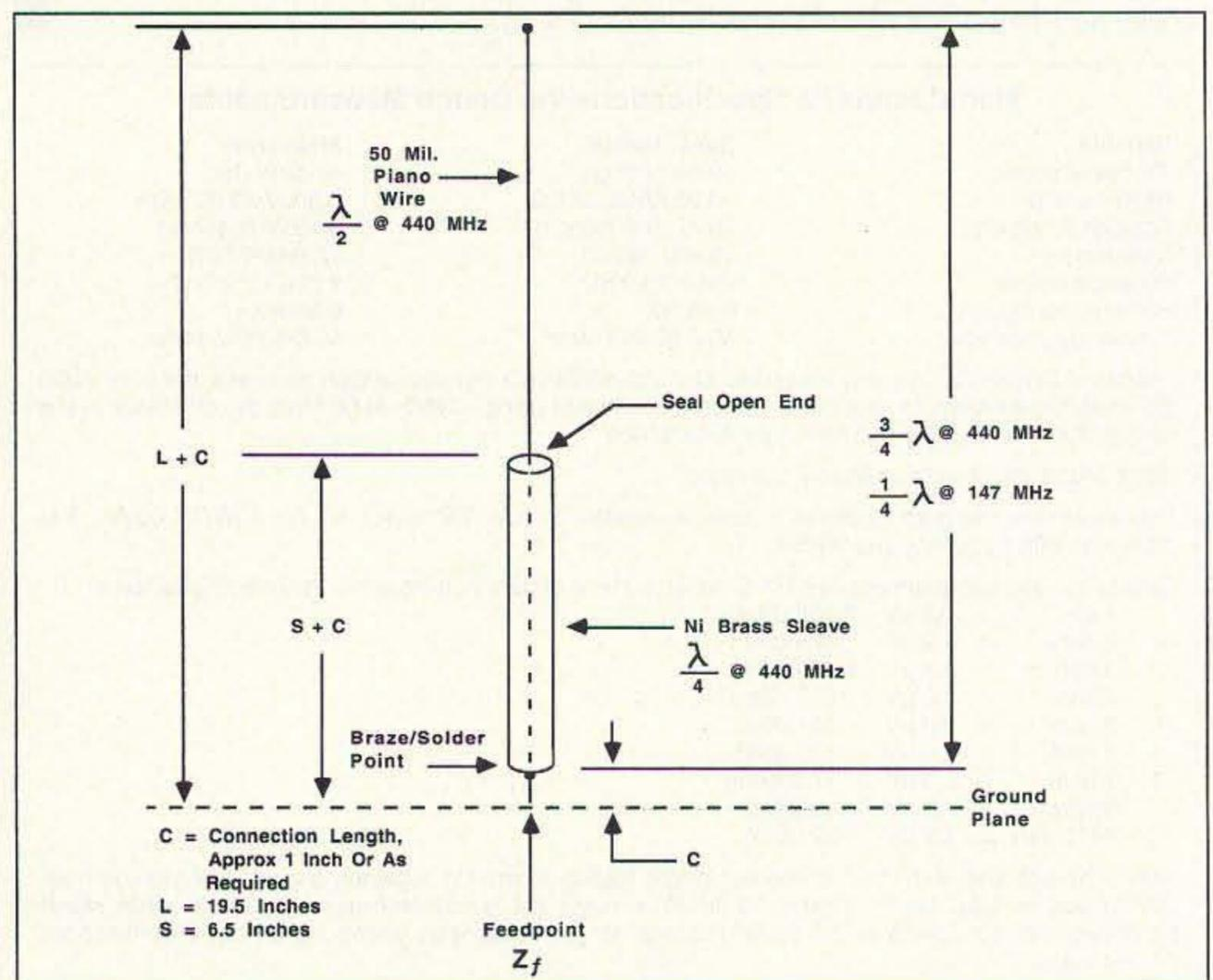
Figure 1. Detailed drawing of the dual-band antenna.
