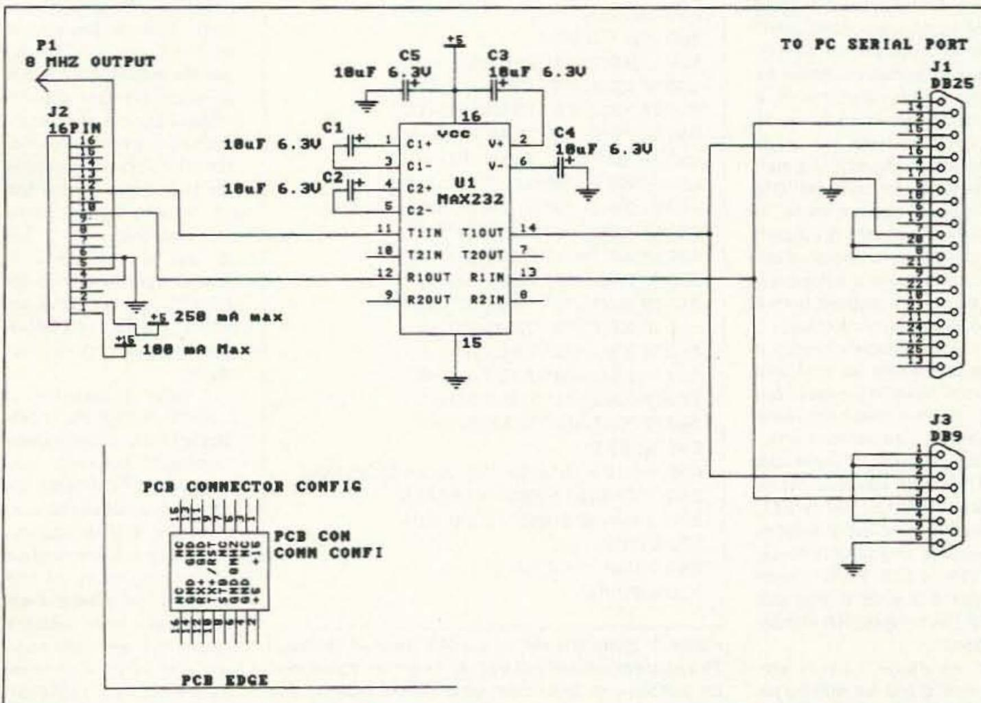
Figure 2. Schematic for Maxim-232 RS-232 PC-LORAN adaptor.
