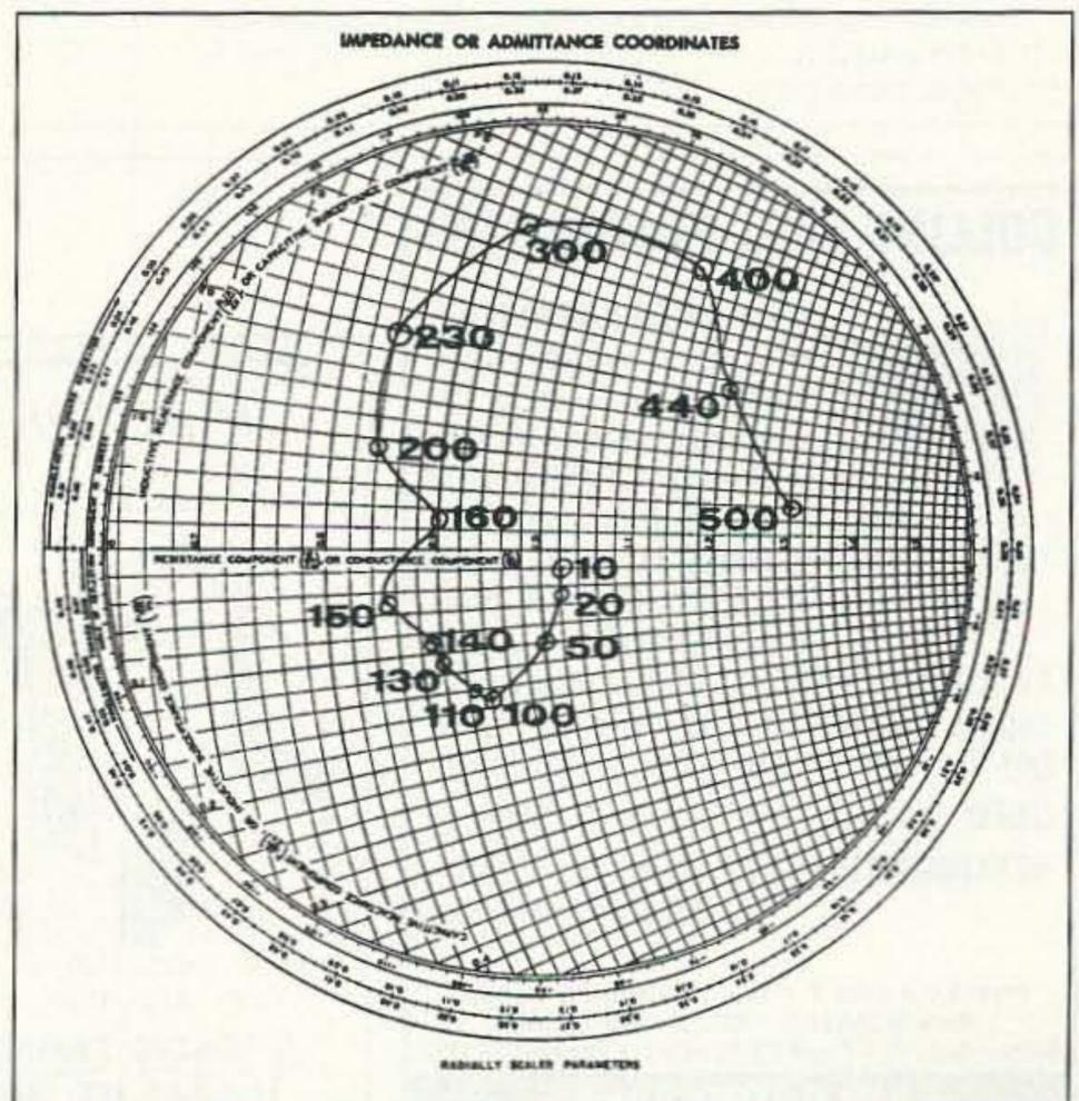
Figure 5. Radial dummy impedance from 10 to 500 MHz. The Smith chart is in expanded form.
