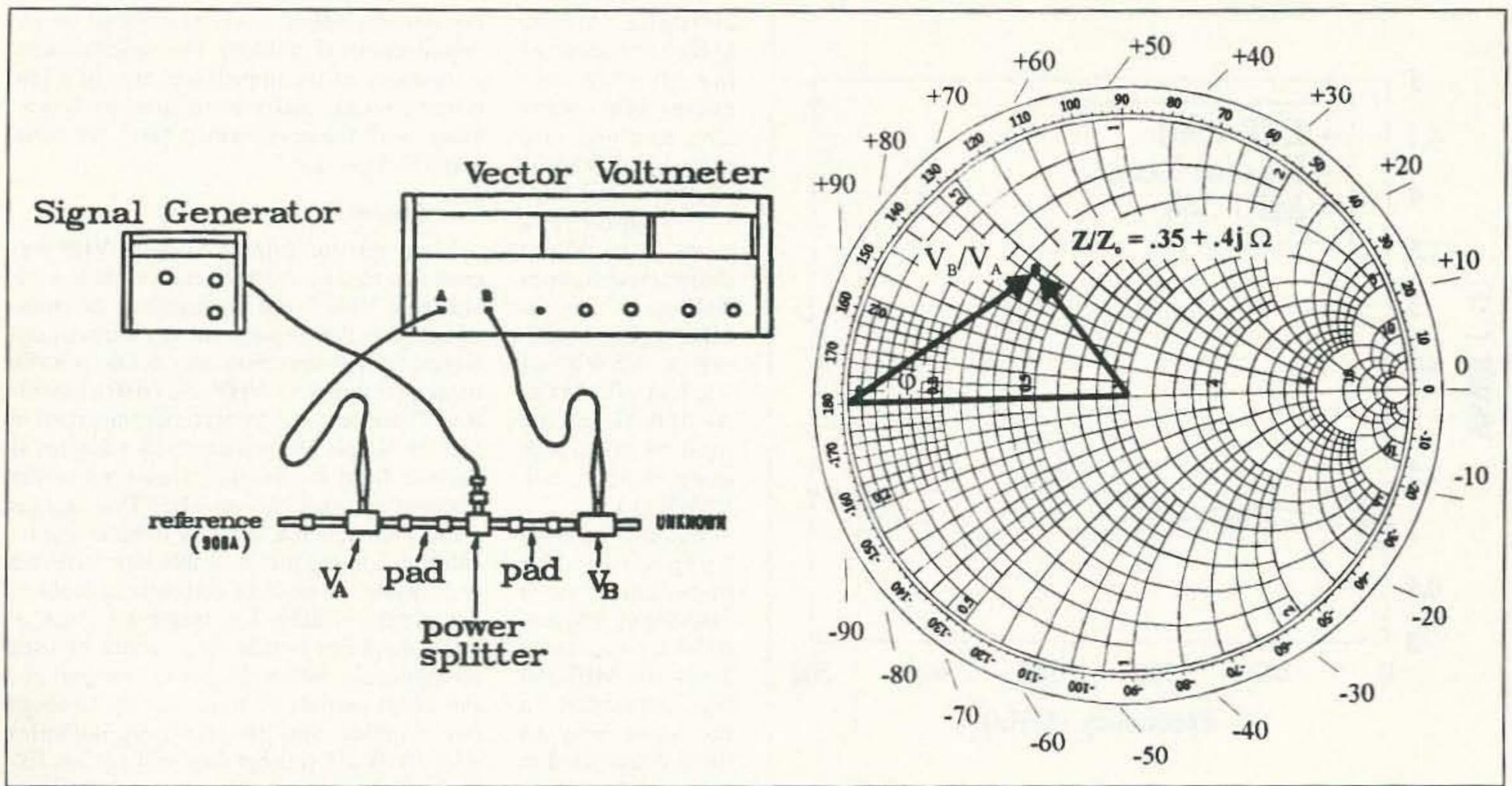
Figure 3. Complex impedance measurement using the Vector Voltmeter.
