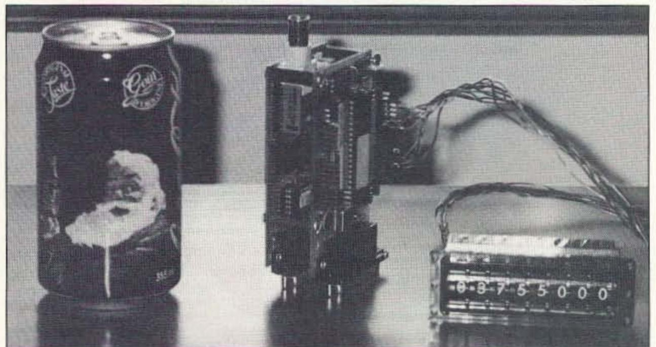
Photo B. Two boards make stand-alone DDS. (Photo by Sandy VE3AAC.)
