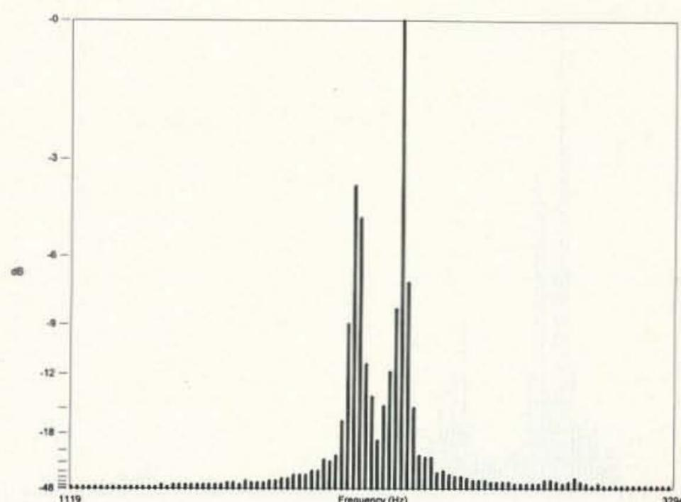
Figure 5. RTTY signal with 200 Hz spacing.
