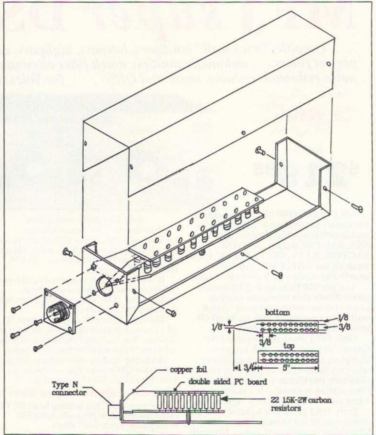
Figure 2 (a). Construction detail of the "DIP" dummy.
