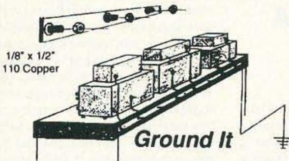
**Solid Copper Buss Stainless Steel Hardware Grounding Stud Every 6 Inches Top or Back Installation**
