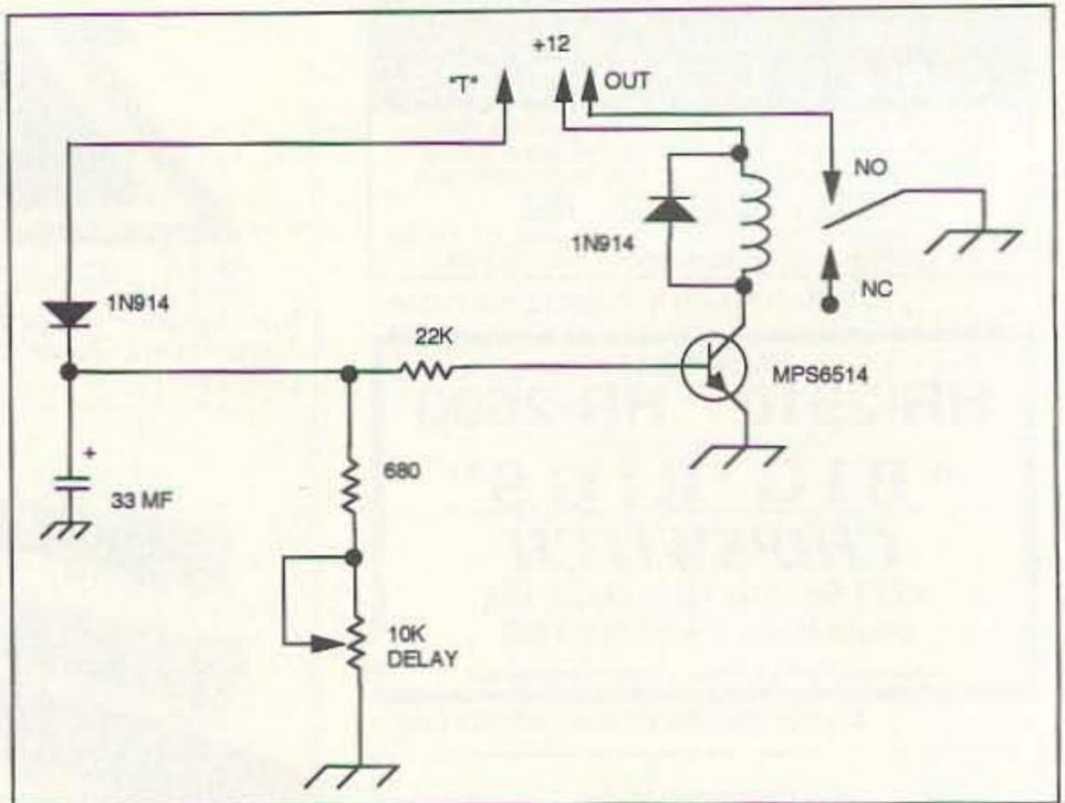
Figure 1. Amplifier T/R switching for the Argosy.
