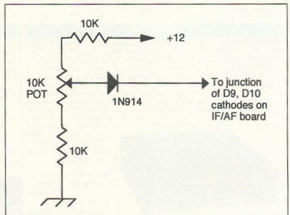
Figure 3. Improved RF gain control for the Argosy.
