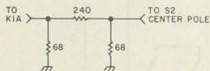
Fig. 2. 20-dB attenuator to enable 100-200-Watt transceiver to be used with QRP Amp . Resistors should be 20 Watts for 50-Watt output, 40-50 Watts for 100-Watt output, and 80-100 Watts for 200-Watt output. Use parallel combinations of smaller wattage resistors to reach these wattage ratings.
