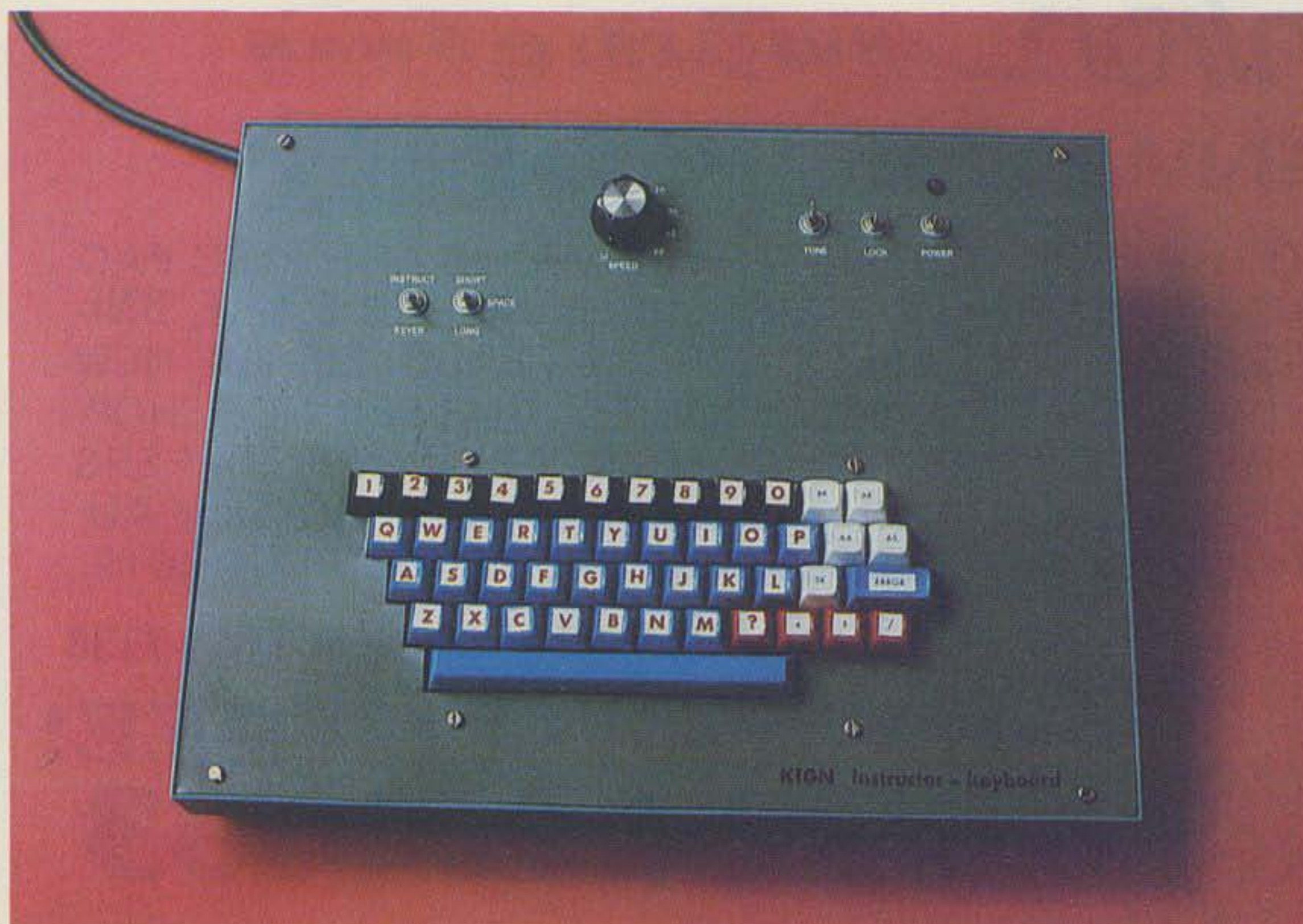
Photo A. The Instructor-KeyBoard is built in a homemade case. The front panel is made of galvanized sheet metal painted with spray enamel. The keyboard keys have been re-labeled with transfer letters. To the left are the Instruct/Keyer and Space switches; the speed control is in the upper center; to the right are the Tune, Sidetone on-off, and Power on-off switches.
