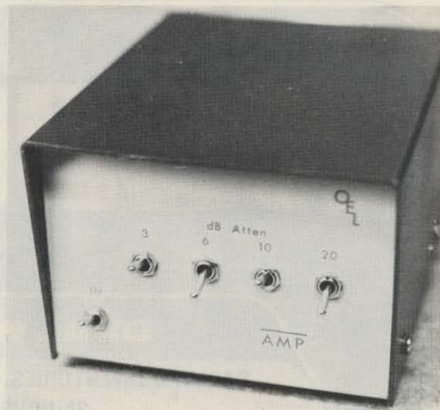
View of QRP Amp shown with 13 dB of attenuation and switched IN.
