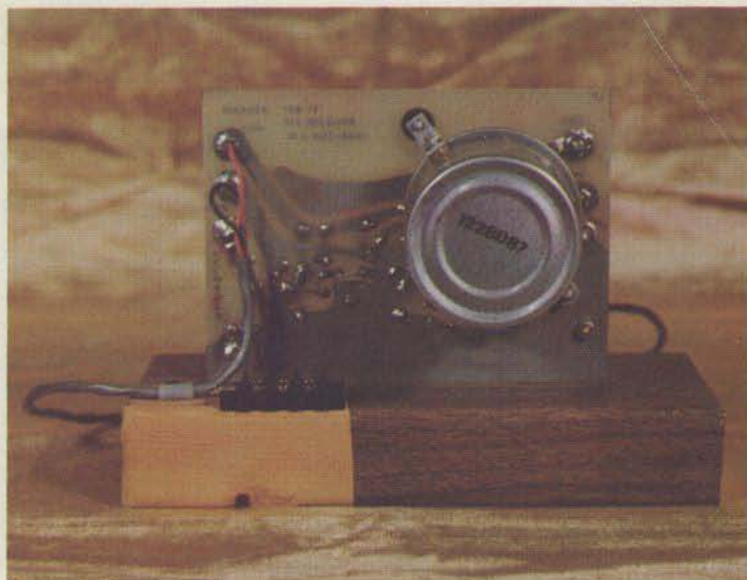
Photo C. Prototype receiver—rear view, showing the shielding method used.
