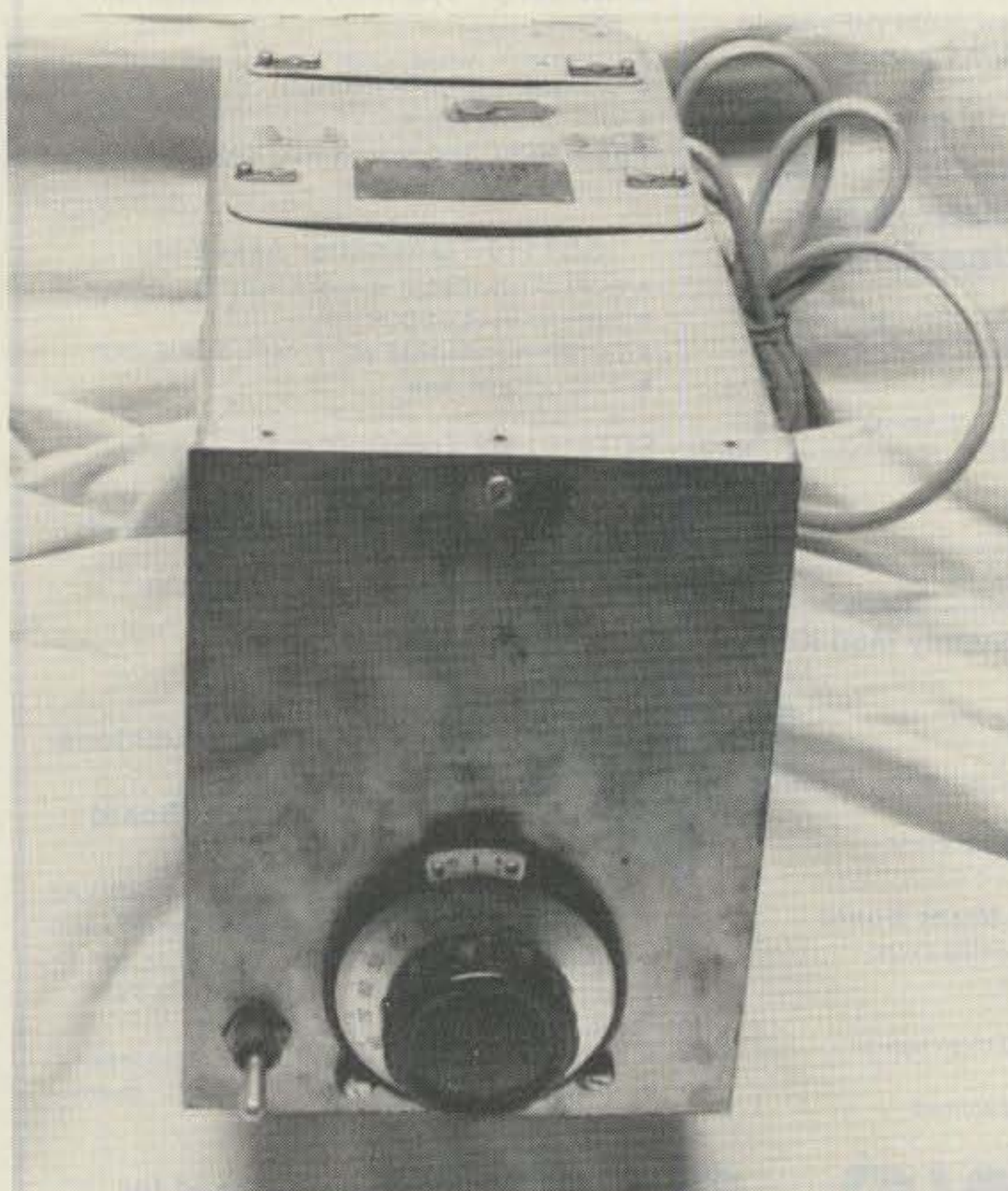
Photo A. Front view of the vfo showing use of the ARC-5 cabinet. The front is covered by a copperclad plate for appearance's sake and for dial mounting.
