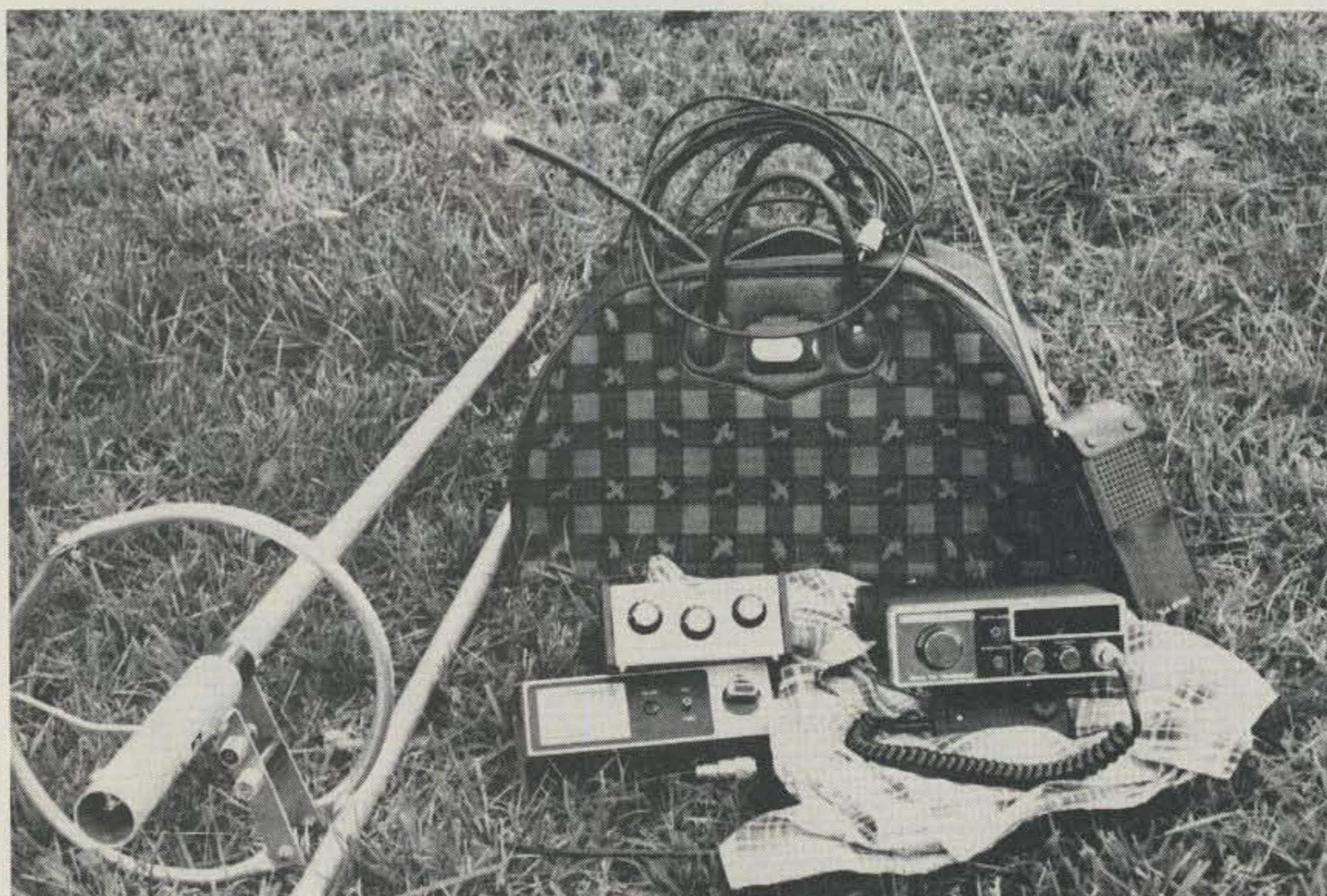
Photo A. Recipe for mountaintopping fun with 10 FM includes (left to right) a Cushcraft 10-meter FM Ringo, an MFJ antenna tuner with knapsack full of loose and long wires, Comtronix FM-80, and a 2-meter hand-held talkie.
