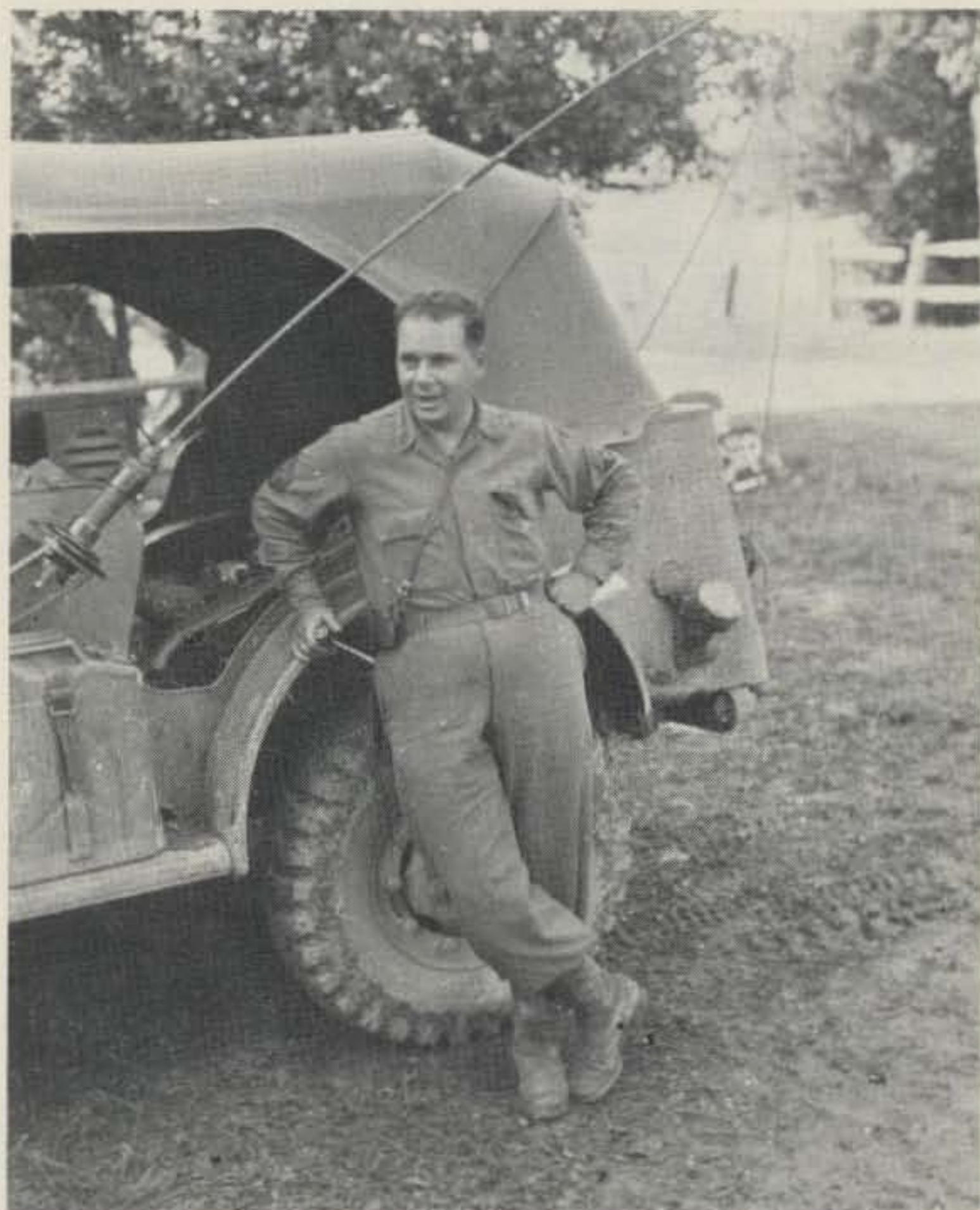
Photo E. The SCR-193 was mounted behind the front seat of this Command Car, and the whole rear compartment was the "radio shack." The rig got a good workout during maneuvers in the Carolinas during the summer of 1941.
