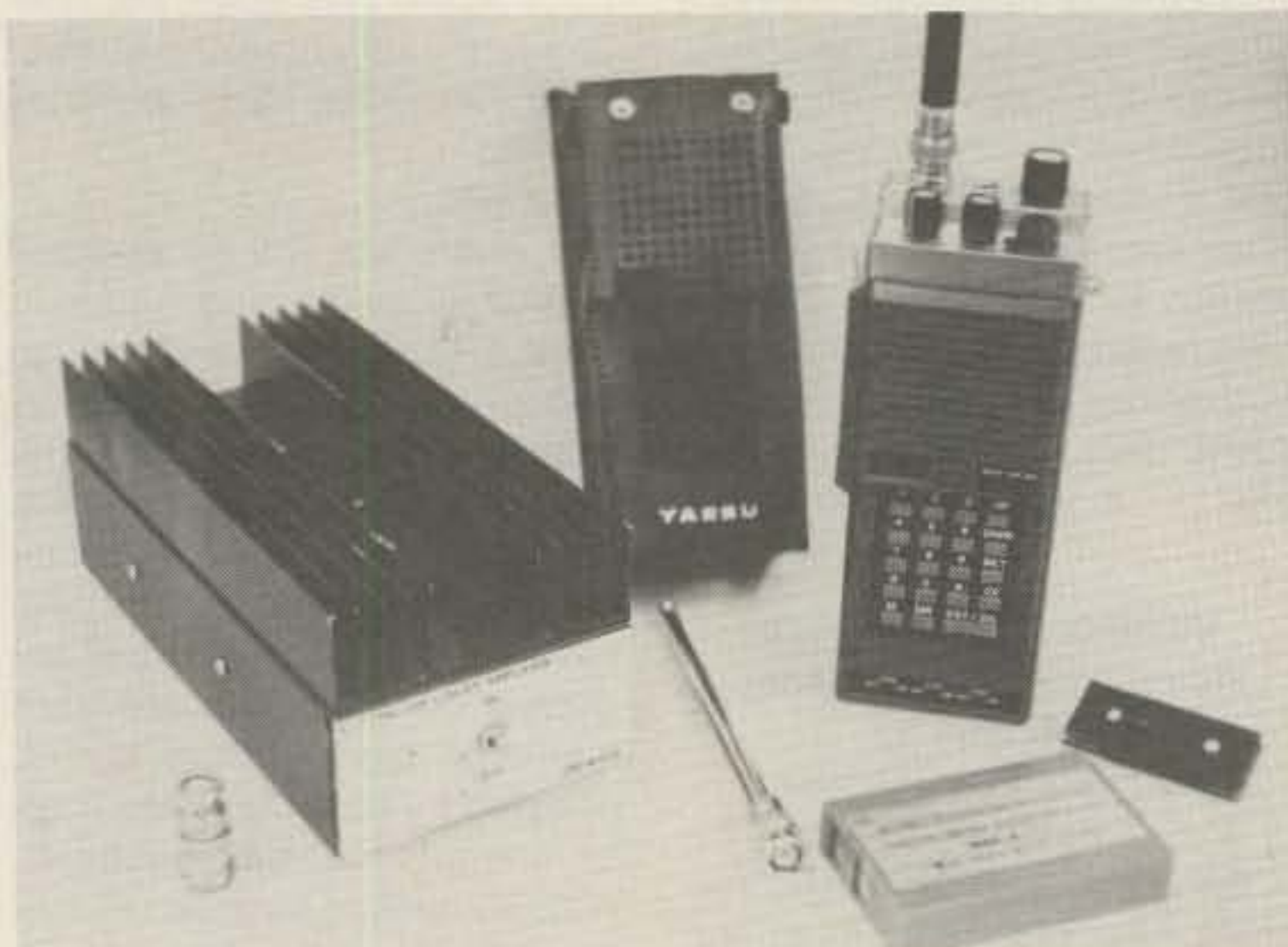
The Yaesu FT-207R and assorted items used by K4TWJ. Vinyl case was cut from FT-202R item. Klitzing amplifier boosts handie output to 50 Watts. Full-length pull-up antenna significantly extends handie's range. Adapter at left mates PL-259 to BNC. Battery tester described in text placed beside 207. Finally, 207's battery pack is in front of unit. A Yaesu speaker mike and length of coax with PL-259 and BNC were secured in the car and thus omitted from this photo.
