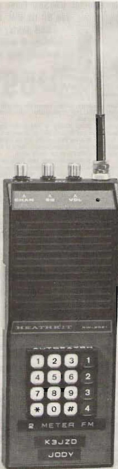
Photo A. Heathkit HW-2021 with the touchtone pad and 1/4-wave antenna installed.
