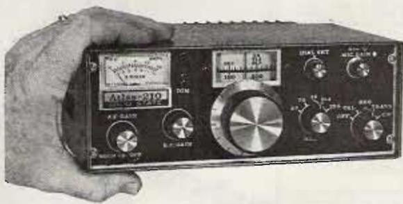
The Atlas 210x or 215x measures only 9 3/4" wide x 9 3/4" deep x only 3 1/4" high, yet the above photograph shows how easily the Atlas transceiver fits into a compact car. And there's plenty of room to spare for VHF gear and other accessory equipment. With the exclusive Atlas plug-in design, you can slip your Atlas in and out of your car in a matter of seconds. All connections are made automatically.
