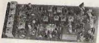
T50 Six Channel, 2W Exciter Kit for 2M, 6M, or 220 MHz ..... \$49.95
