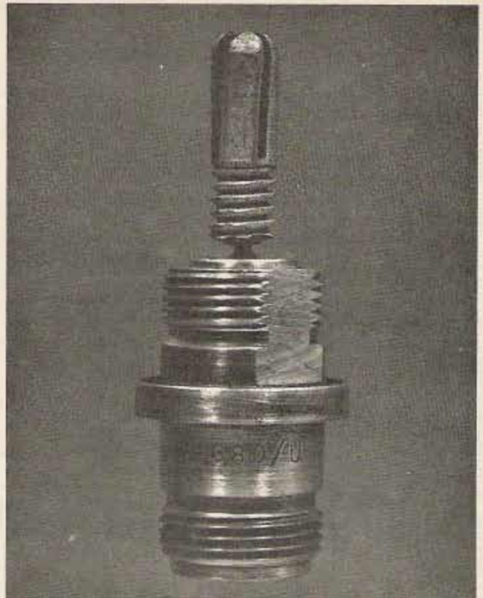
Close-up of "N" type connector with fabricated center pin. The threaded portion of the pin is immaterial.
