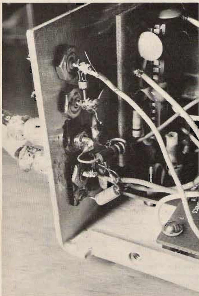
Inside view of connections showing the diode between +12 and PTT to absorb voltage glitches caused by rig's relay releasing and special resistor installed on output of receive frequency to pad it down a bit (3rd one down).
