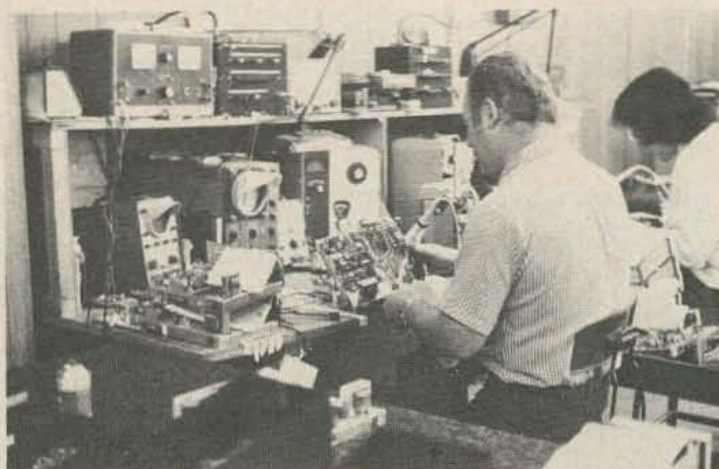
This is one of the test positions for servicing. One of the main problems with scanning receivers is the use of the wrong or bum crystals! At least that makes the sets easy to fix.
