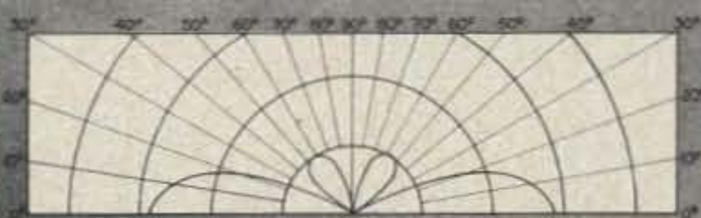
VERTICAL RADIATION PATTERN—G3-144
