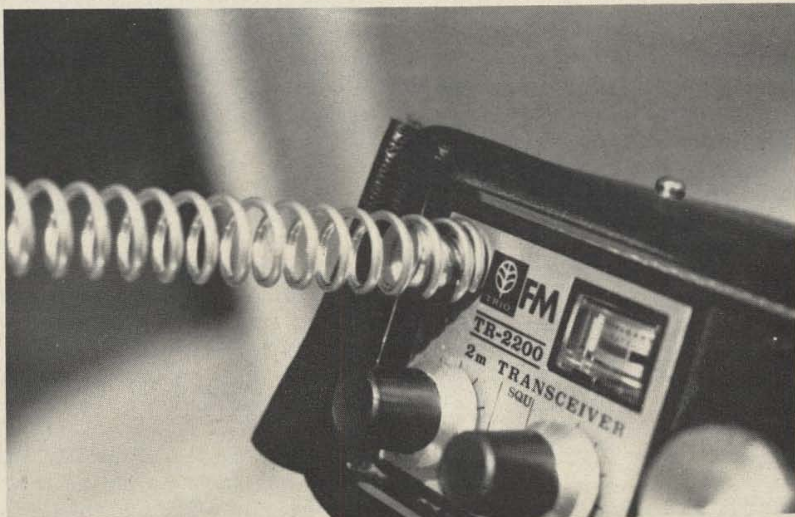
The spring fits snugly over the end of the standard TR-22 antenna. It can be removed in a second for use of the regular antenna.
