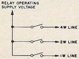
Fig. 5. The simplest way to feed a binary coded control signal into our control cable is to use separate switches and do the adding in our heads.
