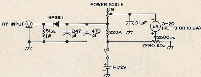
Fig. 1. Schematic diagram of 0.05–500 mW wattmeter.
