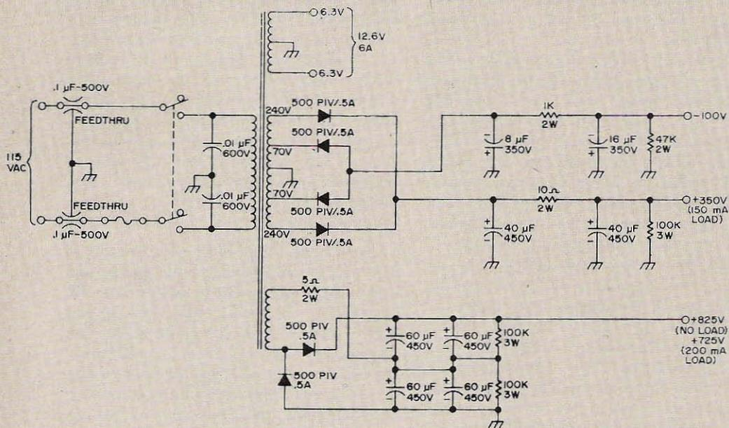
Fig. 1. Schematic of the suggested power supply.
