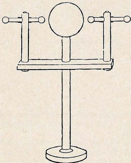
Fig. 1. Lodge's spherical antenna.
