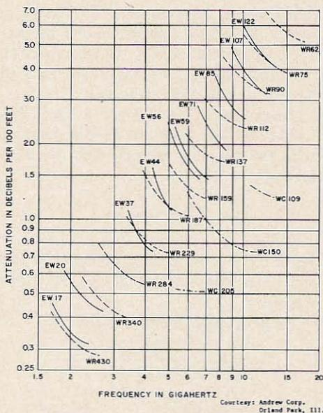
Fig. 10. Waveguide loss chart.
