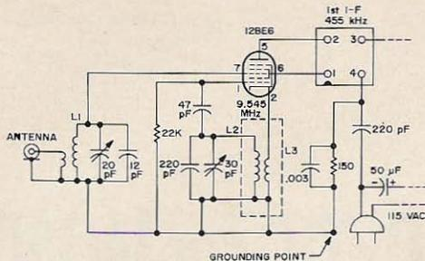
Fig. 2. Modified circuit of 12BE6 converter for WWV.
