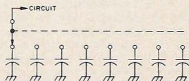
Fig. 2. Eight separate capacitors are needed to make up eight values of capacitance in this simple switching circuit.
