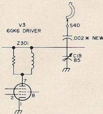
Fig. 2. This is the change incorporated by Swan on the later model 350s to prevent overheating of rf choke L306. (No connection between the junction of the capacitors and the driver plate circuit, please.)
