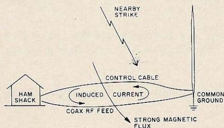
Fig. 8. Strong magnetic flux from a nearby earth strike can damage diodes by inducing large voltages if cables form a sizable open loop.
