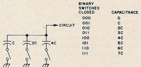
Fig. 4. Switching capacitors according to the pattern of the binary number system enables us to get eight values of capacitance from three capacitors.
