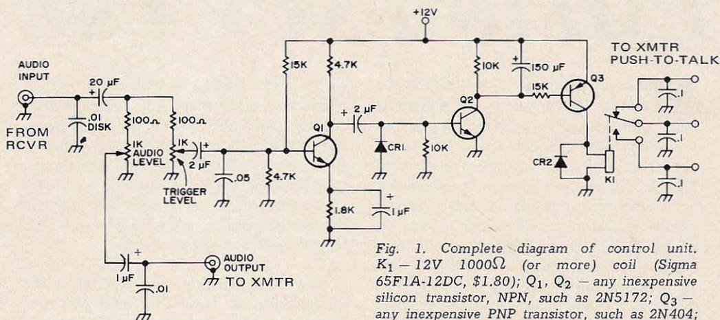
Fig. 1. Complete diagram of control unit.  $K_1$  — 12V 1000 $\Omega$  (or more) coil (Sigma 65F1A-12DC, \$1.80);  $Q_1, Q_2$  — any inexpensive silicon transistor, NPN, such as 2N5172;  $Q_3$  — any inexpensive PNP transistor, such as 2N404; capacitors — all ceramic or electrolytic (15V rating or higher); resistors —  $\frac{1}{4}W$  or  $\frac{1}{2}W$ ;  $CR_1, CR_2$  — any small germanium or silicon diode.
