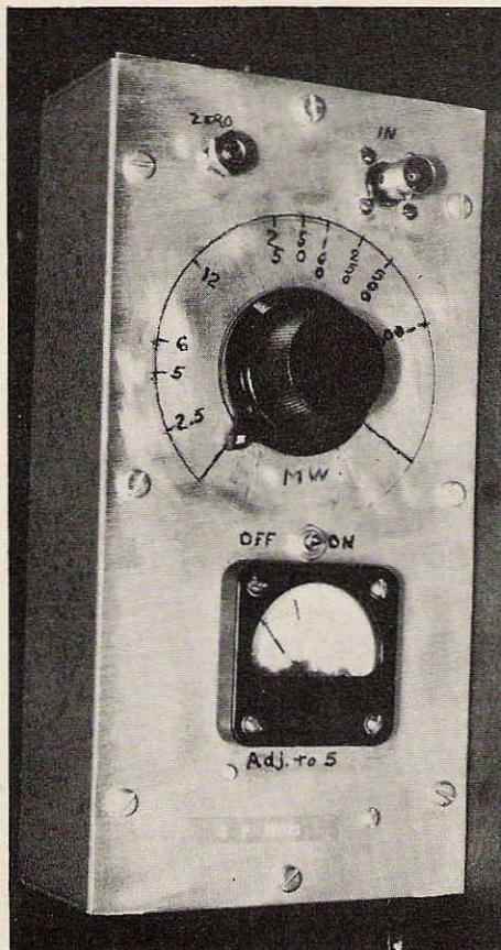
1 to 1000 milliwattmeter top view, 4 x 8 x 2 inch case.
