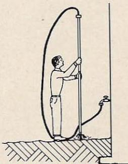
Fig. 2. Insertion of the ground rod. The flowing water will "erode" a hole out ahead of the pipe. The pipe should be started far enough from the wall to miss the concrete footings if they are present. Stop dropping the pipe (and shut off the water) before the top of the pipe is even with the ground to ease removal of the coupling and soldering of the bus. After the bus has been installed, stepping on the pipe will force it down to ground level.
