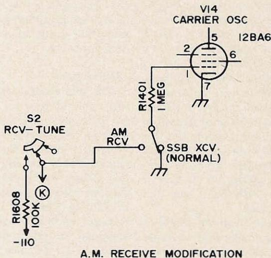
Fig. 1. This diagram shows the changes made in order to copy AM without a beat note caused by drifting of the signal. The switch is mounted on the front panel below the S-meter to the left of the PTT/VOX switch.
