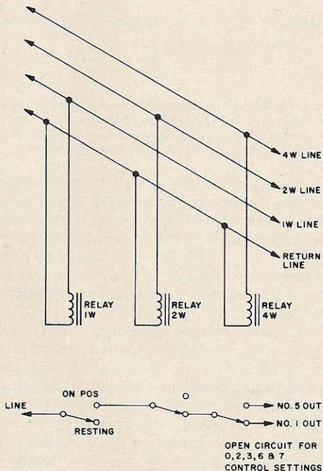
Fig. 10. Here is one station of an elaborate remote switching system. It completes a circuit when the control setting is either 1 or 5. Use this for reference in working out arrangements to function at other control settings.
