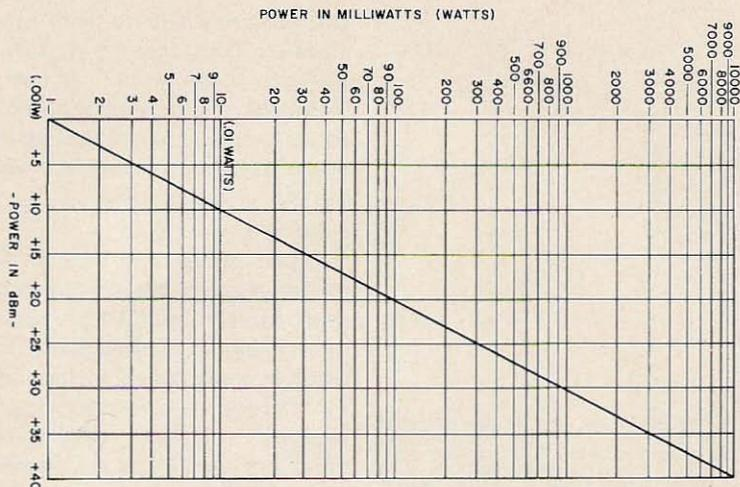
Fig. 6. Transmitter output/dB conversion chart.
