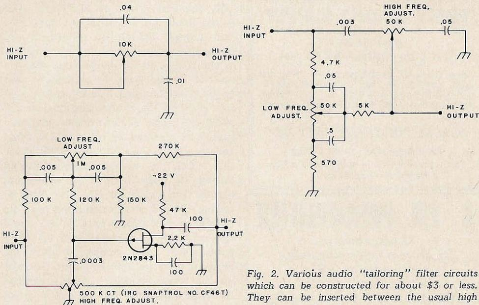
Fig. 2. Various audio "tailoring" filter circuits which can be constructed for about \$3 or less. They can be inserted between the usual high impedance microphone and a transmitter or between the output of a compressor and the audio input of a transmitter.
