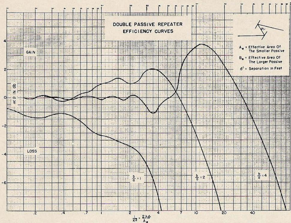
Fig. 1. Double passive efficiency.
