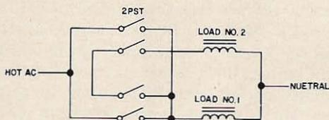
Fig. 1. Schematic for a two load fail safe arrangement.
