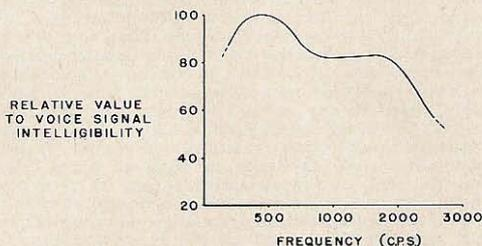
Fig. 1. As shown in this graph, all frequencies in the 300–3000 CPS range do not contribute equally to voice signal intelligibility. A completely "flat" audio response in a transmitter does not, therefore, provide the best voice signal effectiveness.
