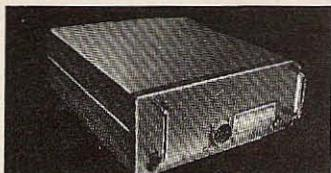
R.C.A. CMC60 B 6/12 volt, 60 watts, 150-170 MHz receiver has vibrator, transmitter, dynamotor power supply, with accessories. .... **\$68.**
