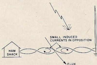
Fig. 9. Induced power is made small and averages to near zero if we twist the cables around each other a few times. Not recommend for twin-lead carrying rf.
