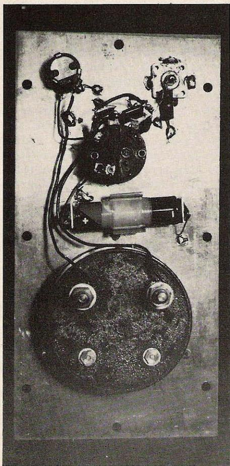
.05 to 500 milliwattmeter, underside view of completed 4 x 8 board mounting.
