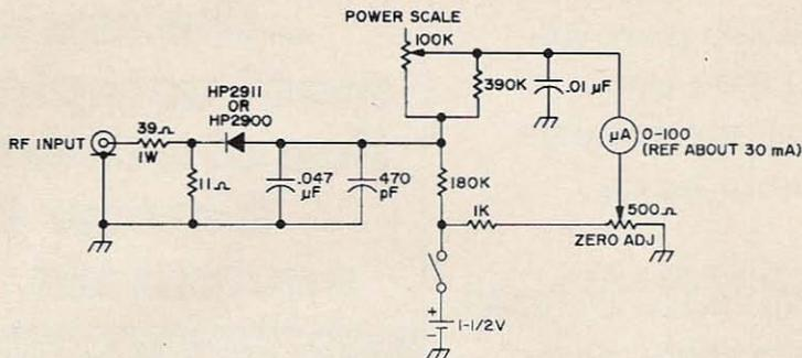
Fig. 2. Schematic of milliwattmeter for measuring rf power levels of 1–1000 mW.
