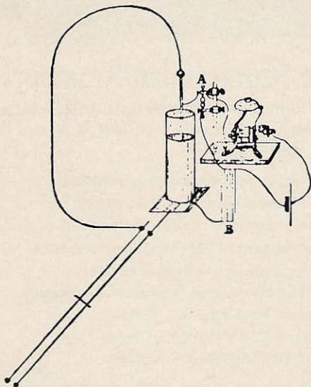
Fig. 4. Lodge's tuned lines and receiving gear.
