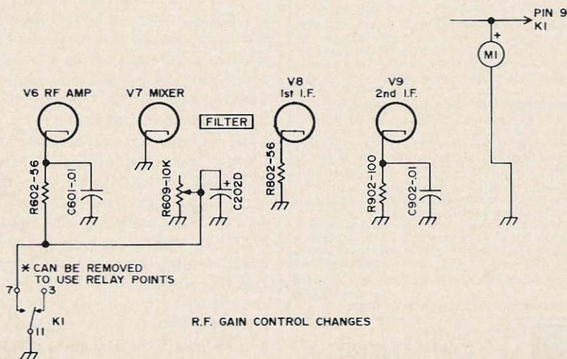
Fig. 4. This eliminates frequent rf gain control scratchiness and gives apparent sensitivity increase.
