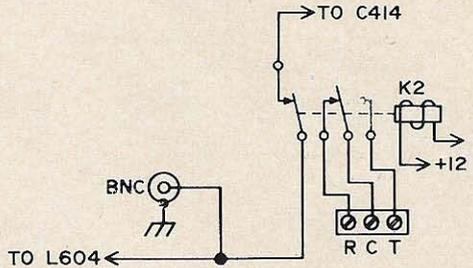
Fig. 3. The BNC connector is mounted on the rear apron between the power connector and accessory socket. This allows injection of signals from VHF converters, frequency calibrators, etc., without the possibility of damage due to accidental tripping of the transmit switch.
