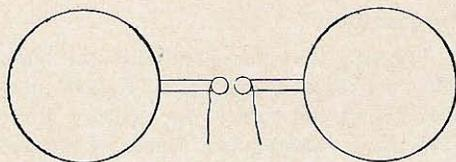
Fig. 3. Standard Hertz radiator producing the wave of Fig. 2.
