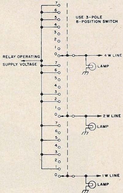
Fig. 6. We will probably need a three wafer rotary switch for this circuit, which will code the correct voltages into the control cable for each setting. Pilot lamps offer binary readout of the signal applied to the system.
