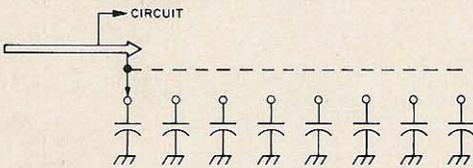
Fig. 3. If we use a continuous shorting switch, we still need eight capacitors, and the switch will cost more than an ordinary selector switch.
