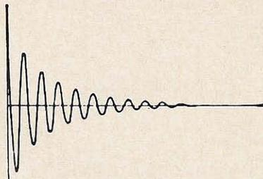
Fig. 2. Highly damped wave.
