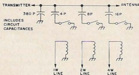
Fig. 12. Remotely located at the base of an antenna tower, this system will switch in parallel capacitances for tuning the antenna to any of eight frequencies over a narrow band.
