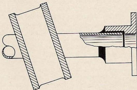
Fig. 1. Female hose connector is sweat-soldered to rigid copper ground pipe. Solder is shown in solid black. Use a blowtorch and plenty of heat. If the hose coupling is forgotten, it can be easily slipped over the plain end of the pipe after the soldering is finished. Soldering in a pipe to pipe coupling for a longer ground rod is similar although less convenient because the pipe will be vertical. Have a friend hold the upper pipe.
