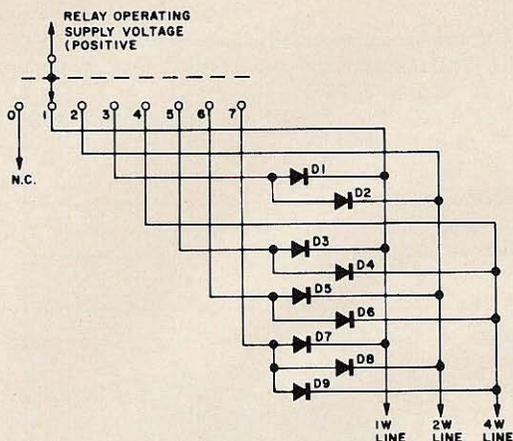
Fig. 7. A more complex circuit enables us to use a simpler switch. This is the way to do it for large systems.
