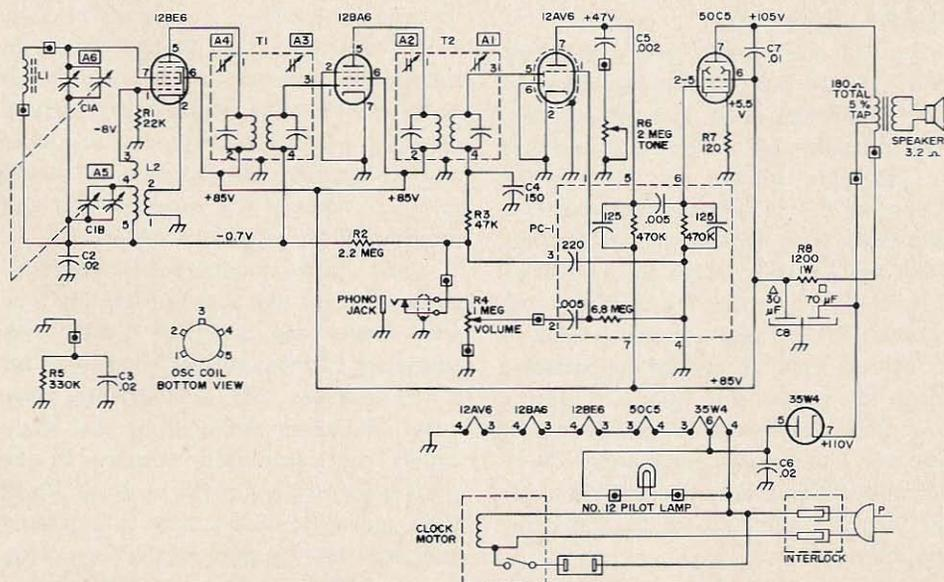
Fig. 1. Unmodified circuit of a typical ac/dc broadcast band receiver.
