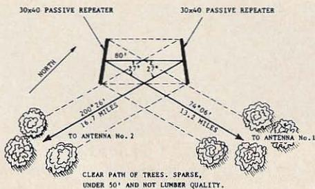
Fig. 12. Double passive repeater with horizontal included angle of  $27^\circ$ . Typical layout.
