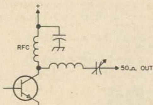
Fig. 1. Alternate output circuit to provide 50 ohm output for the 2N2950.
