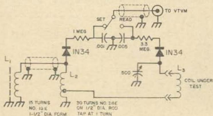
Fig. 1. Schematic of Q-meter.
