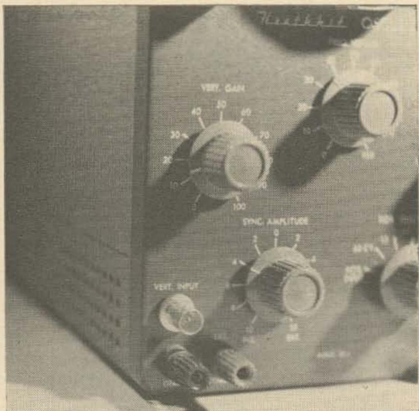
Shielded leads should always be used with an oscilloscope when you're checking high-impedance circuits, since the unshielded variety can easily pick up 60-cycle ac fields which exist in every building wired for power. Yet most inexpensive scopes have no convenient method for attaching shielded leads and maintaining the shielding intact all the way up to the scope itself.
