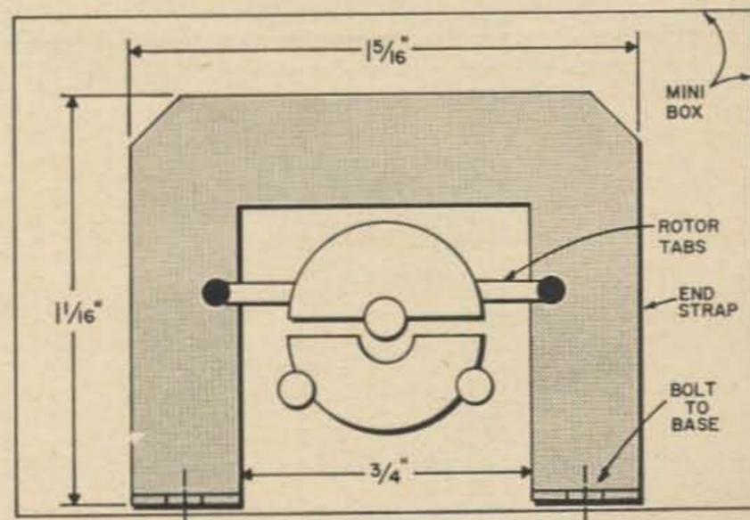
Fig. 5. Details of the top ground strap and the capacitor grounding strap.
