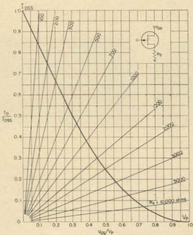
Fig. 6. Normalized FET transfer curve.
