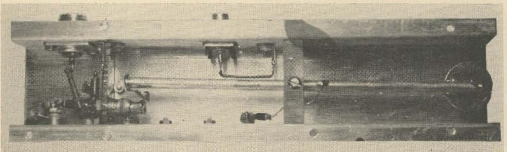
Inside of the 8058 Nuvistor preamp. C3, the plate tuning capacitor, is at extreme right. L1, the plate line, runs from the tube to C3. RFC2, the plate feed choke is near the center support and the output link L2 is just above it.
