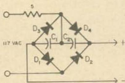
Fig. 1. "Full Wave Tripler." It doesn't work.
