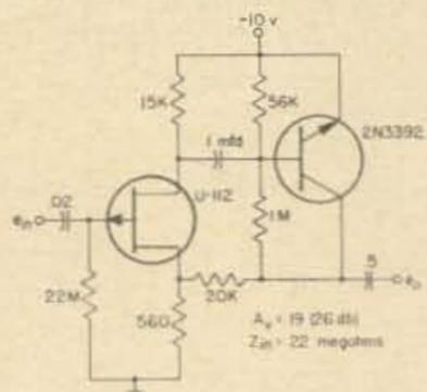
Fig. 13. High impedance preamplifier.
