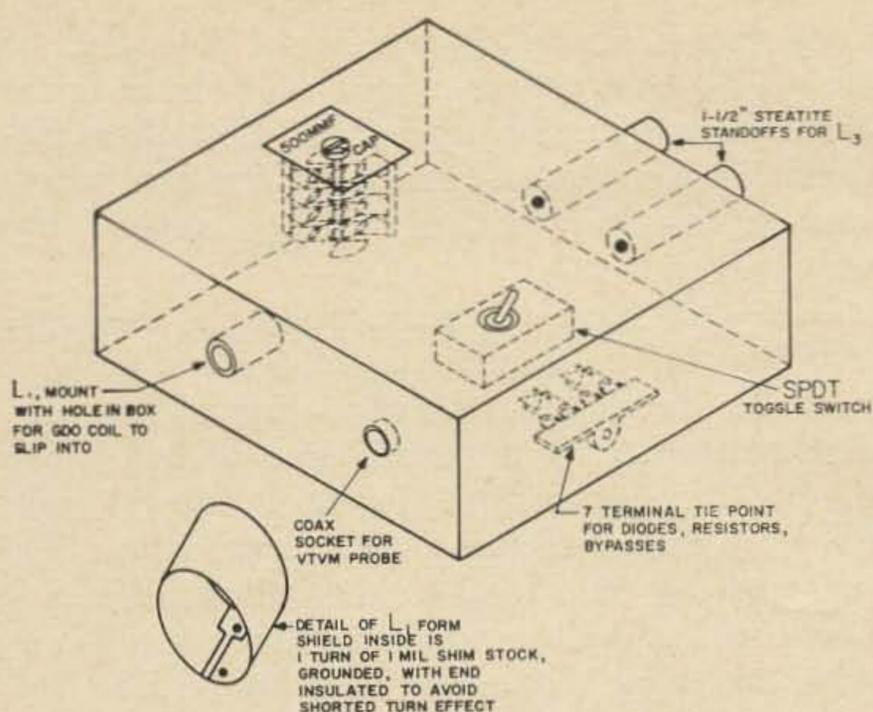
Fig. 2. Suggested layout of Q-meter.
