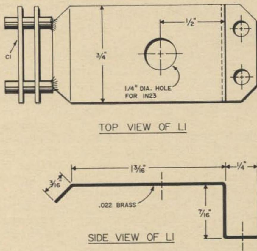
Fig. 4. Details of L1. See Fig. 3 for location.
