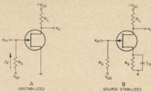
Fig. 9. Biasing FET amplifier stages.
