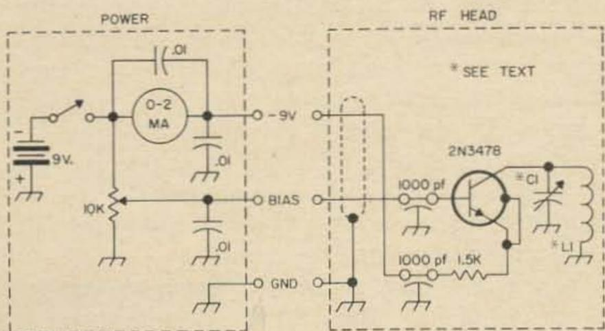
Fig. 2. Final circuit of the dip meter.
