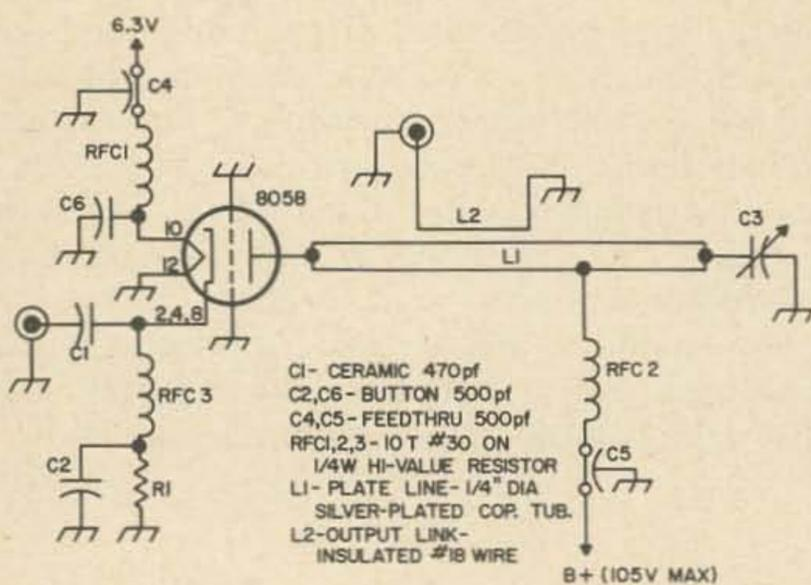
Fig. 1. Schematic of the 8058 preamp for 432 mc.
