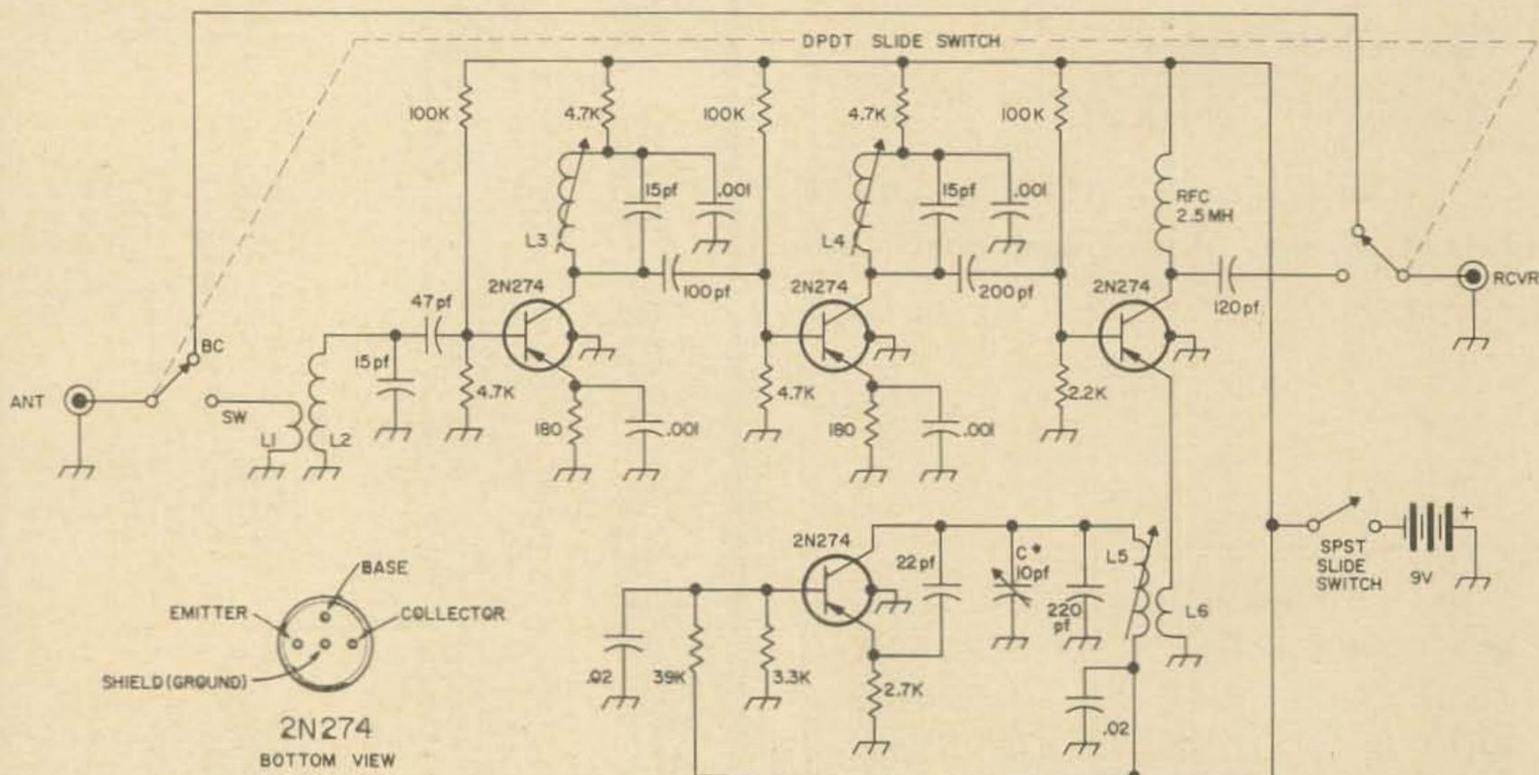
Fig. 1. The transistorized tunable twenty meter converter.
