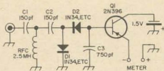
Fig. 1. The WIJL Transistorized Field Strength Meter. A printed circuit board is available for 50¢ and a wired board for \$2.50 from the Harris Company, 56 E. Main, Torrington, Conn.
