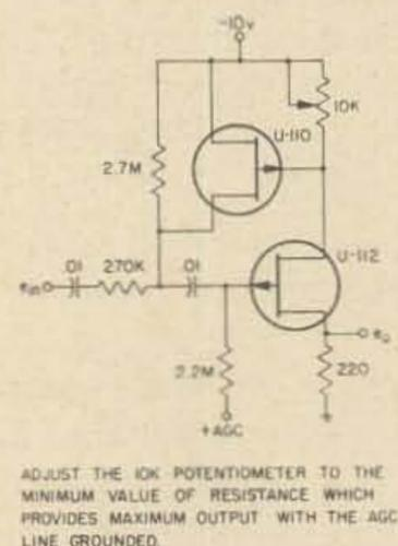
Fig. 11. Automatic gain control circuit.
