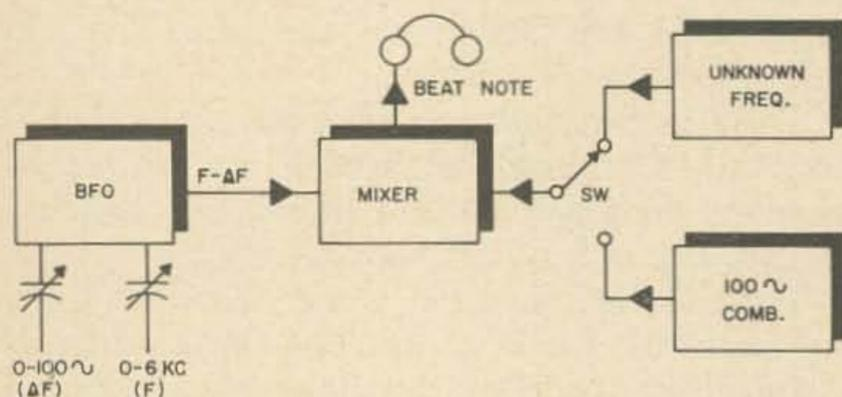
Fig. 1. Block diagram of the Audio Frequency Standard.
