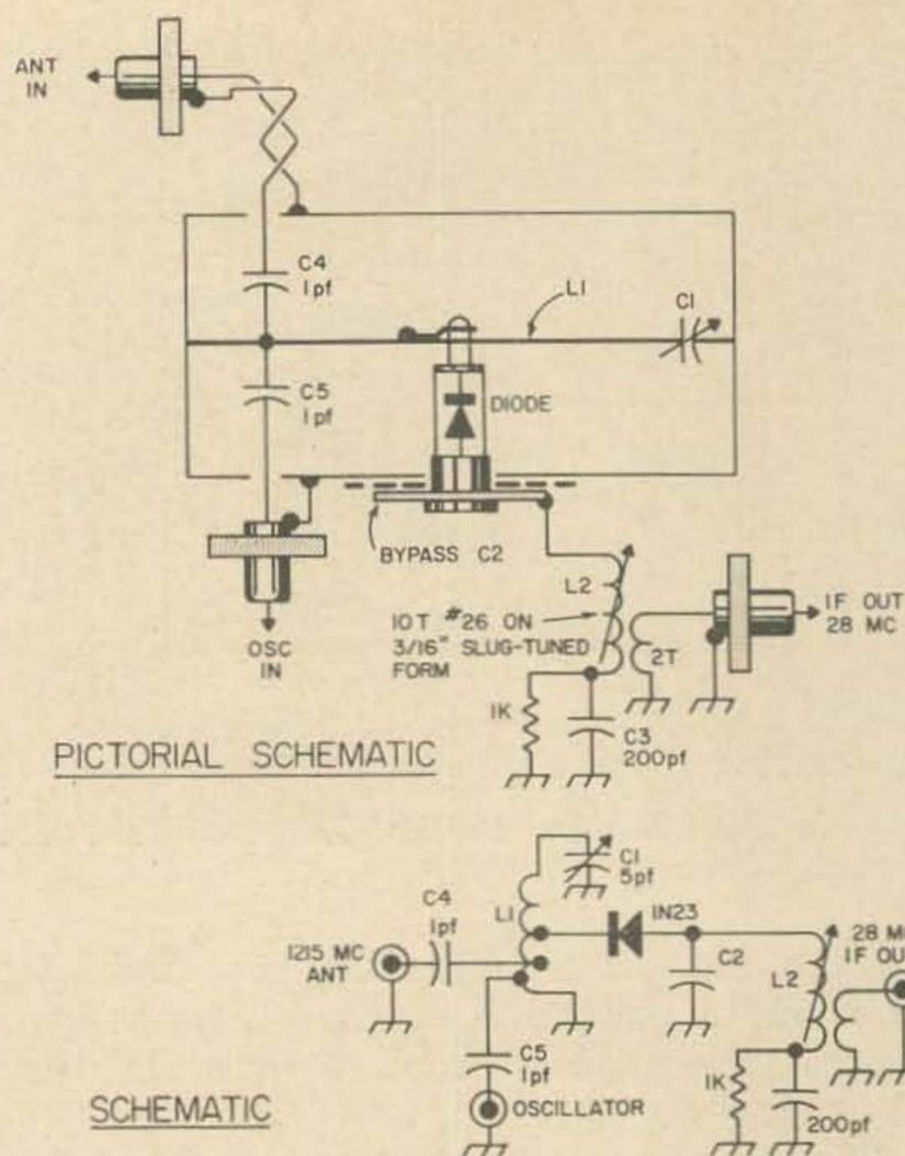
Fig. 7. Pictorial schematic and schematic of the 1250 mc mixer.
