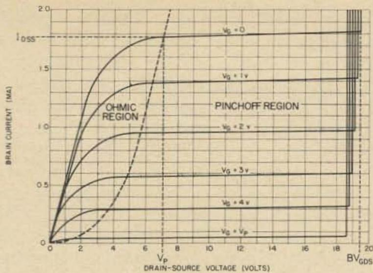
Fig. 3. FET drain characteristics.
