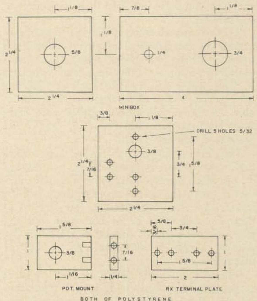
Fig. 5. Box drilling details.
