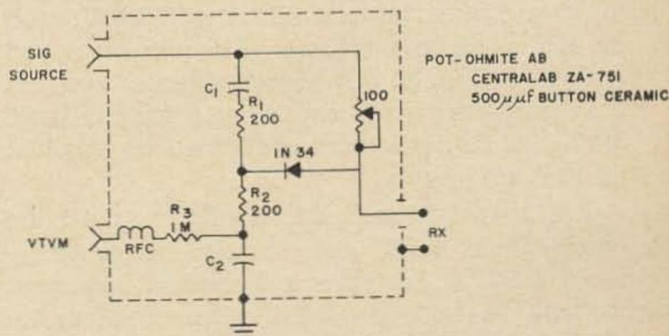
Fig. 3. Schematic of Impedance Bridge.
