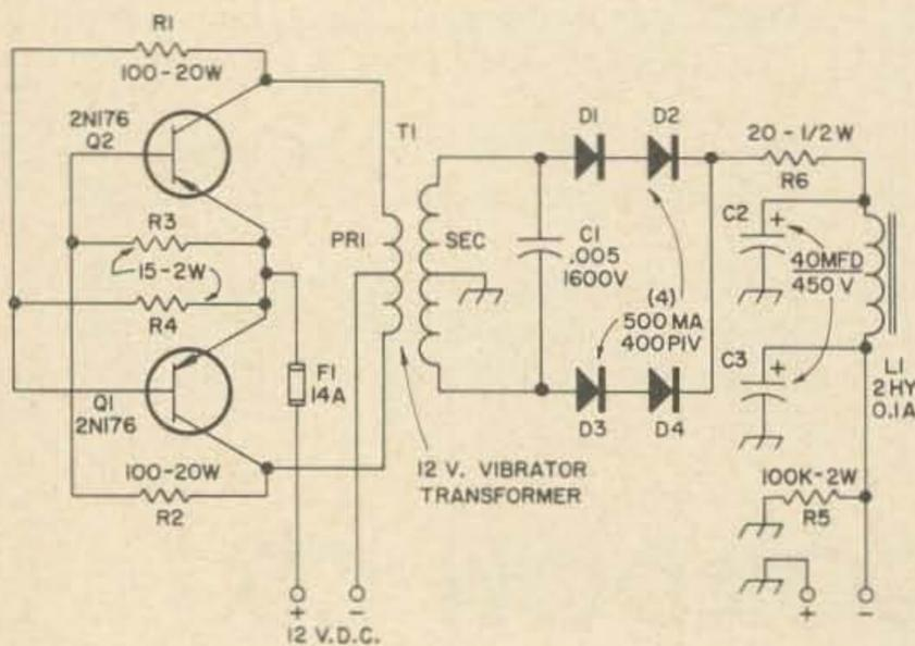
Fig. 1. Schematic of the Pauper's Portable Power Pack.
