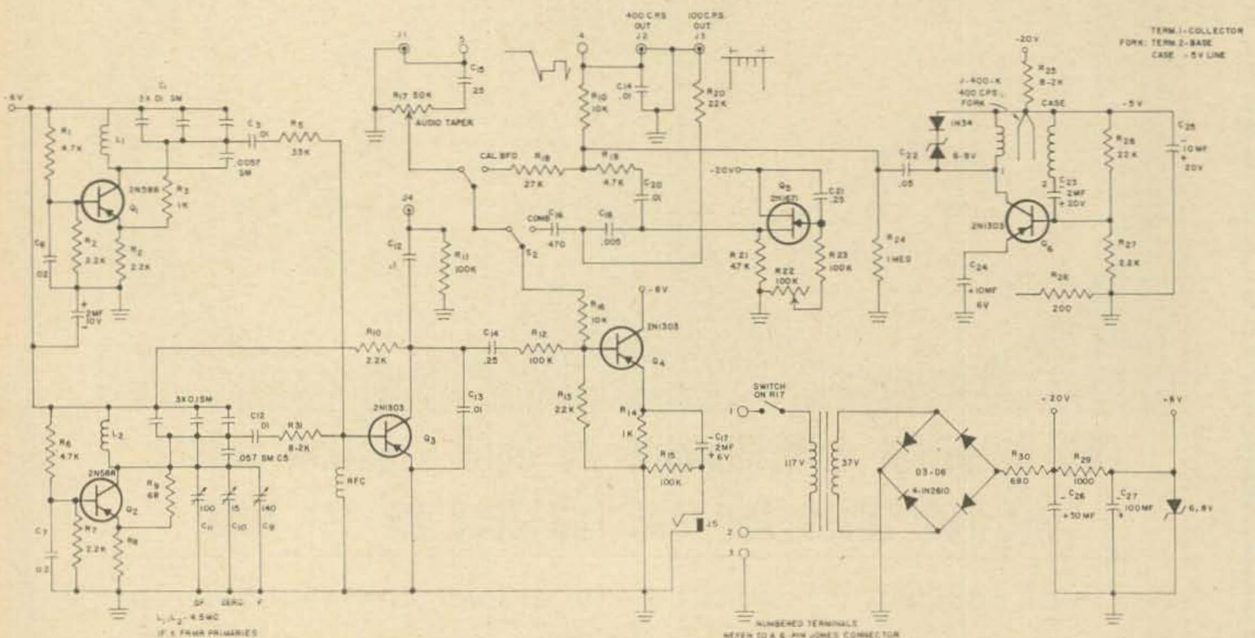
Fig. 3. Schematic of the 100-6000 cycle Audio Frequency Standard.  $L_1$ ,  $L_2$  are 4.5  $\mu$  transformer primaries. Remove internal capacitors. T1 is a miniature 37 v transformer (available from author for \$1.) The fork is a Philamon J-400-K.  $C_5$  should be .0057 and the three .1's above it .01's.
