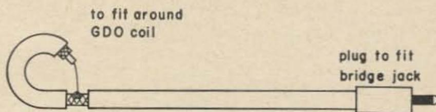
Fig. 6. GDO coupling cable.
