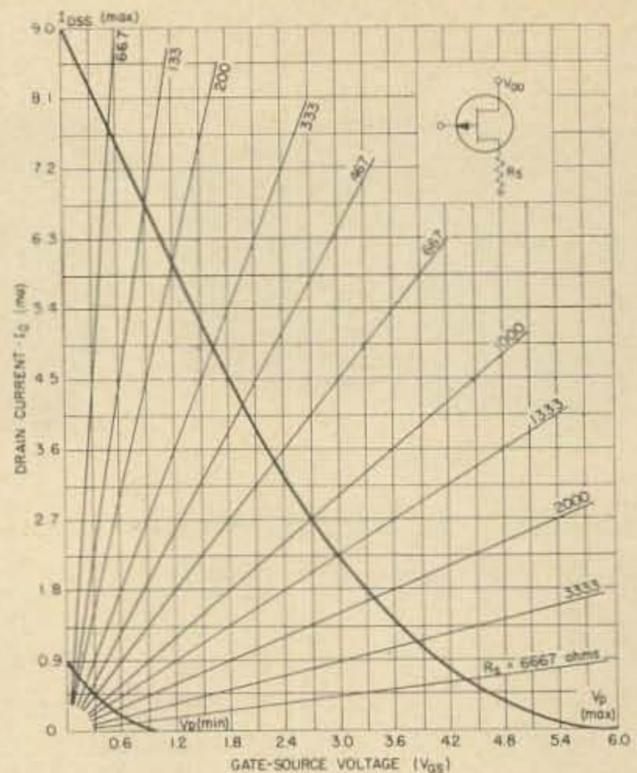
Fig. 7. U-112 transfer characteristics.
