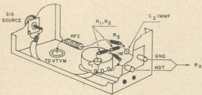
Fig. 4. Cutaway showing parts location.
