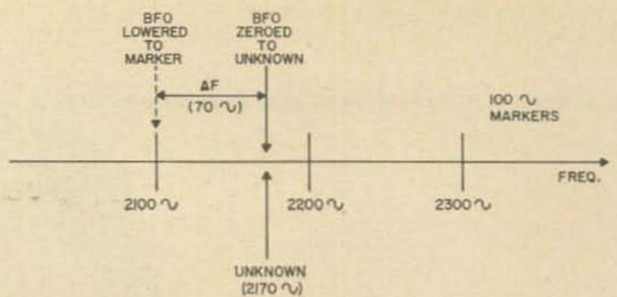
Fig. 2. Frequency relationships in measuring an unknown.
