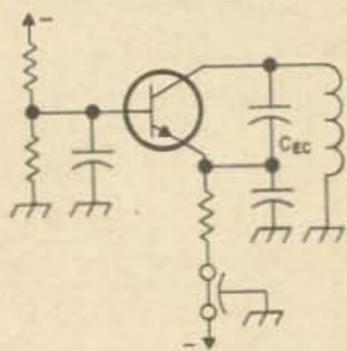
Fig. 1. Basic grounded emitter Colpitts oscillator.
