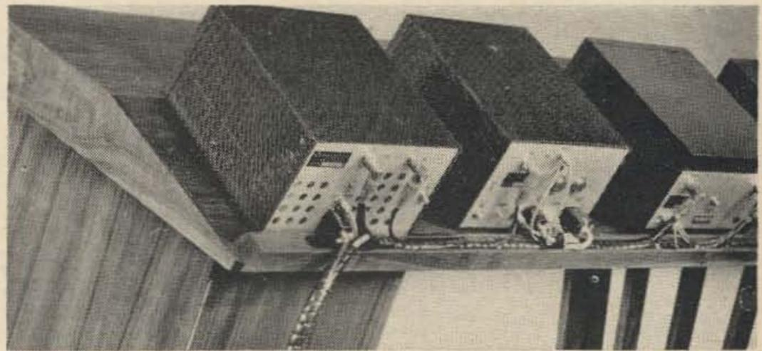
Functional trough keeps cable neat, allows easy access to connections. Equipment mounts safely on tilted surface at just the right operating angle.
