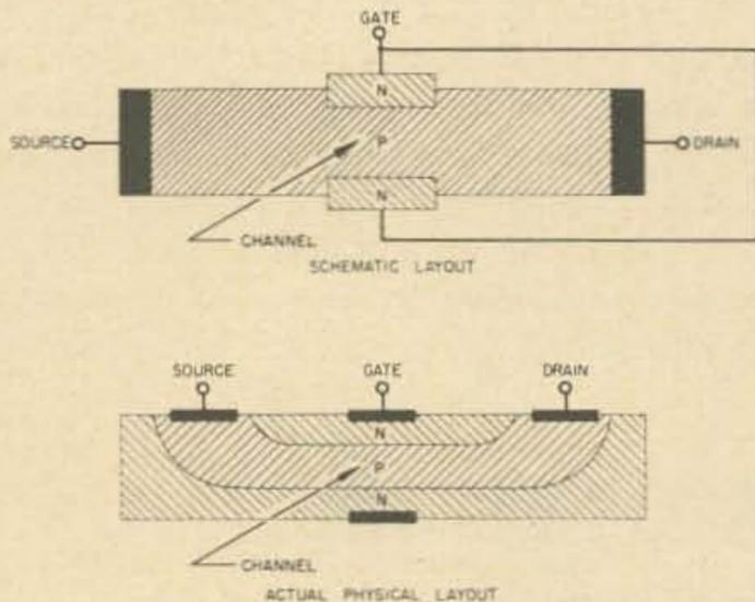
Fig. 1. The Field effect transistor.
