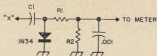
Fig. 2. Typical metering circuit. One needed for each stage.
