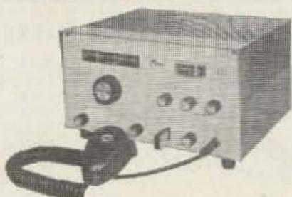
RECEIVER: Special triple conversion design, Selectivity about 10 KC at 6db and less than 16 KC at 50 db, Tuning dial calibrated 144 to 148 MC, Adjustable Squelch. TRANSMITTER: Push to Talk, Straight through final amplifier with xtal controlled 18 Watt input, self-contained Supply for AC & 12 Volts D C.
