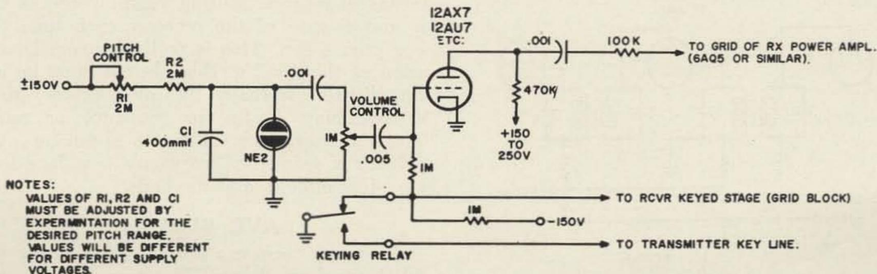
FIG. 2 SIMPLE KEYED SIDETONE GENERATOR.
