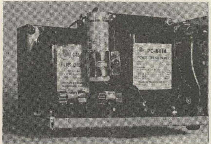
Internal view. The two silicon rectifiers conceal two identical rectifiers, one behind each of the two shown. The second filter condenser is located directly behind the one shown.
