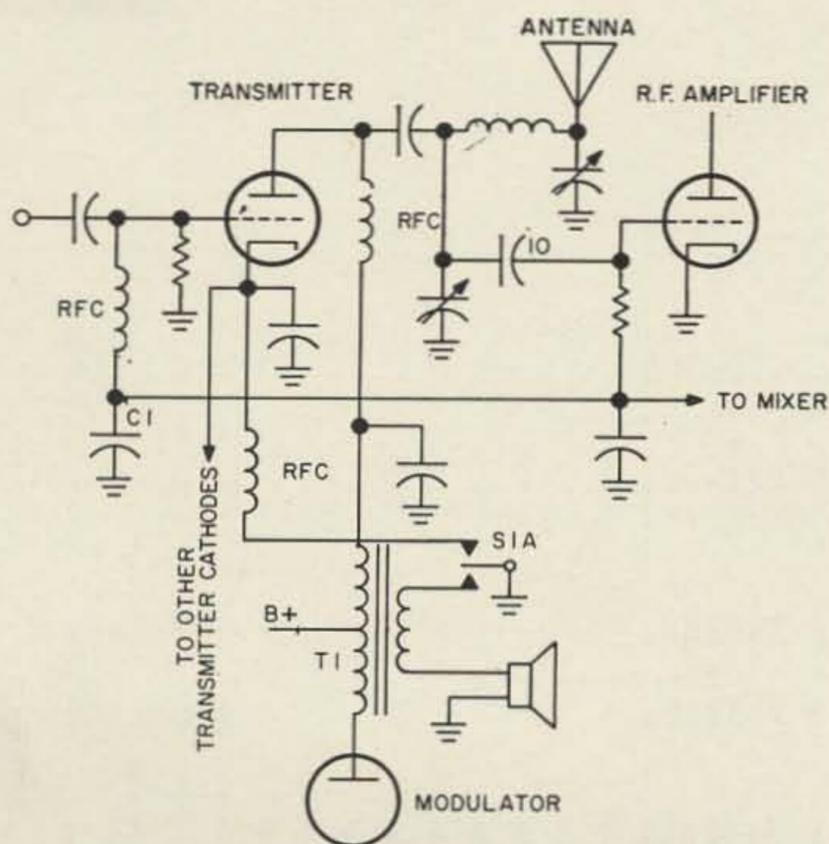
TI - TRANSCEIVER TYPE MODULATION TRANSFORMER
