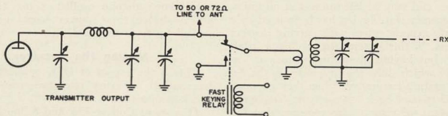
pedence antenna connection. Most modern commercial receivers use 52 or 72-ohm inputs and rf voltages seldom get very high, even with a powerful local transmitter. The danger point is the *secondary* of the first rf transformer—at the grid of the rf amplifier. Good practice would be to install the neon lamp from grid to ground of the rf amplifier tube. (Fig. 1 A & B)
