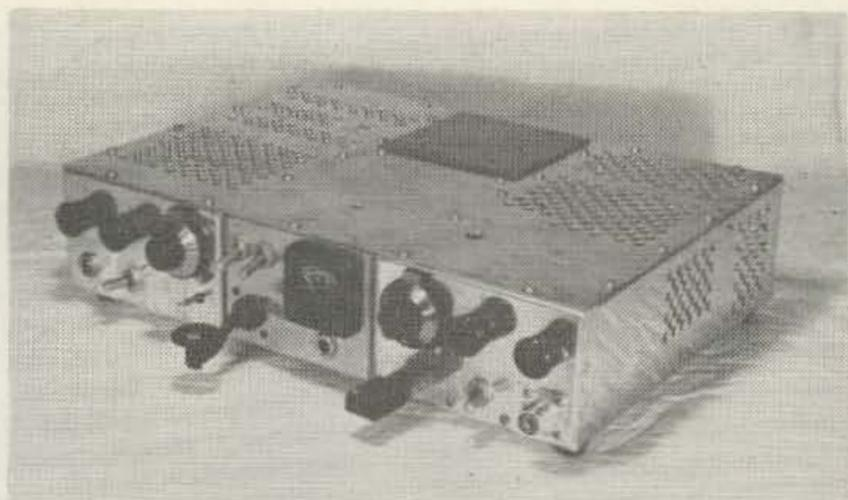
Three quarter view showing panel layout, built-in key, and ventilating holes on side and top of the chassis. The relatively symmetrical layout gave the unit its name.
