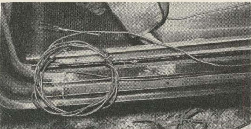
Fig. 8: Photo showing cables in channel to rear engine for tachometer and temperature circuits.
