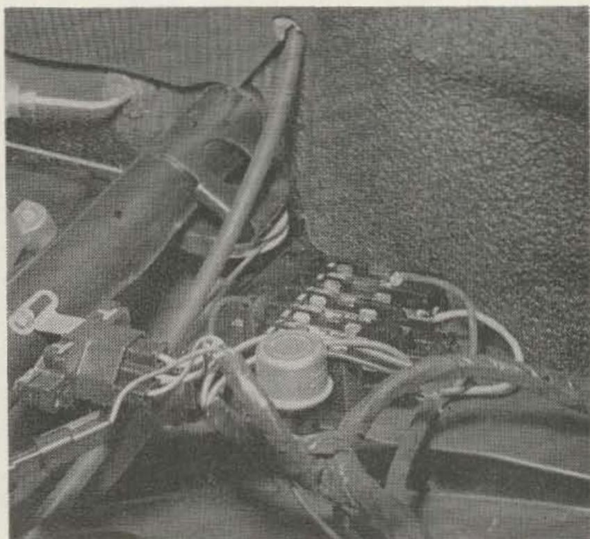
Fig. 10: Battery pickup on fuse block under dash.
