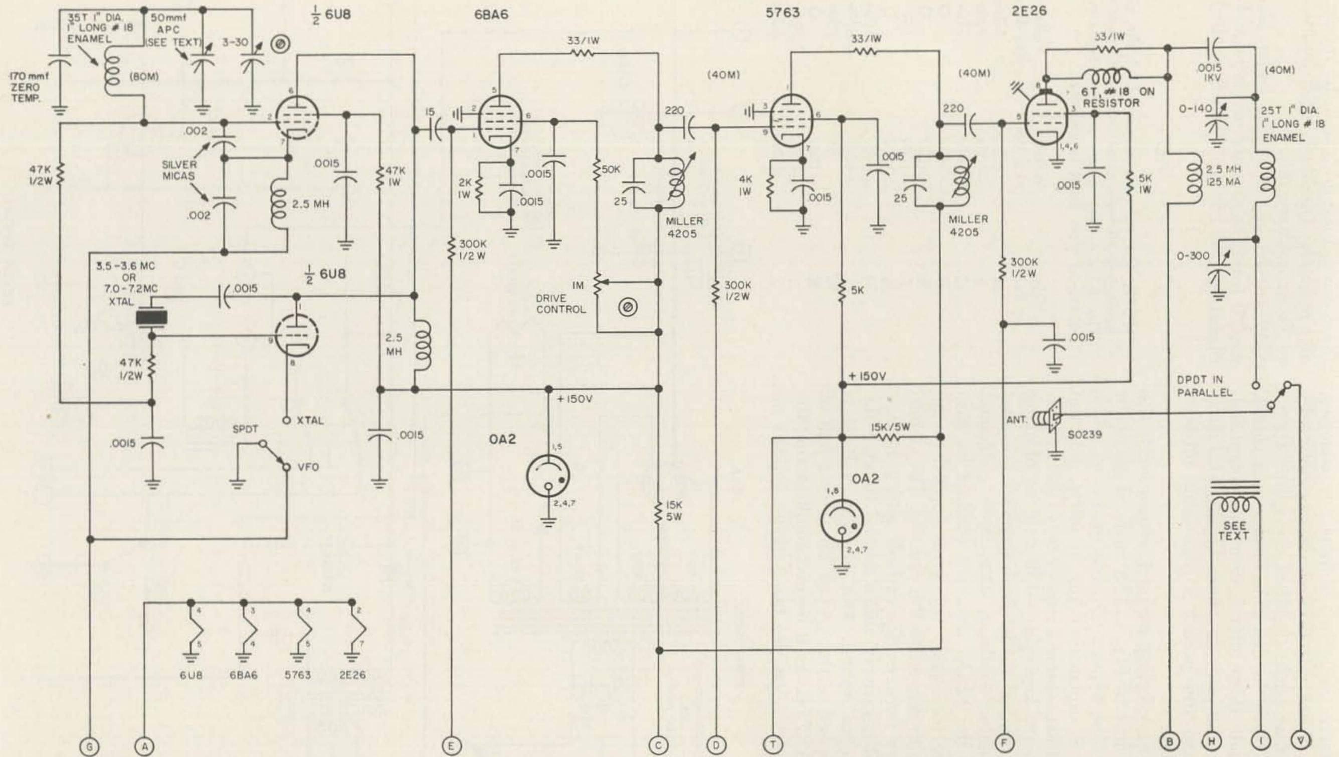
NOTE: All by-pass capacitors are 600v disc ceramics unless otherwise indicated.
