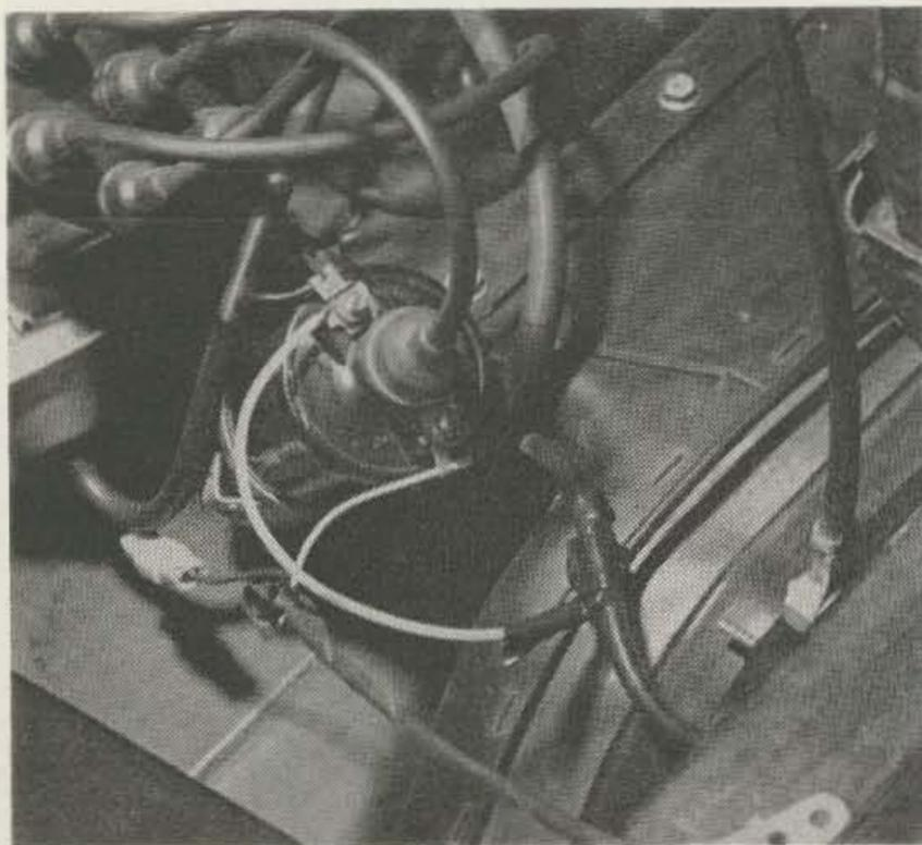
Fig. 9: Photo showing connection of RG-58/U to low side of coil.
