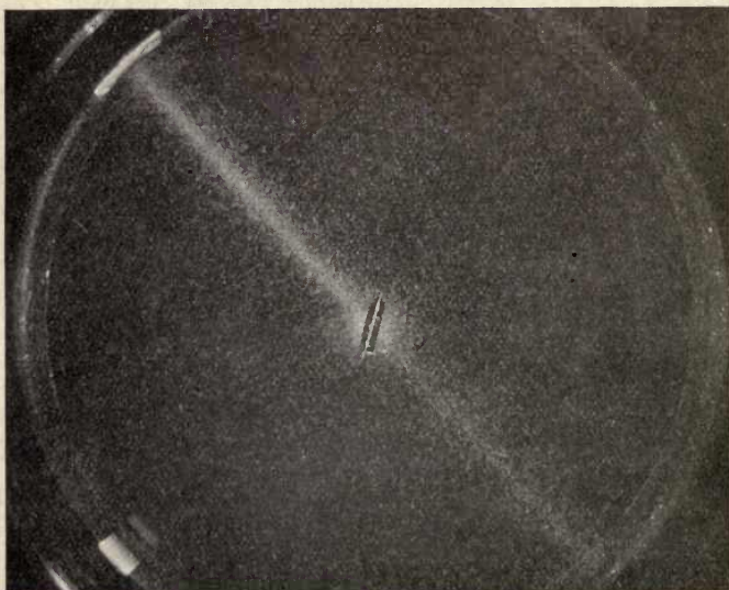
FIG. 2.—Photograph obtained by C. T. R. Wilson showing the passage of X rays (from left to right) through a thin copper plate (see p. 158).
