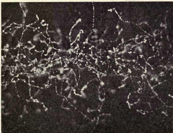
FIG. 76.—Photograph obtained by C. T. R. Wilson of the path of a beam of X rays in air supersaturated with moisture (see p.155). The beam of rays, about 2 mm. in diameter, traversed the air (from left to right of the picture) immediately after the expansion which produced the supersaturation. The axis of the camera was horizontal, and the magnification of the photograph is 6 diameters.
