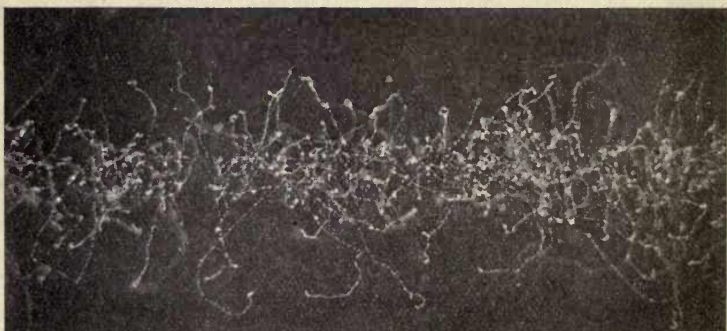
FIG. 1.—Photograph obtained by C. T. R. Wilson of the path of a beam of X rays in supersaturated air. The beam of rays, some 2 mm. in diameter, was sent through the moist air (from left to right in the figure) immediately after the expansion which produced the supersaturation (see p. 155). The axis of the camera was horizontal, and the magnification of the photograph is about 2\frac{1}{2} times.
