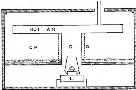
Fig. 58.—Hot Radiating Chamber.
