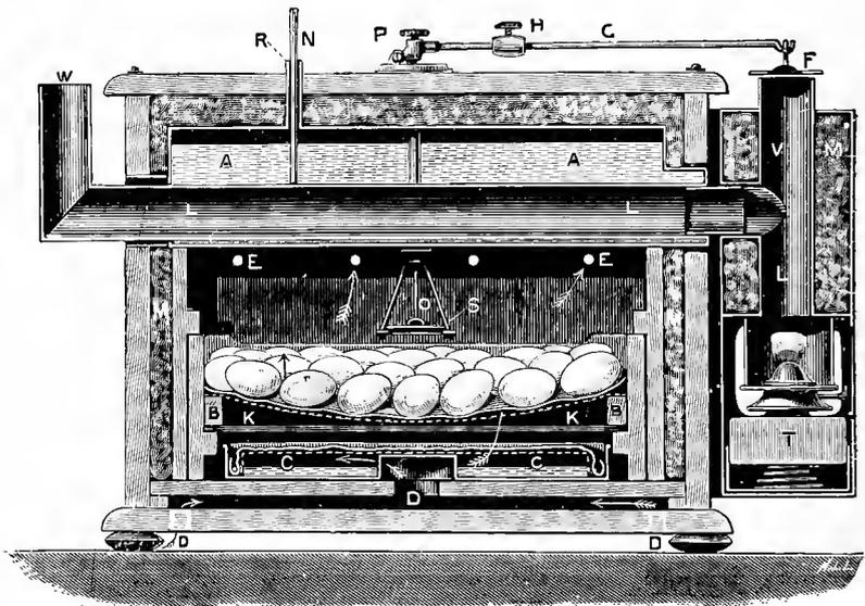
Fig. 35.—A Tank Incubator (Hearson's Pattern).
