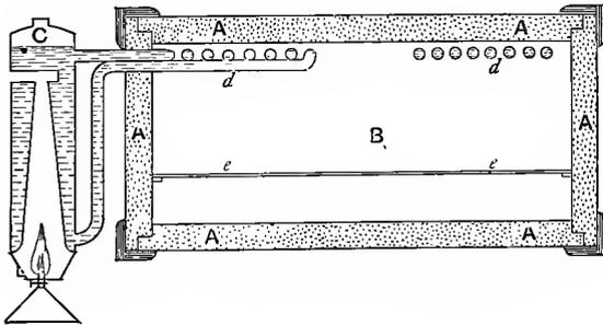
Fig. 44.—Principle of Cyphers' Incubator.
