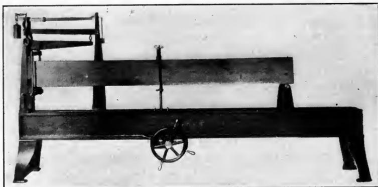
FIG. 31.—Machine for testing light wooden beams.<sup>1</sup>
