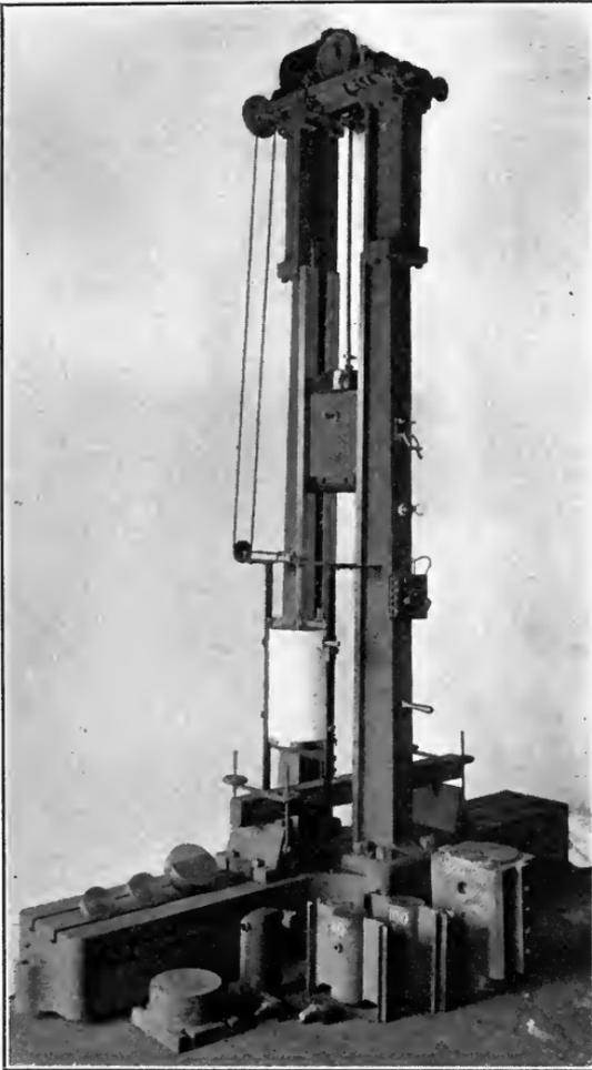
FIG. 38.—Turner impact testing machine.
