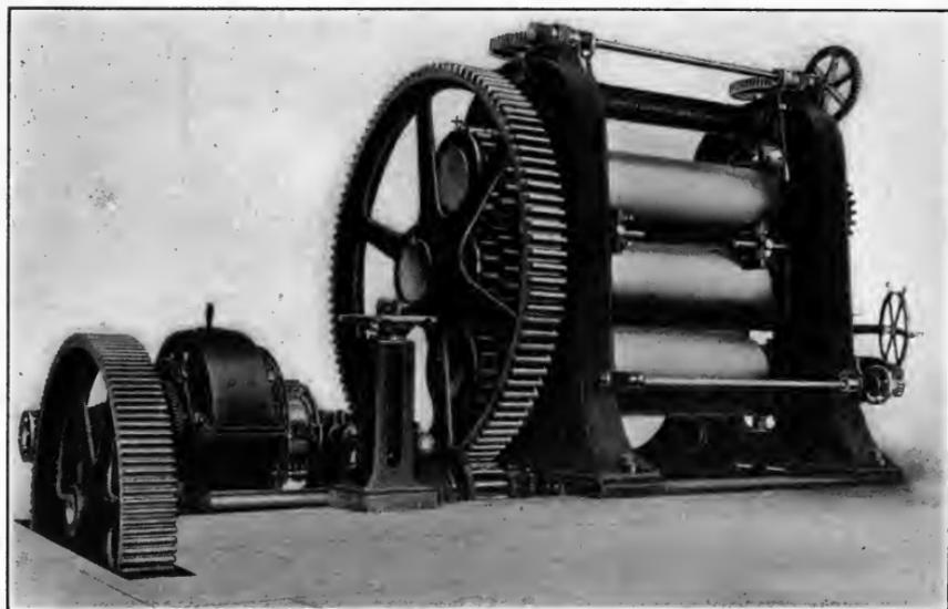
FIG. 90.—Calender with coil clutch motor drive.<sup>1</sup>
