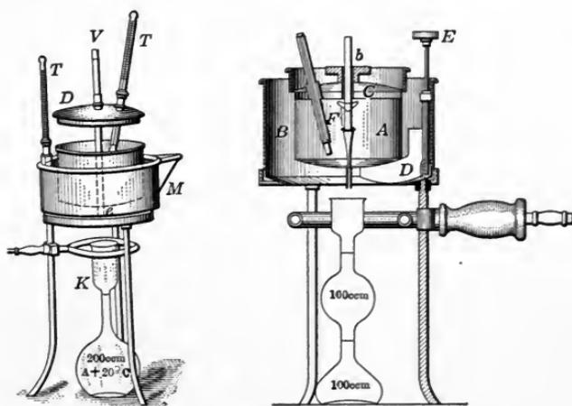
FIG. 86.—Engler's viscosimeter.
