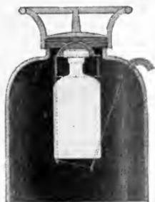
FIG. 46.—Section through portable fire extinguisher.
