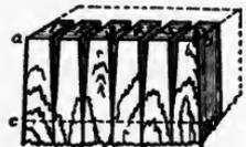
FIG. 41.—Result of unequal shrinkage. The formation of checks.<sup>1</sup>
