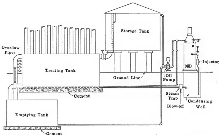
(b) Tank with Horizontal Bottom—The Poles Stand Vertically—The Process is With Change of Oil.
