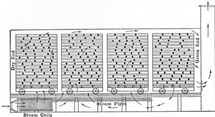
FIG. 70.—A scheme for a radiator kiln.
