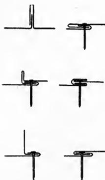
(c) Method of Joining and Fastening Tin.
