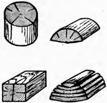
FIG. 40.—Defects due to unequal shrinkage.<sup>2</sup>
