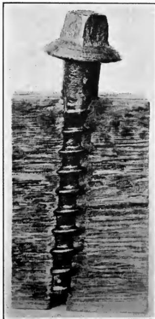
FIG. 35.—Displacement caused by screw spike. Photograph, Spencer Otis Company.
