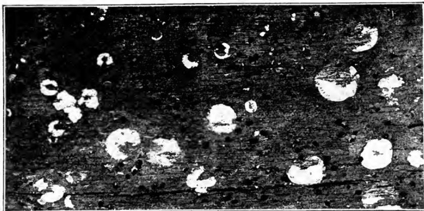
Surface of Wood recently Occupied by Shipworms. Life Size.
