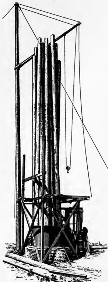
FIG. 76.—Open-tank for Butt treatment of long poles. From "Preservative Treatment of Poles," Kempfer (United States Forest Service, Bulletin No. 84).
