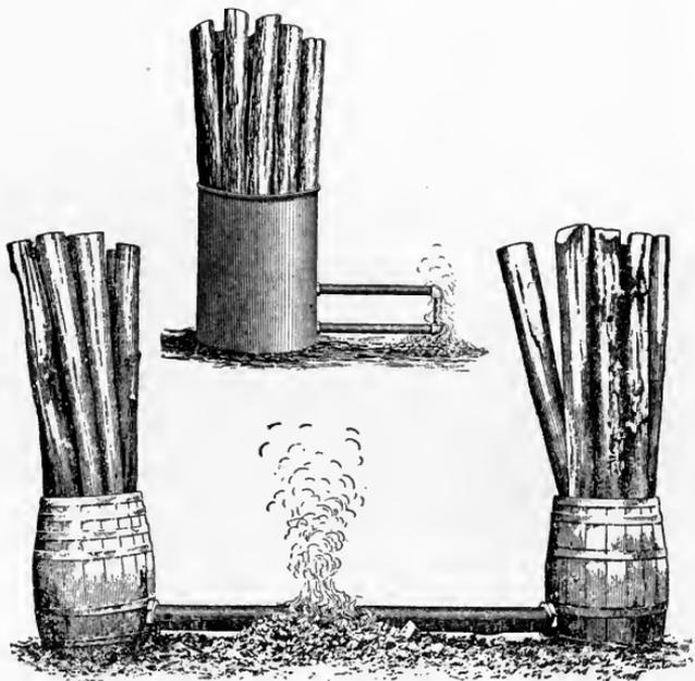
FIG. 77.—Simple apparatus for treating posts.<sup>1</sup>
