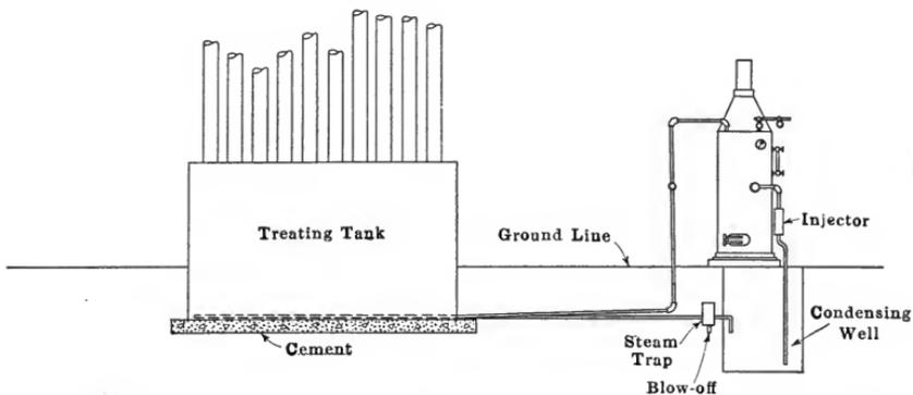
(a) Tank with Horizontal Bottom—The Poles Stand Vertically—The Process is Without Change of Oil.
