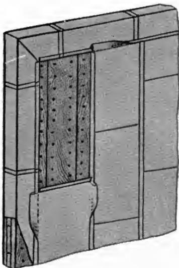
FIG. 45.—Corner of tin-clad fire door.
