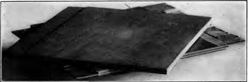
FIG. 85.—Portion of three-ply panel.
