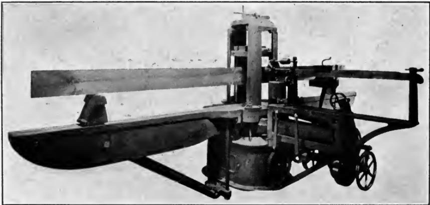
FIG. 32.—Machine for testing heavy wooden beams.<sup>1</sup>
