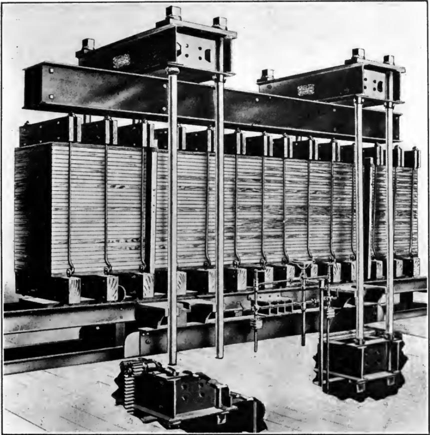
FIG. 83.—Large double-cylinder veneer press.<sup>1</sup>
