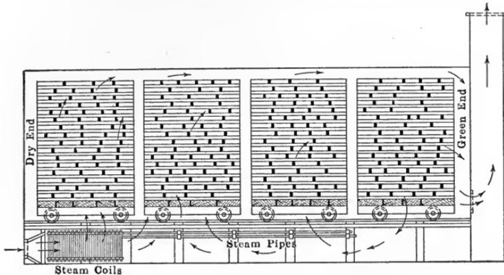
FIG. 70.—A scheme for a radiator kiln.
