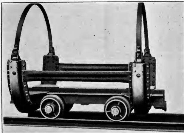
FIG. 78.—Pressed-steel car for cylinder-treatment of ties.<sup>1</sup>
