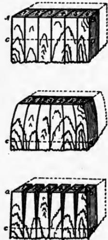
FIG. 41.—Result of unequal shrinkage. The formation of checks.<sup>1</sup>
