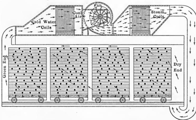
FIG. 71.—A scheme for a blower kiln.
