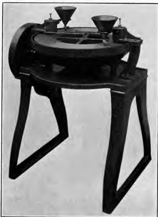
FIG. 39.—Dorry machine for making abrasion tests.
