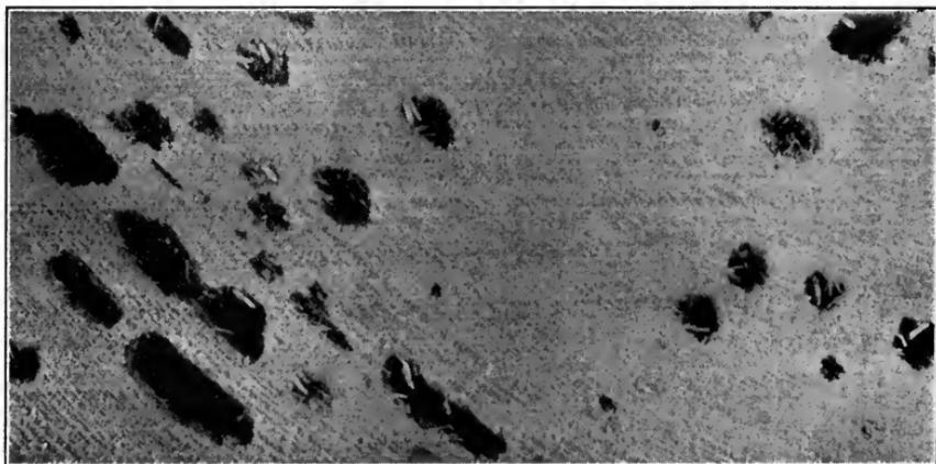
FIG. 44.—Section of wood cut from cypress after attack by wood-destroying fungus (*Dædalea vorax*).
