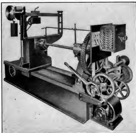
FIG. 33.—Olsen machine for making torsion tests.
