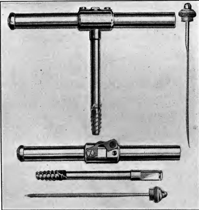
FIG. 22.—Instrument for removing cores to determine ages of trees.<sup>1</sup>
