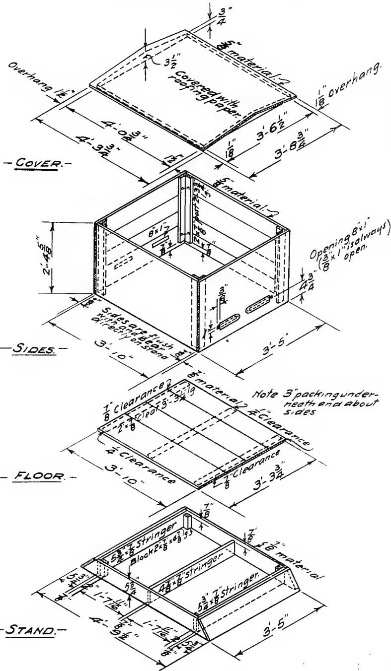
It is convenient to make the case collapsible. The sides may be held together by hooks, or they may be held together more firmly by means of a thumb-screw placed near the top and operated from the inside in combination with dowels in the floor to prevent spreading below, the thumb screws and dowels to be held in cleats fixed on the sides.
