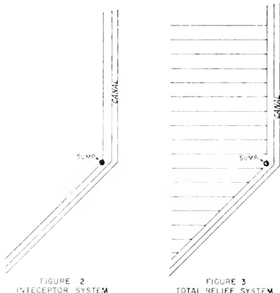
The term "perimeter interceptor" is applied to fields surrounded by a single-line drain, several of which exist in the area studied.
