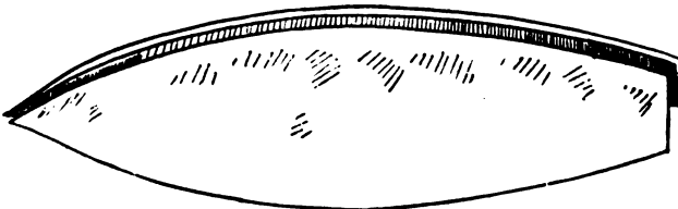
FIG. 99.—Folded Gore with a second Gore over it, ready for Pasting.
