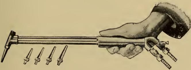
be detached, and several of different capacity are supplied with each torch, which allows a considerable range of work to be carried on without changing torches.
