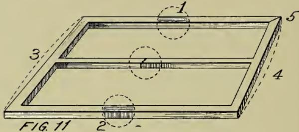
1) Preheating when necessary of broken parts to be welded. 2) Adjusting of flame in blow torch so that operator uses the **neutral flame**, which means avoiding carbonization or oxidization of metal. 3) Annealing or cooling off slowly, after weld has been made, covering weld with lime, ashes or asbestos board so that weld cools about as slowly as when being heated and 4) finishing, practically covers with exception of boiler and a few other lines of work, the whole field of welding.
