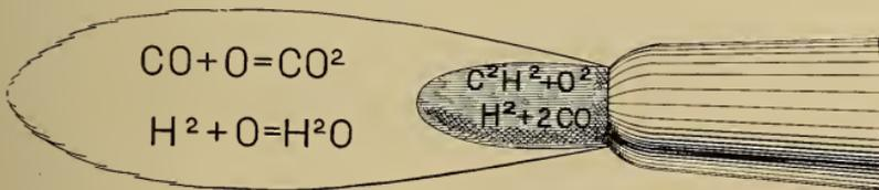
Phases of the combustion in the oxy-acetylene flame.
