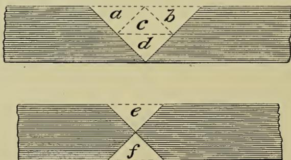
Illustration showing one-half saving in bevelling weld from both sides when possible; "E" "F" spaces being equal to "A" "B" spaces; and "C" and "D" extra spaces to be filled when bevelling from one side.
