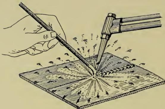
The metal added must not fall, drop by drop, into the weld.
