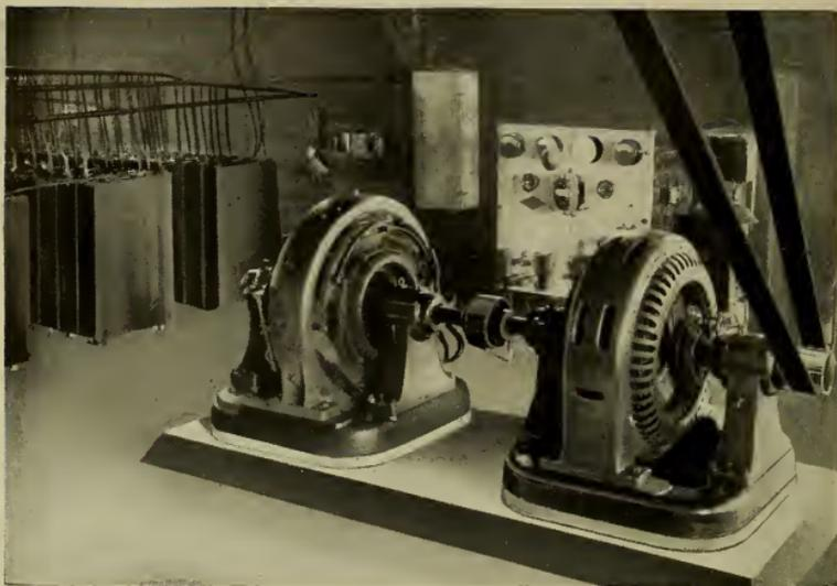
View of a corner of one of our 100 cell oxygen and hydrogen generating plants, making 7500 to 10,000 feet of oxygen gas and 15,000 to 20,000 feet of hydrogen gas, of over 99 per cent purity per day, also showing 150 h. p. motor generating plant.
