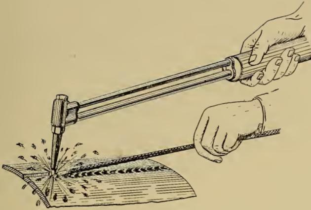
Proper method of holding welding rod.
