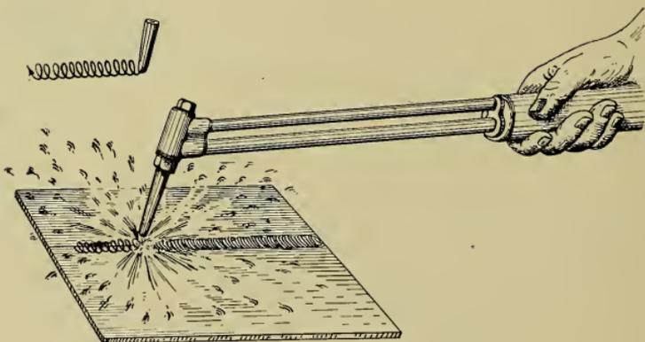
Side to side movement for the execution of welds of greater thickness.
