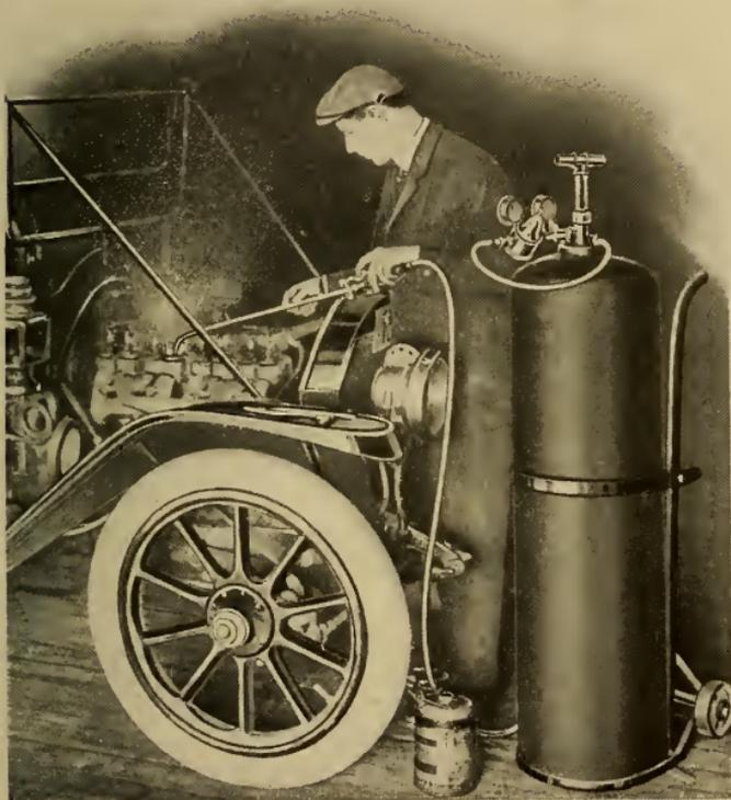
Oxygen Carbon Burner at Work.
