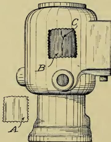
To weld interior surface of a motor cylinder cut out patch "A" weld crack "C" then weld patch "A" in space "B."
