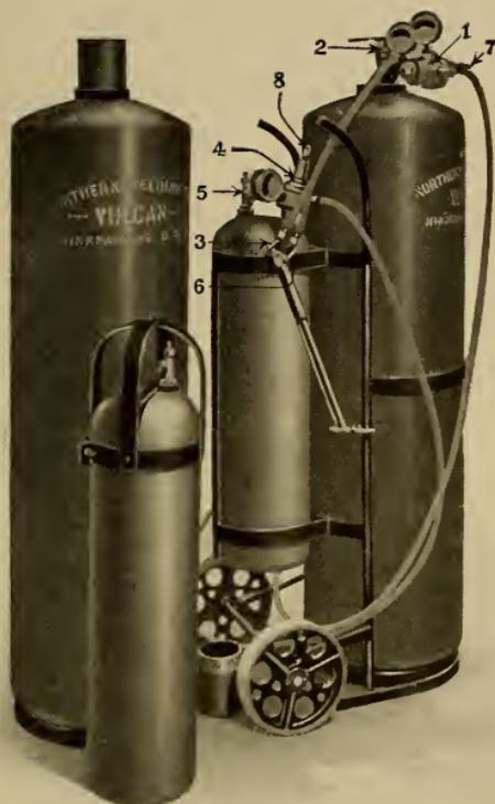
Vulcan No. 2 portable plant, showing low pressure oxygen drums.
