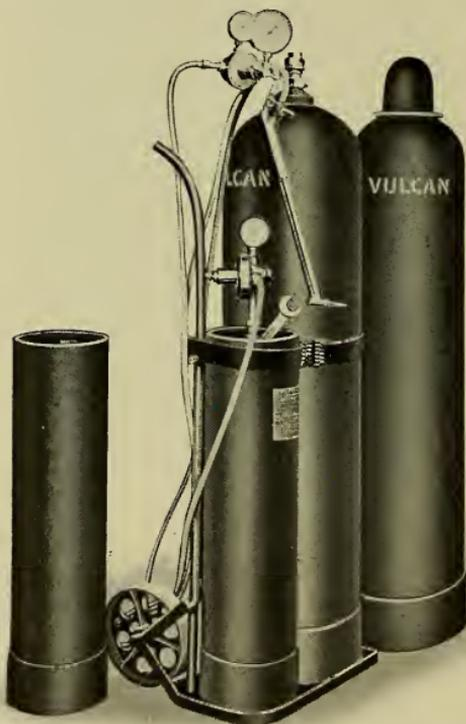
Showing high pressure oxygen drums containing 200 cu. ft. each. Weight of these 200 cu. ft. oxygen drums approximately same as low pressure 100 cu. ft. drums thus saving one half of freight expense. Cut also shows two 100 cu. ft. acetylene drums.
