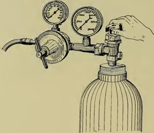
Valve on top of oxygen drum should be opened very slowly and left wide open while in use.
