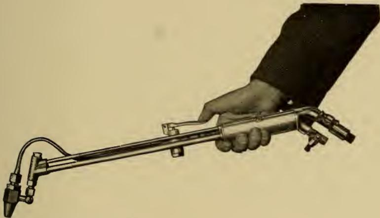
Cutting torch which cuts steel 2" thick x 1 ft. wide in 1 minute; or cuts a battleship slab of steel 4 ft. x 4" in 7 minutes.
