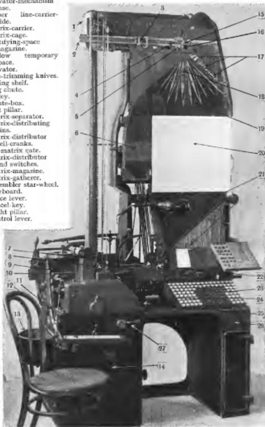
FIG. 428.—Bellows or Electric compositor: front view.
