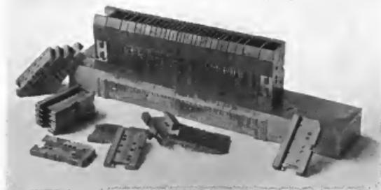
FIG. 207.—Bellows of Electric compositor matrices with slug.
