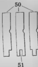
FIG. 327.—(Fig. 4. in patent abridgment.) Grant-Logros-Maw line-justifying machine. Type with special foot-nick.
