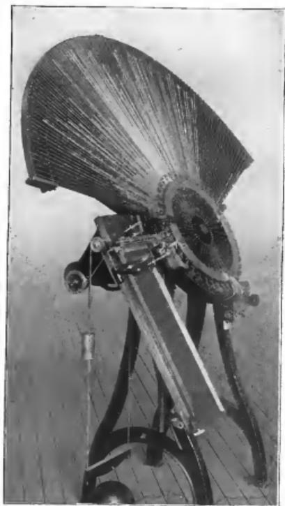
FIG. 336.—Dow automatic distributing machine.
