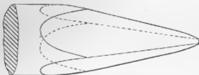
FIG. 152.—Roughing or chisel tool for punch-cutting machine.
