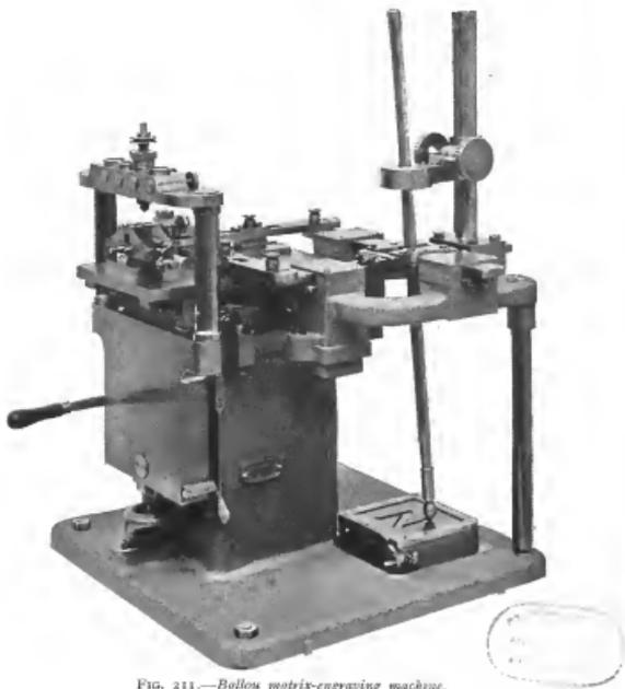
FIG. 211.—Bullow matrix-engraving machine.
