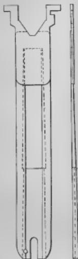
FIG. 201.—*Linotype; wedge-space matrix, or space-band.* Scale: full size.
