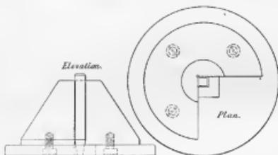
FIG. 145.—Jointer or stone-facer for punches. Half size.
