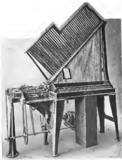
FIG. 325.—Wicks composing machine; with Stringer line-justifier attached.
