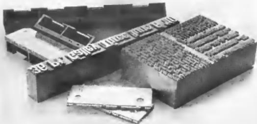
FIG. 255.—Bellows or Electric compositor, slugs.
