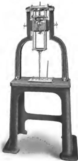
FIG. 212.—Matrix-engraving machine; American Type Founders Co.
