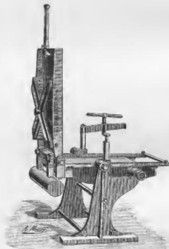
FIG. 469.—Casting-press for flat stereotype-plates: open.
