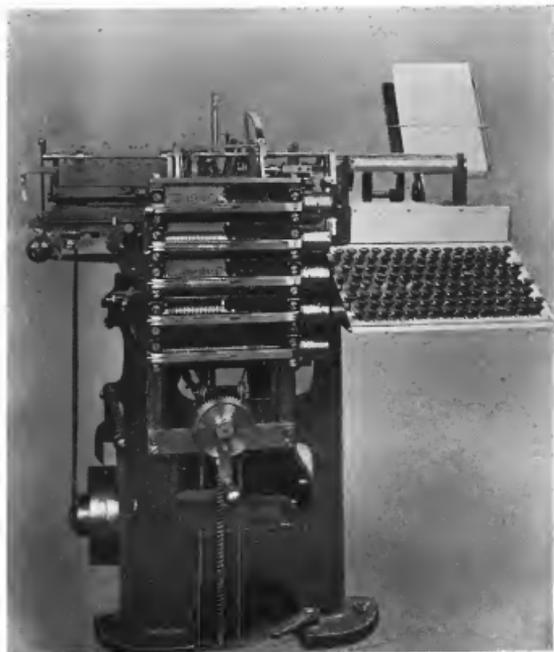
FIG. 337.—Rototype composing and casting machine.
