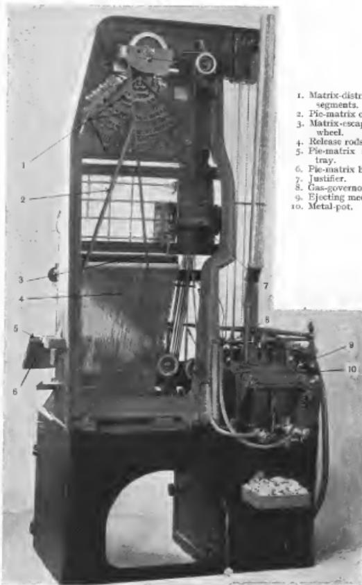
FIG. 429.—Bellows or Electric compositor; back view.
