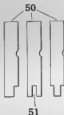
FIG. 327.—(Fig. 4, in patent abridgment.) *Grant-Legros-Maw line-justifying machine. Type with special foot-wicks.*
