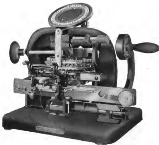
FIG. 88.—Embossing machine: hand "Graphotype"; Addressograph.
