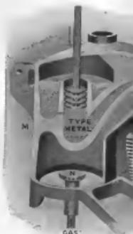
FIG. 418.—Linotype; metal-pot and mould.
