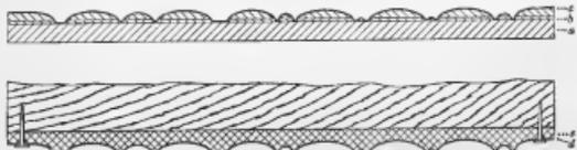
FIG. 486.—Section of typographical etching-plate showing plate with wax built up for whites, and section of the electrotyped shell filled and mounted.
