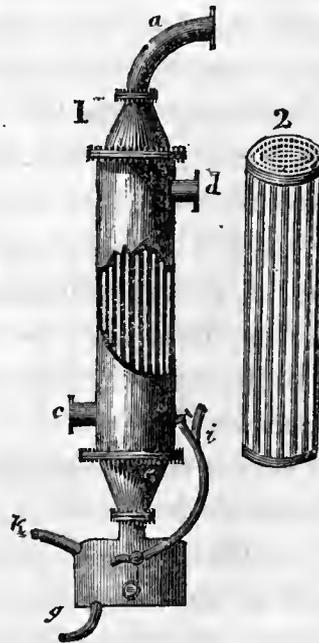
The elbow pipe *a*, No. 1 of Fig. 27, is connected by one flanch with the eduction way of the engine, and by the other to the cone of the condenser, which for a 10 horse power engine, is a cylindrical vessel of 3 feet 6 inches long, and 7 inches internal diameter. In this cylinder are placed in circles forty copper tubes, 5-8ths in diameter, which are inserted into
