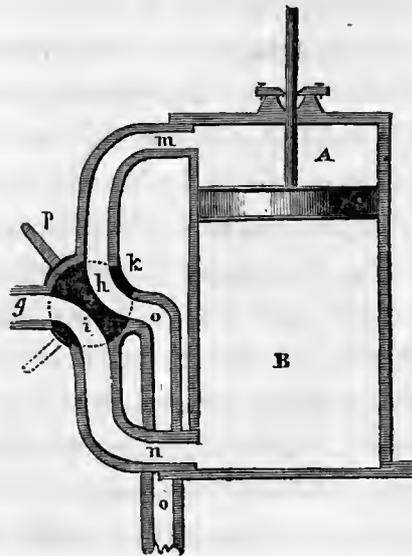
Let **A B** represent a section of a steam engine cylinder, with the rod of its piston, working as before, through an air-tight stuffing box, and **g** the pipe that brings steam from the boiler, and which terminates near the cylinder, in the four (or rather two) way cock **h i k** and the pipes **m n o**, which are drawn much larger than they should be, in proportion to a
