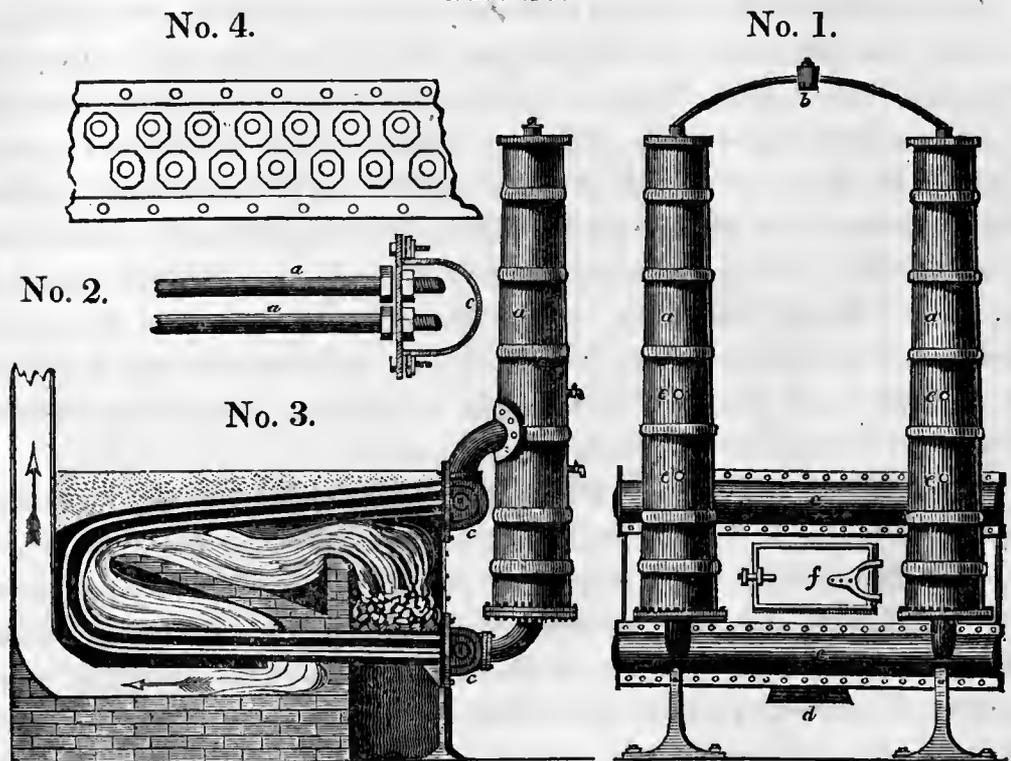
Fig. 26, No. 1, represents a front view of this boiler; *a, a,* are the chambers into which the steam and water are received when generated in the tubes, and are there separated from each other by the steam rising, and the water falling to the bottom; these chambers are therefore called *the sepa-*
