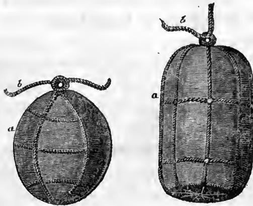
*a a* the two fenders, *b b* the ropes by which they are suspended.
