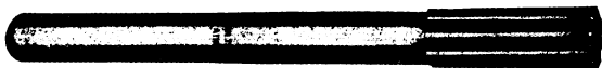
Fig. 54. Rose Fluted Chucking Reamer Courtesy of Union Twist Drill Company, Athol, Massachusetts
