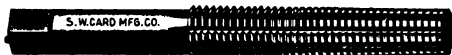
Fig. 111. Hob for Cutting Full Threads Courtesy of S. W. Card Manufacturing Company, Mansfield, Massachusetts
