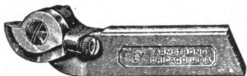
Fig. 98. Threading Tool for Hand Taps Courtesy of Armstrong Brothers Tool Company, Chicago
