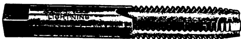
Fig. 106. Tap Showing Method of Filing Away Teeth at the Point Courtesy of Wiley and Russell Manufacturing Company, Greenfield, Massachusetts
