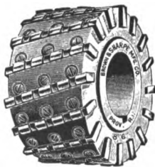
Fig. 213. Spiral Cutter with Inserted Teeth Courtesy of Brown and Sharpe Manufacturing Company, Providence, Rhode Island
