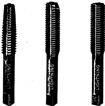
Fig. 97. Types of Hand Taps. Left-Taper Tap; Center-Plug Tap; Right-Bottoming Tap Courtesy of Wiley and Russell Manufacturing Company, Greenfield, Massachusetts
