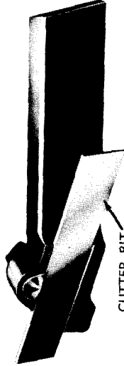
STRAIGHT PARTING CUTTING TOOL HOLDER WITH CUTTER BIT
