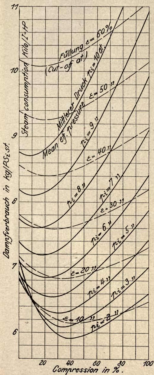
Fig. 10. Saturated steam 14 at. abs. Noncondensing, Clearance space 5%.
