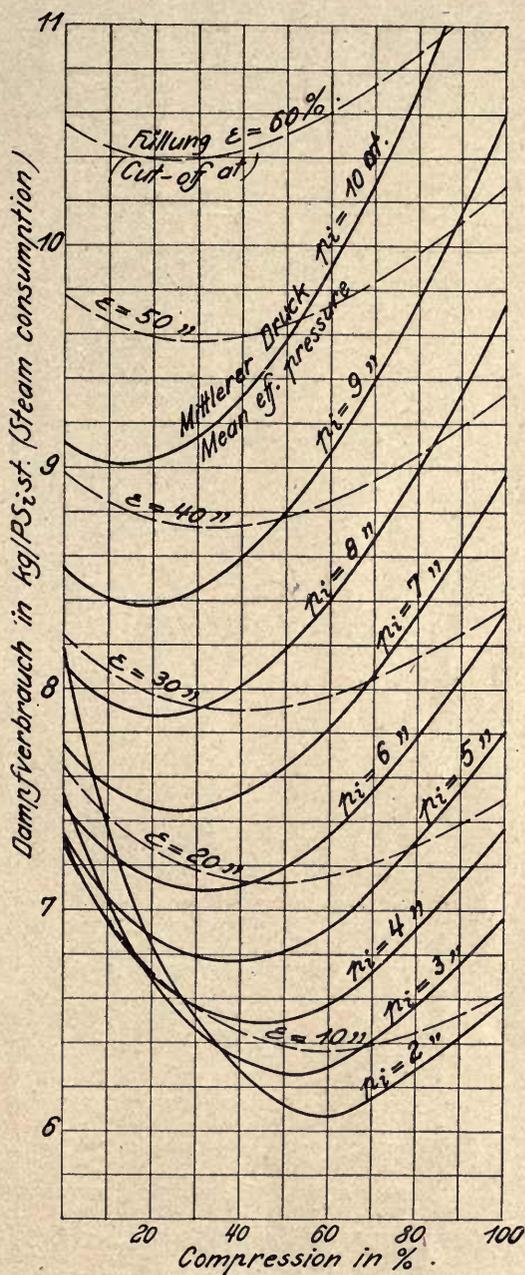
Fig. 11. Saturated steam 14 at. abs. Noncondensing, Clearance space 8%.
