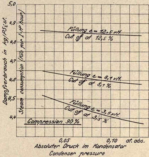
Fig. 31. Superheated steam 300° C, 13 at. abs.
