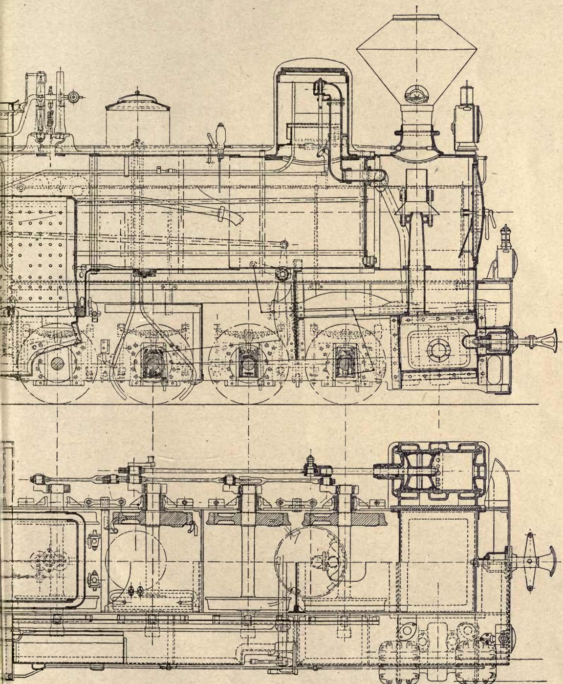
The superheater una-flow locomotive is at least on a par with the superheater compound, although even here the former has a slightly higher fuel consumption for heavy loads. Larger cylinders are of course more feasible with the una-flow system than with the compound engine.
