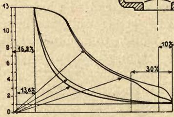
It is the policy of the Kolomna Engine Works, in cases where superheating is not acceptable, to obtain improved economy by applying the una-flow system. In this way they rebuilt with una-flow cylinders eleven saturated steam locomotives of the tank type of the Warsaw narrow gage railway during the years 1913—1914. These una-flow cylinders are fitted with piston valves and have the cylinder ends jacketed, in addition to the heads.
