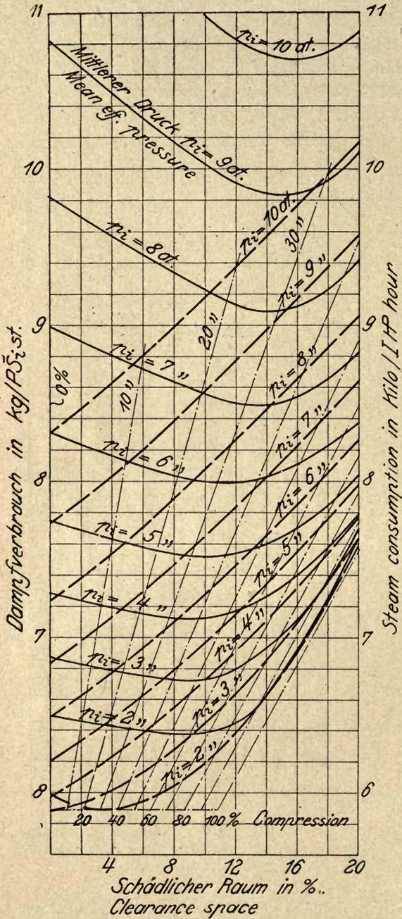
Fig. 19. Saturated steam 14 at. abs. Noncondensing.
