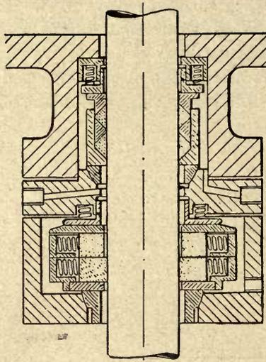
Type A Simplex packing for steam pressures up to 6 at.
