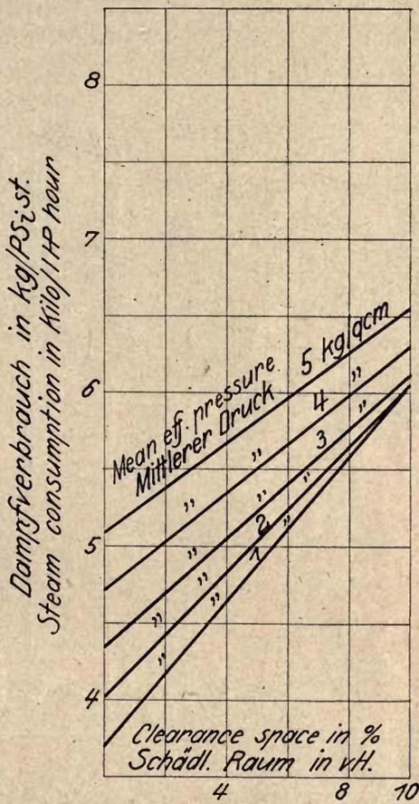
Fig. 22. Saturated steam 13 at. abs. Condensing (0.1 at. abs.).
