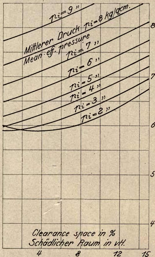
Fig. 21. Saturated steam 13 at. abs. Noncondensing.
