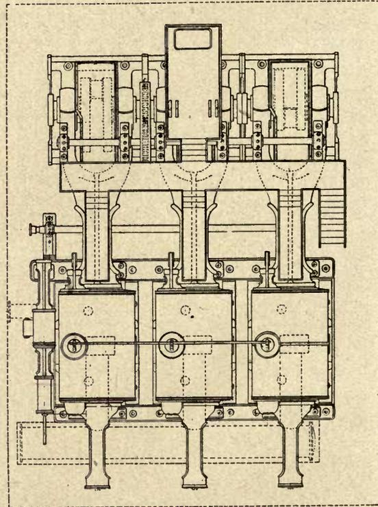
and the cut-off falls to practically 35%. A considerable saving of steam and increased safety of operation are the result. The limitation of the maximum cut-off of the main valve has the advantage that for early cut-offs the port openings are considerably improved, which is especially important in view of the essentially unfavorable valve opening consequent on the use of crossed eccentric rods.
