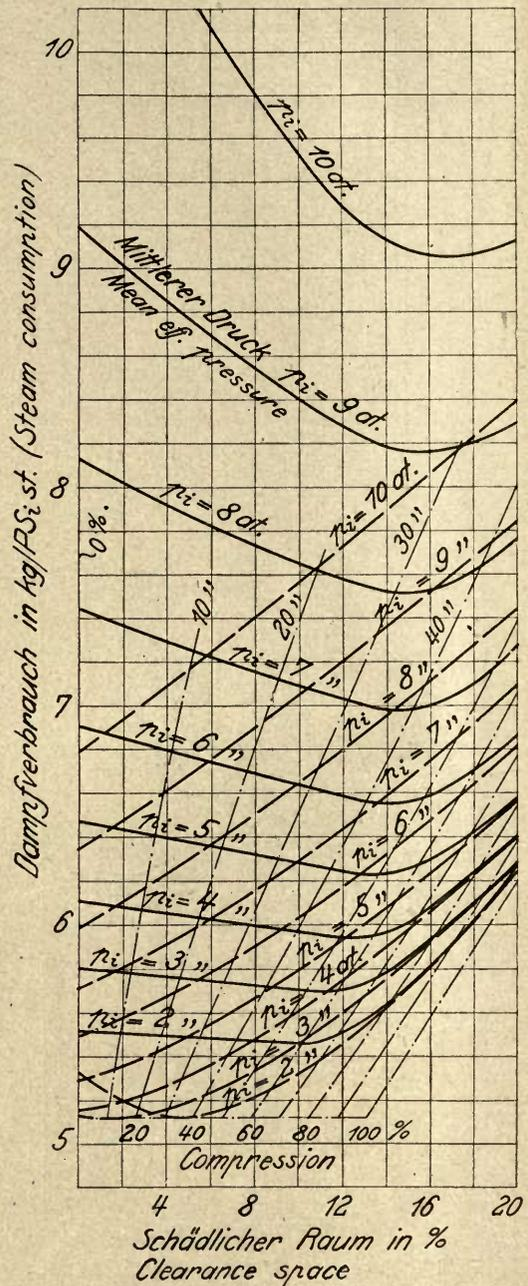
Fig. 20. Superheated steam 300° C, 14 at. abs. Noncondensing.
