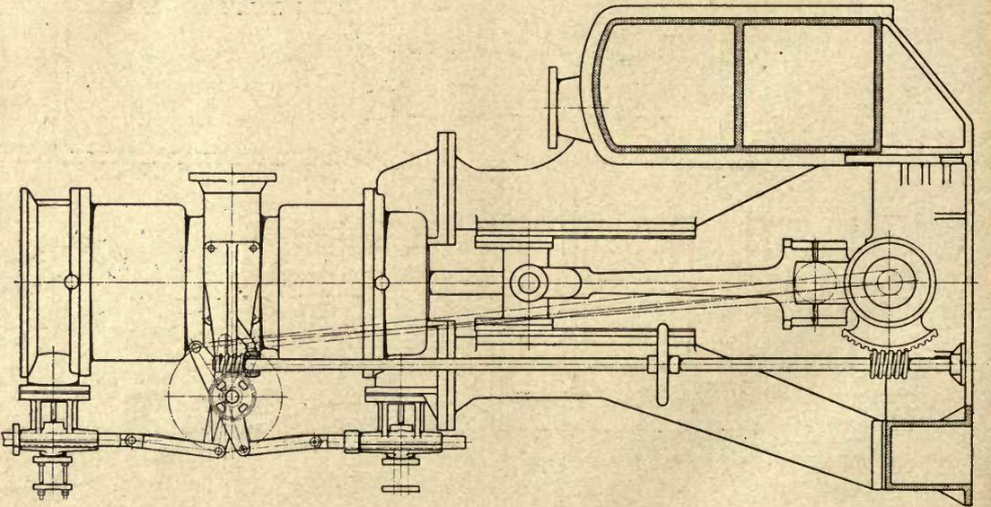
In Fig. 27 is illustrated a two-cylinder una-flow marine engine built by the Kingsford Foundry & Machine Works, of Oswego, N. Y. This engine is fitted to
