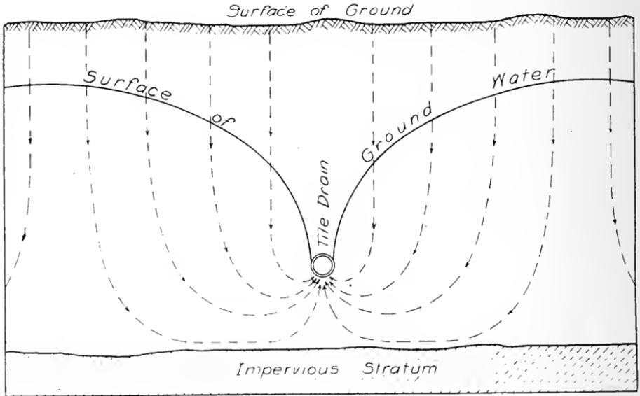
Fig. 6. Diagram Illustrating the Movement of Water from the Surface to the Drain.
