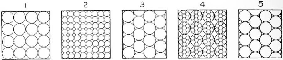
Fig. 3. Ideal Arrangement of Spherical Soil Particles.
