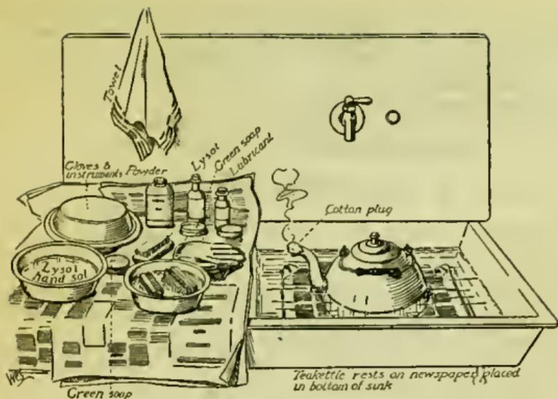
Figure 2. Sink Set-Up.
