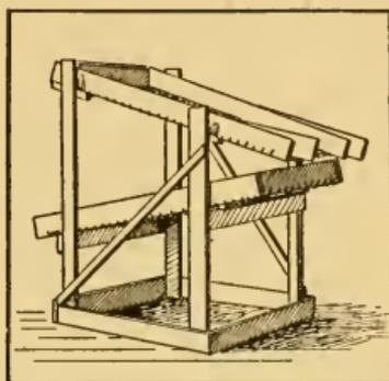
FIGURE 40.—An easily constructed potato grader.
