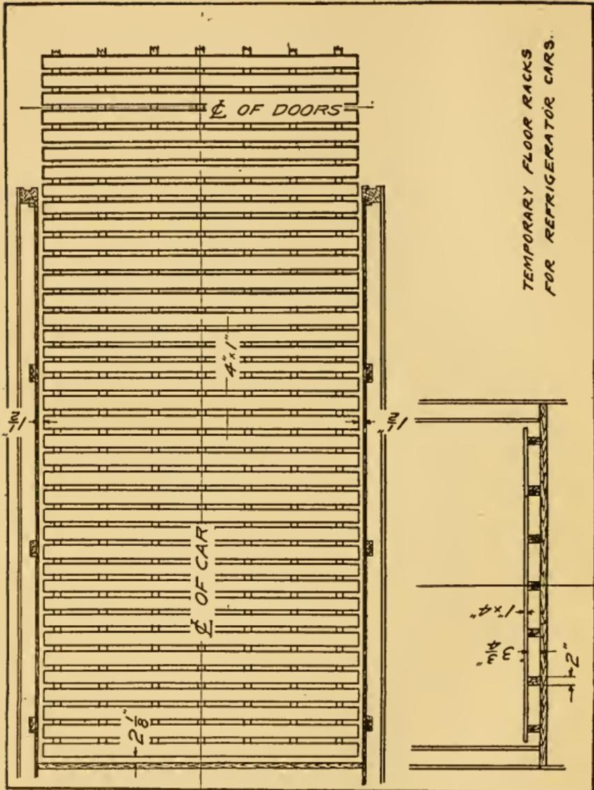
FIGURE 42.—Temporary floor racks for refrigerator cars.
