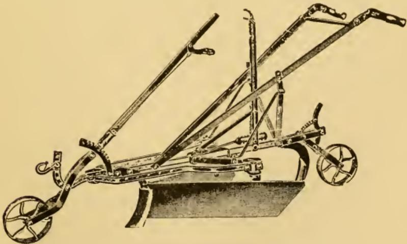
FIGURE 11.—Five-tooth cultivator with banker attachment.
