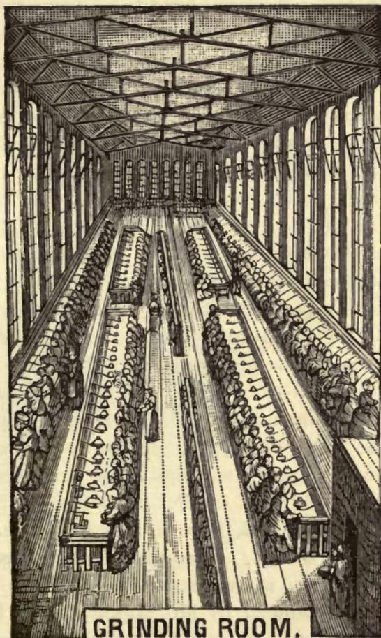
room more than 160 girls are busily employed cross and straight grinding steel pens on wood cylinders covered with emery. The room in which the finished pens are placed in boxes measures 54 by 30 feet, and in it alone are employed
