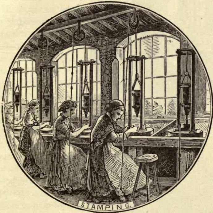
ascend. Taking a handful of blanks with her left hand, by a dexterous motion she makes a little train of them between the thumb and finger in parallel order, presenting the first in the most ready position to be passed to the other hand. The right hand is brought toward the left, and, taking a blank, places it with the point toward the worker in a guide upon the bed of the stamp, then
