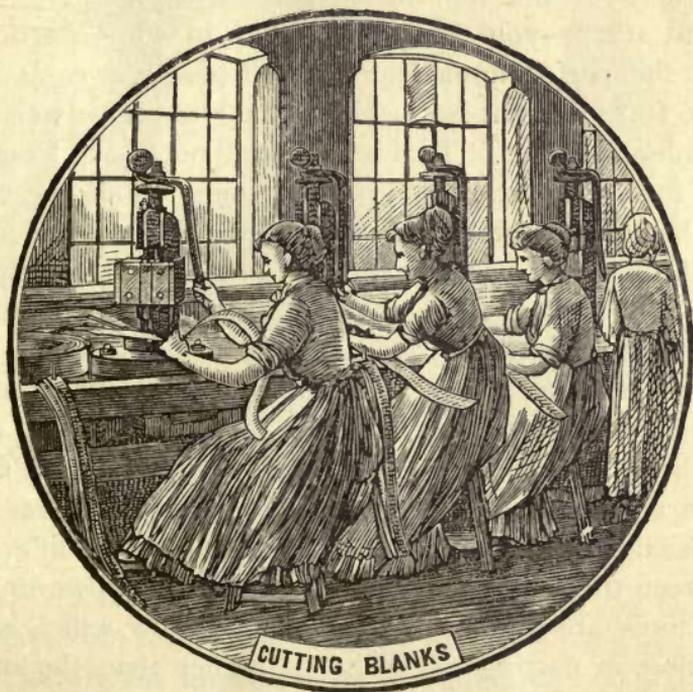
blank. The girl with her left hand introduces one of the strips of steel at the back of the press, and, pulling the handle toward her with the right hand, the screw
