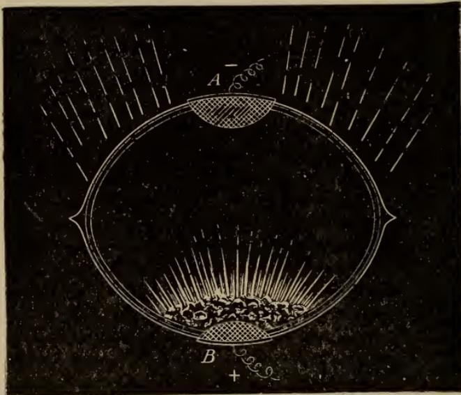
FIG. 69.—Electrical Phosphorescence.
