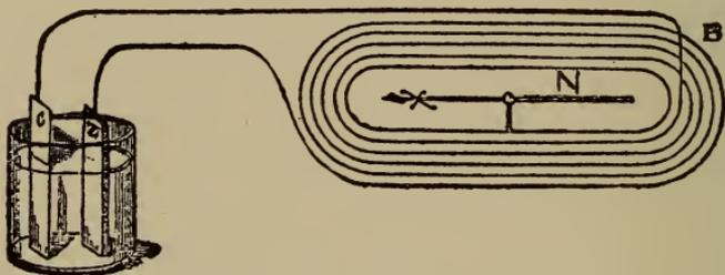
FIG. 30.—The Galvanoscope.
