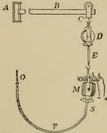
FIG. 82.—An Electric Drill.
