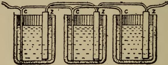
FIG. 14.—Cells in Parallel.
