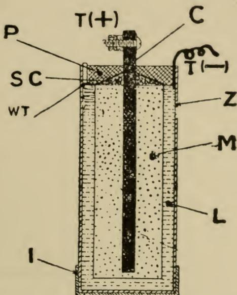
FIG. 19.—The E. C. C. Dry Cell.
