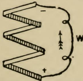
FIG. 23.—Thermo-electric Couples in Series.
