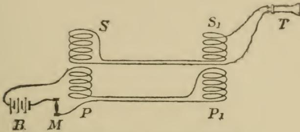
FIG. 92.—The Induction Balance.
