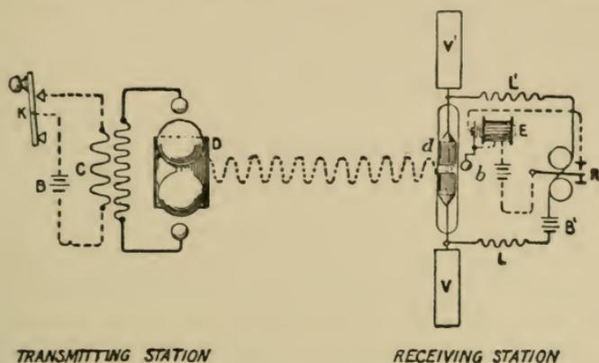
FIG. 102.—Marconi's Apparatus.
