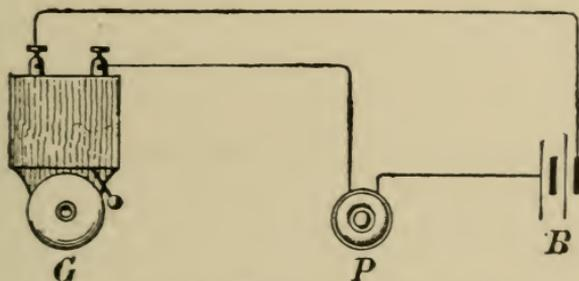
FIG. 83.—An Electric Trembling Bell.
