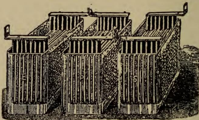
FIG. 21.—The E. P. S. Accumulator.
