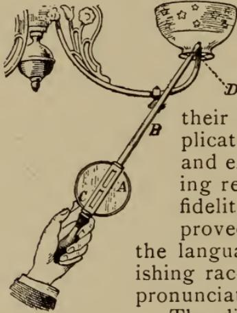
FIG. 95.—An Electric Gas Lighter.
