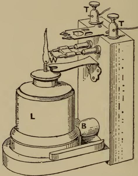
FIG. 96.—An Electric Lamp Lighter.
