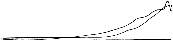
Fig. 14. Diagrams Taken after Adjusting Valve. Scale 40, Head End.
