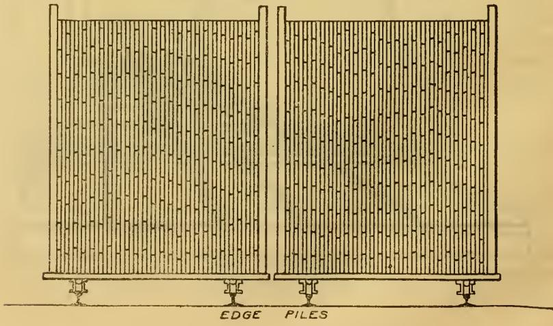
FIG. 17.—Methods of piling lumber for kiln drying.
