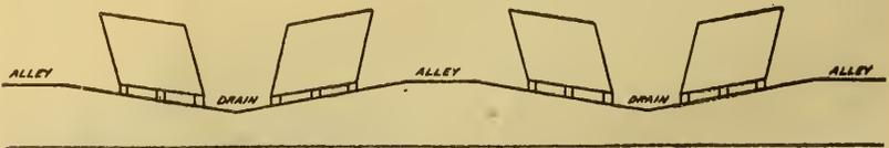
FIG. 15.—Method of providing drainage under lumber piles.
