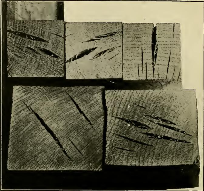
FIG. 1.—HONEYCOMBED OAK TIMBERS, THE RESULT OF CASEHARDENING.
