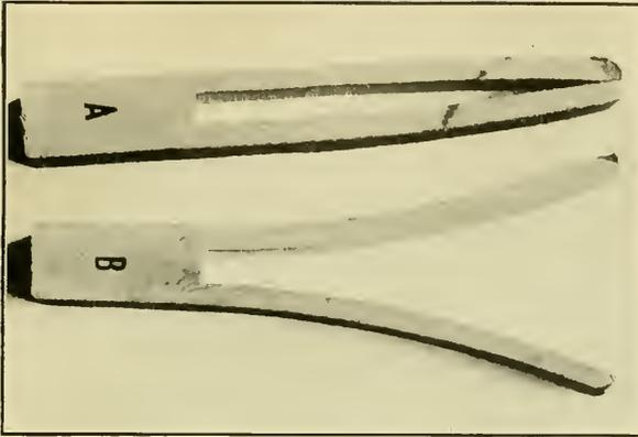
FIG. 1.—SECTIONS CUT FROM CASEHARDENED BOARDS.
