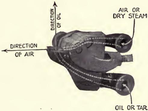
Fig. 1. High Pressure Oil Burner.
