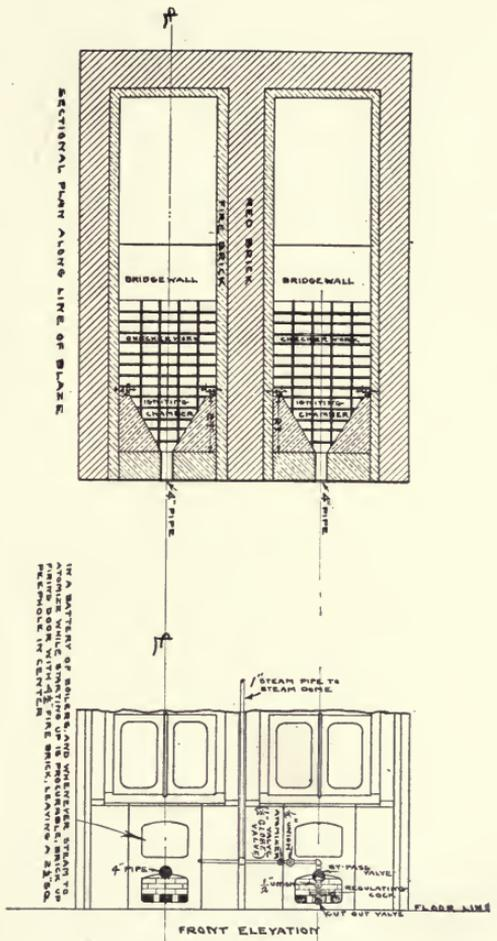
IN A BATTERY OF BOILERS, THE BRICK ARCHES SHOULD BE APPROXIMATELY SIMILAR UP TO REGULAR SIZE, TO PREVENT DOWN DRAFTS OF FIRE BRICK, LEAVING A 25% EXCESS IN THE LARGER ARCHES.
