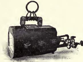
Fig. 2. A portable furnace such as is shown in operation in Fig. 1.
