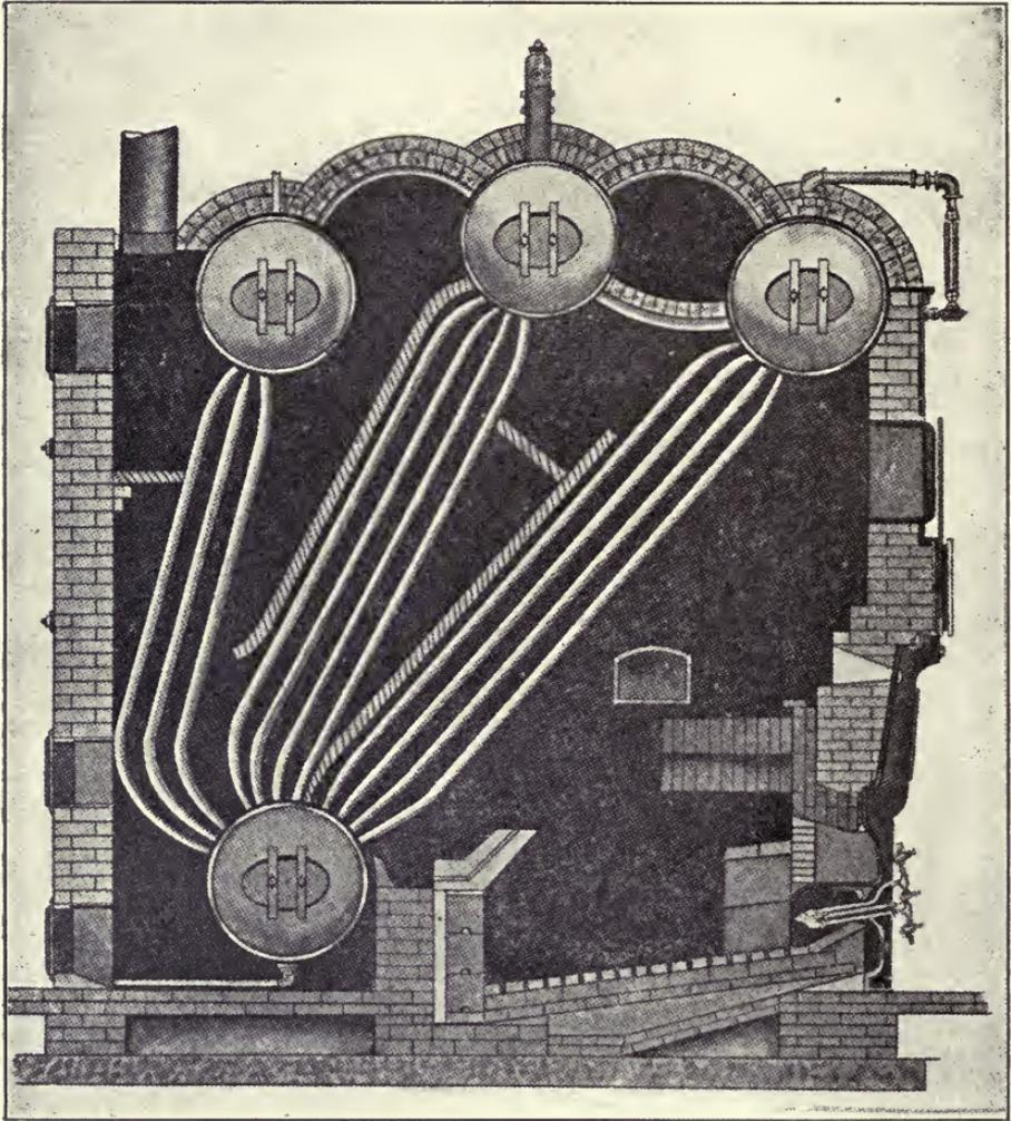
Fig. 6. Stirling Boiler Equipment.
