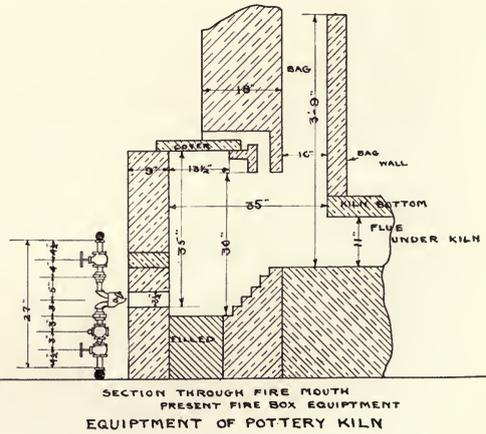
Two ways of equipping a pottery kiln, the type of construction shown in the upper views being the most modern.
