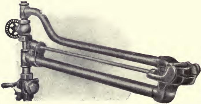
High Pressure Oil Burner mounted for Marine or Stationary Boilers burning oil or tar exclusively as fuel.
