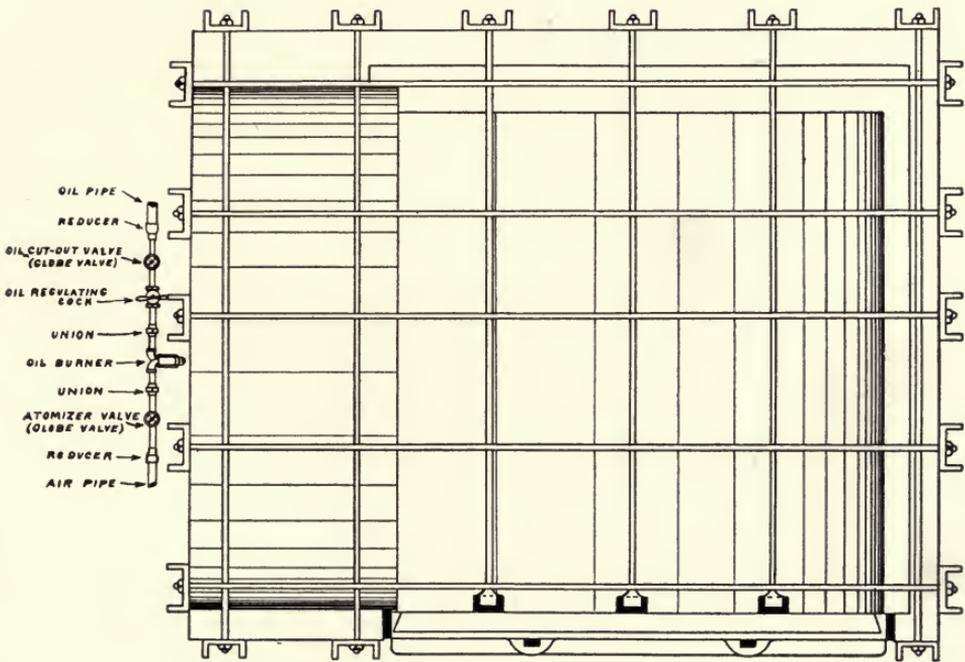
PLATE HEATING FURNACE
