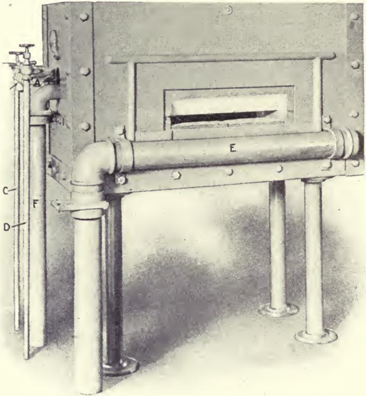
A—Oil burner. B—Oil regulating cock. C—Air pipe. D—Oil pipe.
