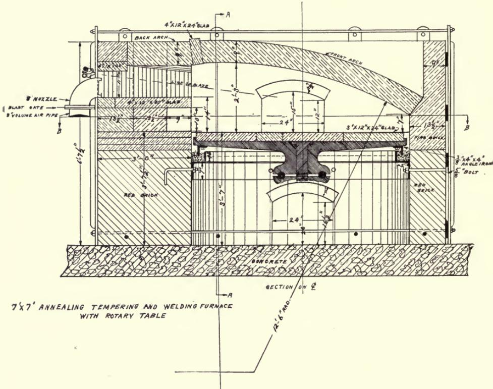
7 ft. x 7 ft. Annealing Furnace with Rotary Table.
