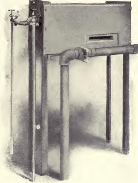
A—Oil burner. B—Oil regulating cock. C—Oil pipe D—Air pipe.
