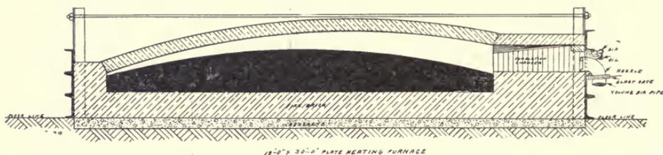
Plate Heating Furnace, charging space 18 ft. x 30 ft.
