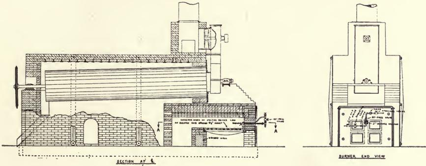
Equipment of Ore or Sand Roaster and Dryer.
