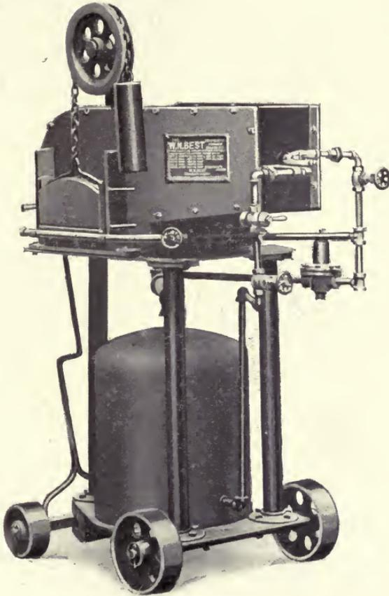
A self-contained portable outfit with 20 gallon oil tank, which can readily be moved around from place to place and which is used for heating 8,000  $\frac{3}{4}$ -in. x 3-in. rivets in ten hours, as well as for forging, tool dressing, etc. Very convenient for small work in shops not equipped with the regular oil system as well as for work where portable outfit is necessary.
