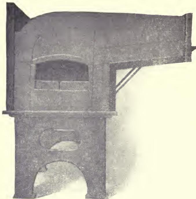
Furnace with front casting removed to show special shaped brick lining.
