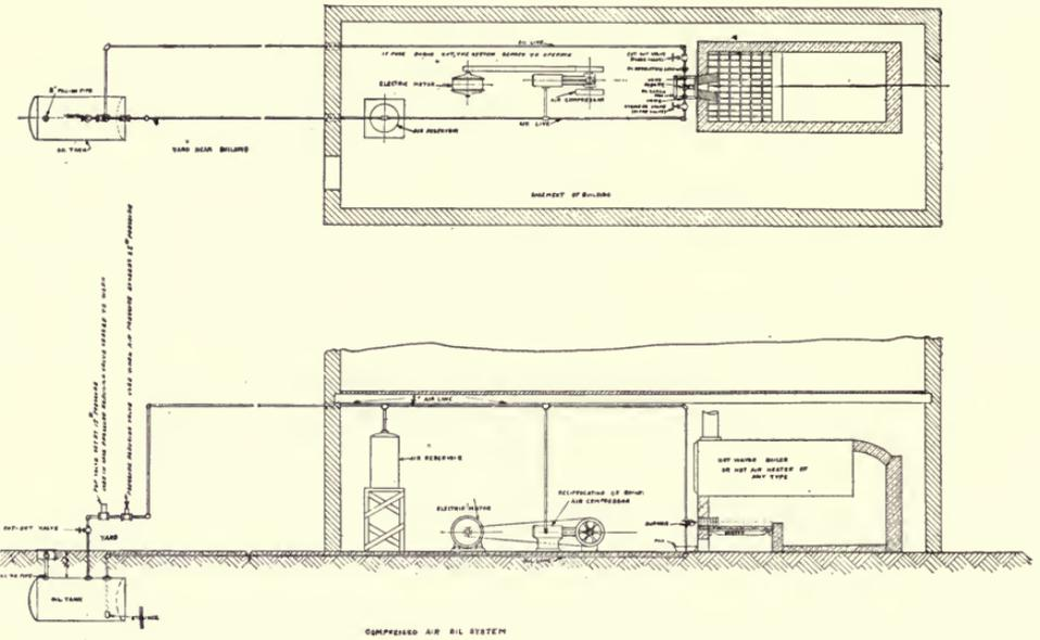
Fig. 4. Compressed Air System.
