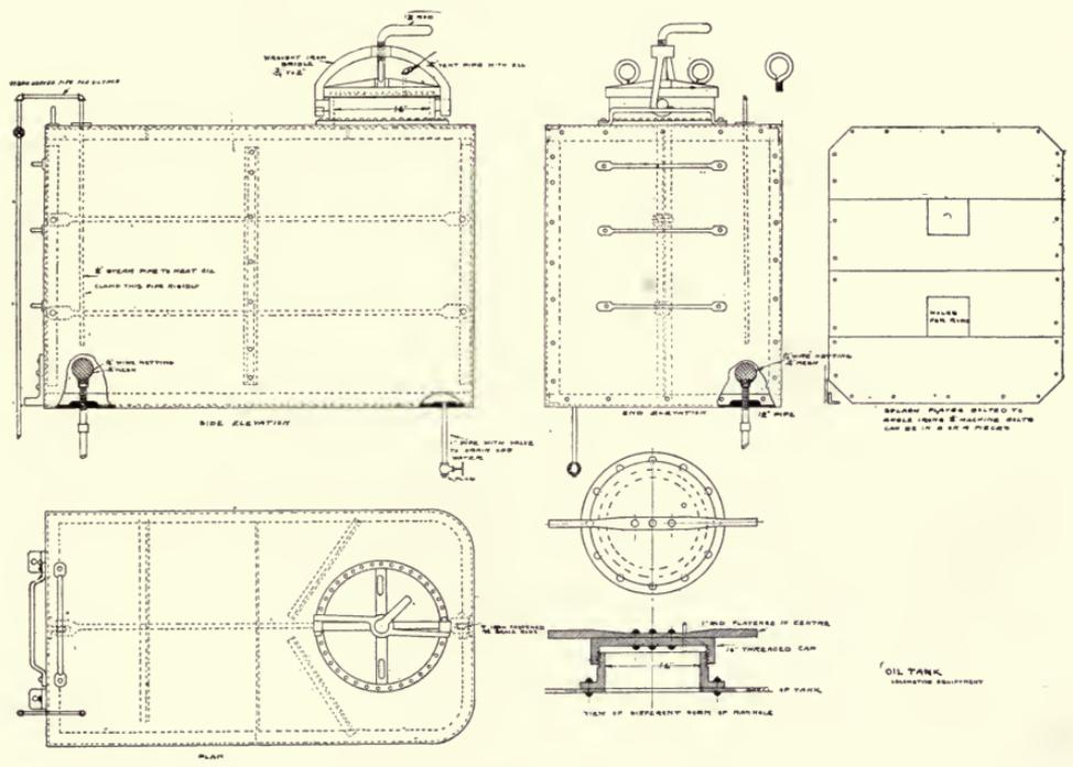
Fig. 5. Oil tank placed in former coal space of locomotive tender.
