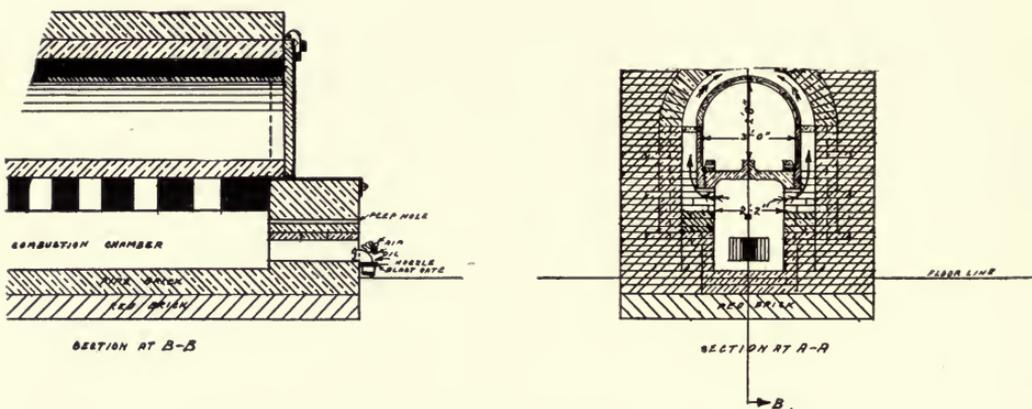
Muffle Furnace for Baking Enamel, Annealing, etc.
