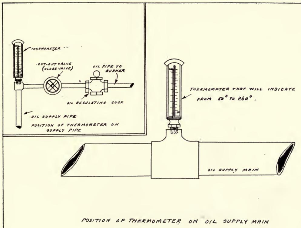
Fig. 1. Above cut illustrates manner of placing thermometers on main oil supply lines or on oil supply pipe to burner.
