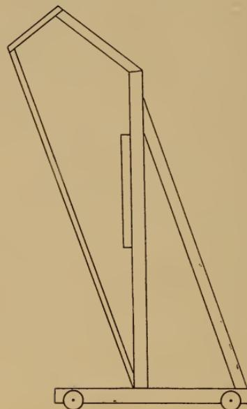
wheels or casters that it may be moved and used in any desirable position in the room. The protection shield for the lights is made part of the framework. See plate A.
