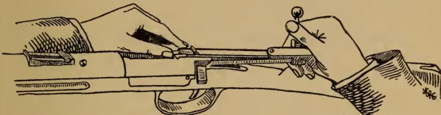
3. Take bolt handle in left hand, back of hand down, bolt upside down. Grasp cocking piece with right hand (Fig. 118).
