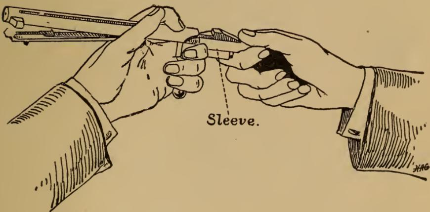
4. Slightly draw back cocking piece and turn it toward the operator until the firing pin can be removed from the bolt.
