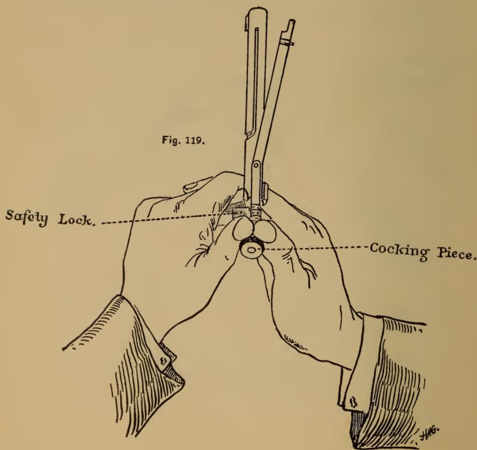
4. Grasp bolt and cocking piece as in third operation for dismounting. Draw back and turn cocking piece from the operator until its nose enters the notch on the rear end of the bolt (see Fig. 118).
