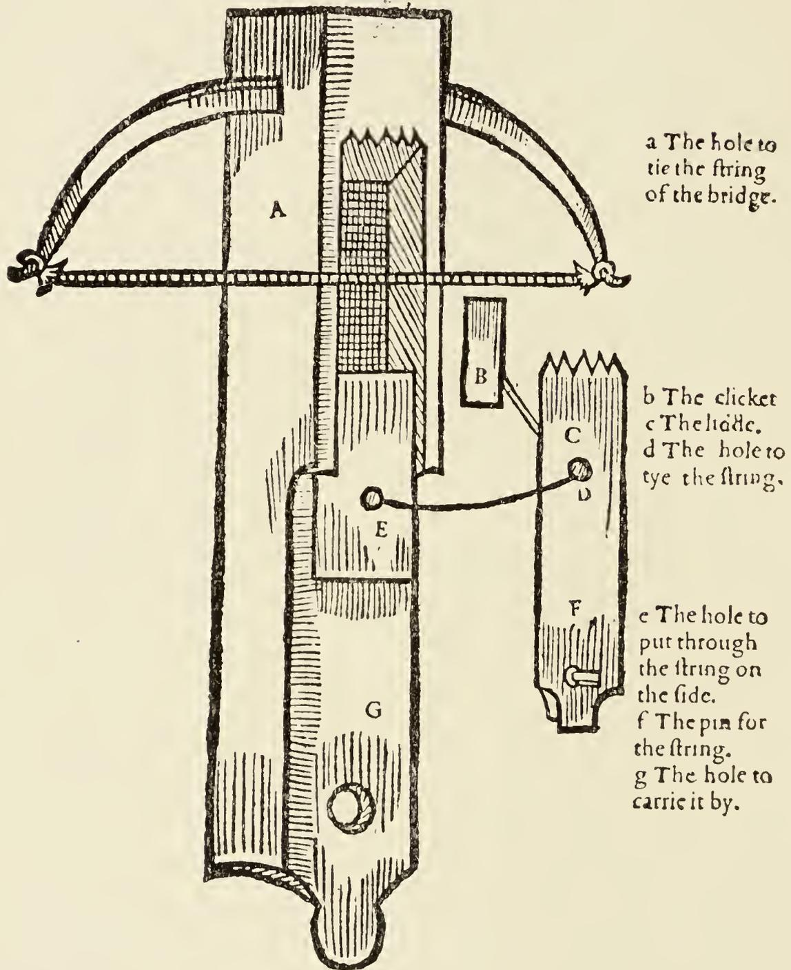
This engine or trappe with the bow, is made like a bore, of a whole peece of wood, with the lidde opening & shutting aboue, and this side is unbent, shewing the left side and the lidde, and clicket, taken out: with holes and the string for to set him, as more plainly shall be shewed bent and set.
