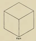
Isometric projection has the appearance of perspective, but no account is taken of the diminishing of the parts with distance. A cube treated isometrically will be as in
