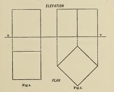
in front of it, will be a square, as in Fig. 4; and its *plan* a square also. Viewed from one of its angles, the representation will be as in Fig. 5. The two views in each case are shown upon the same piece of paper, the space above the line  $x \ y$  representing the vertical plane; that below, the horizontal plane.
