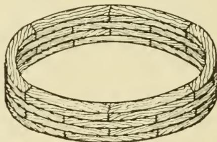
Fig. 32. Example of Building up with Segments.
