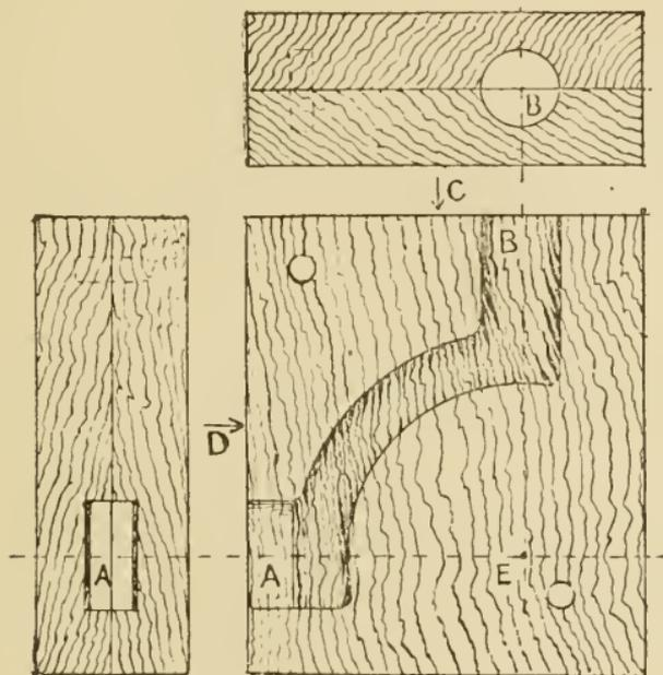
Fig. 48. Core Box for Exhaust Passage.
