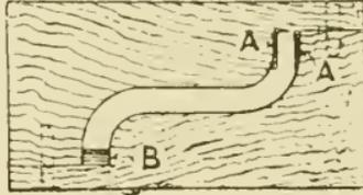
Fig. 47. Core Box for Steam Passage.
