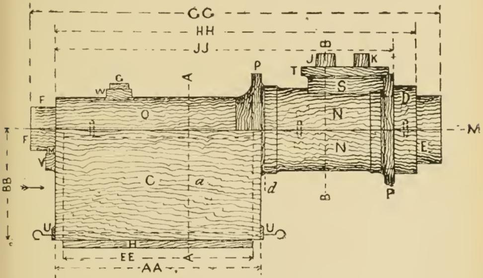
Fig. 41. Cylinder Pattern—Outside View.
