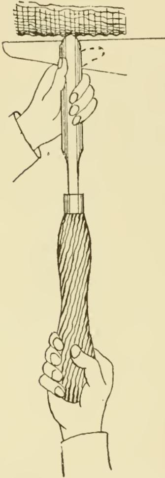
Fig. 89. Method of holding Turning Gouge.
