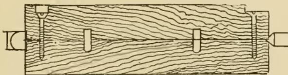
Fig. 99. Jointing for Turning.
