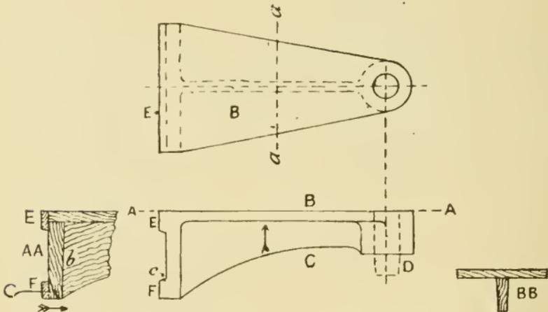
Fig. 5. Casting of a Single Bracket.
