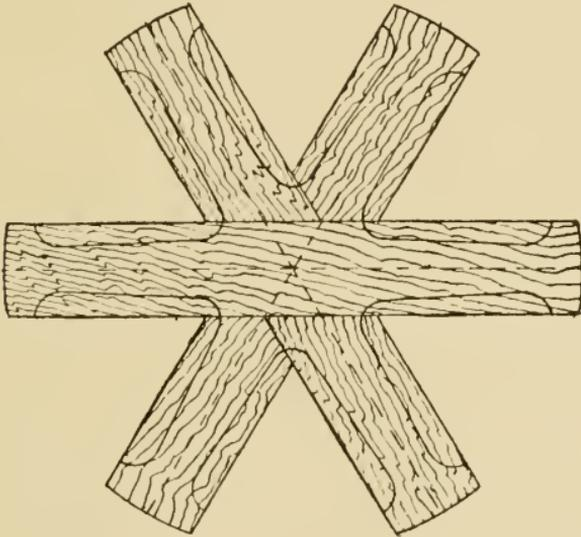
Fig. 57. Wheel Arms, prepared for cutting out.
