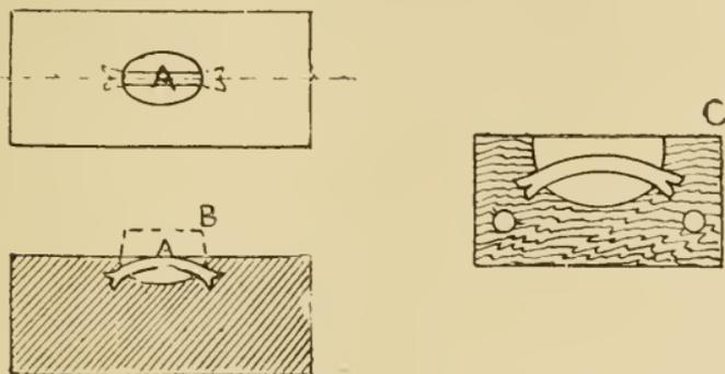
Fig. 18. Casting of Weight with Eye.
