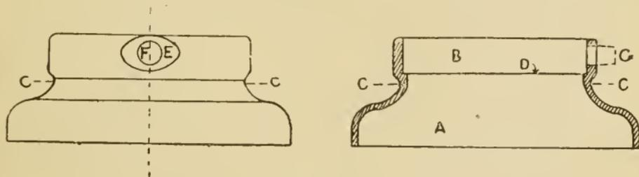
Fig. 14. Casting of Chimney Base.
