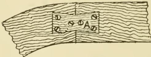
Fig. 36. Dovetailed Fastening.
