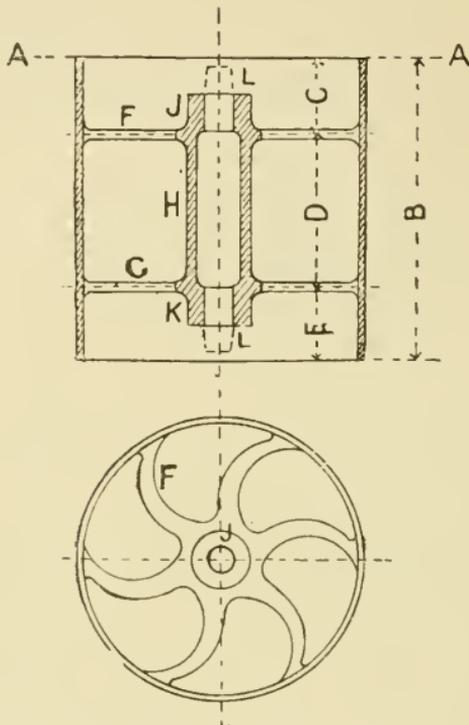
Fig. 12. Casting of Double Armed Pulley.
