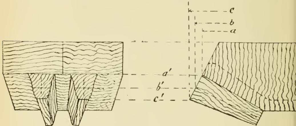
Fig. 68. Tooth Block for Bevel Wheel.
