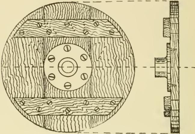
Fig. 97. Face Plate with Battens.
