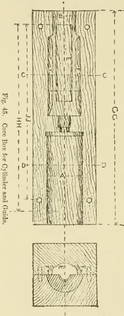
Fig. 45. Core Box for Cylinder and Guide.
