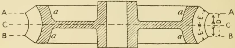
Fig. 9. Casting of a Worm Wheel.
