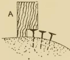
Fig. 81. Gauging "thickness" with nails.
