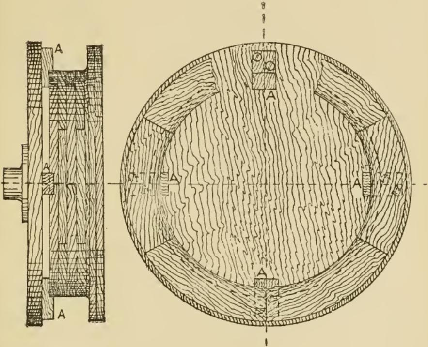
Fig. 96. Chucking with Blocks.
