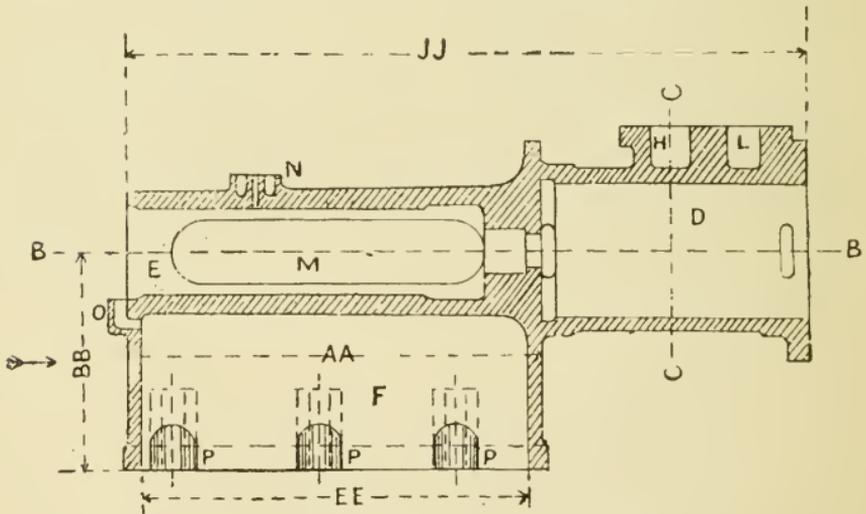
Fig. 37. Cylinder—Sectional Elevation.
