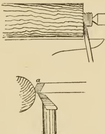
Fig. 91. Chisel turning Perpendicular Faces.
