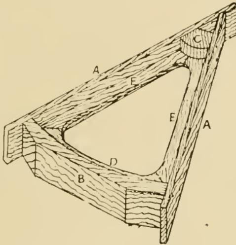
Fig. 67. Core Box for Arms of Cross Section.
