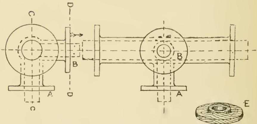
Fig. 13 Casting of Branch Pipe.
