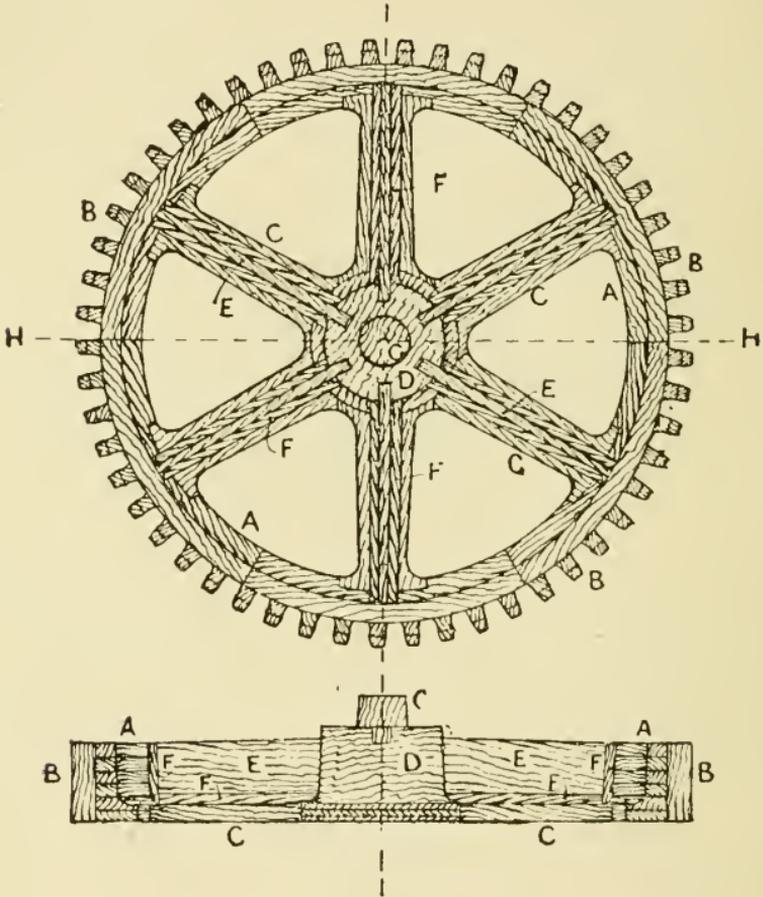
Fig. 56. Pattern for Spur Wheel.
