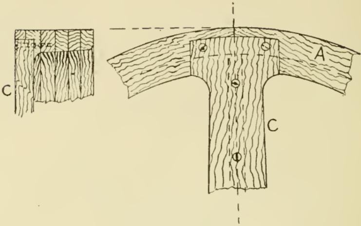
Fig. 58. Attachment of Arm to Rim.
