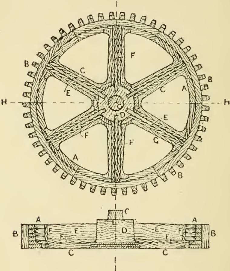
Fig. 56. Pattern for Spur Wheel.
