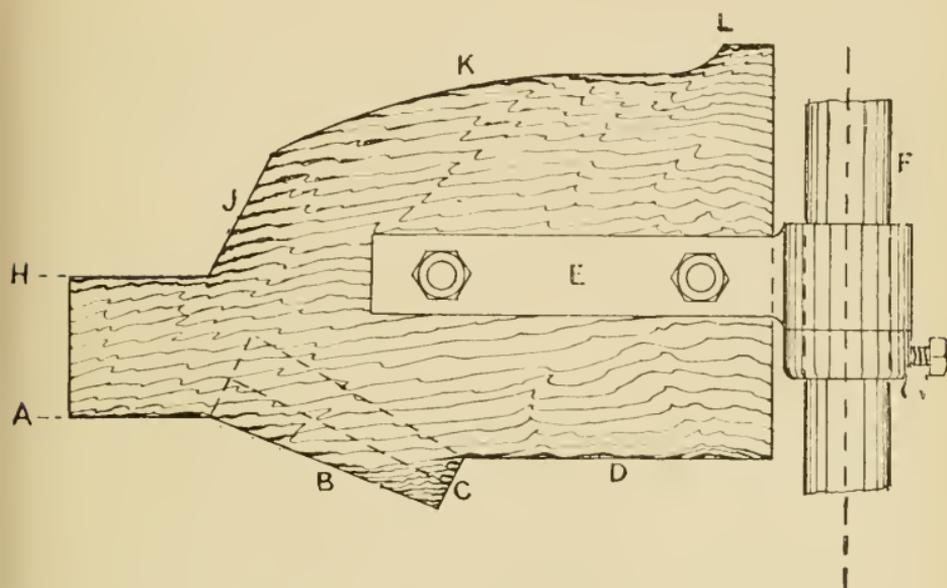
Fig. 69. Board for striking Bed and Cope.
