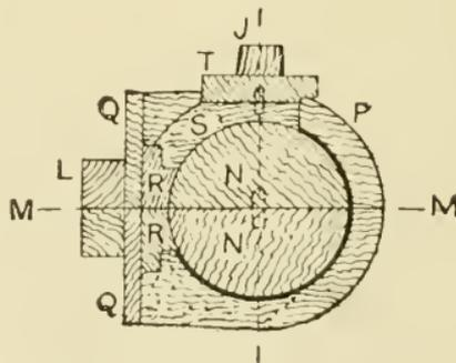
Fig. 44. Cylinder Pattern—Cross Section B-B, Fig. 41.
