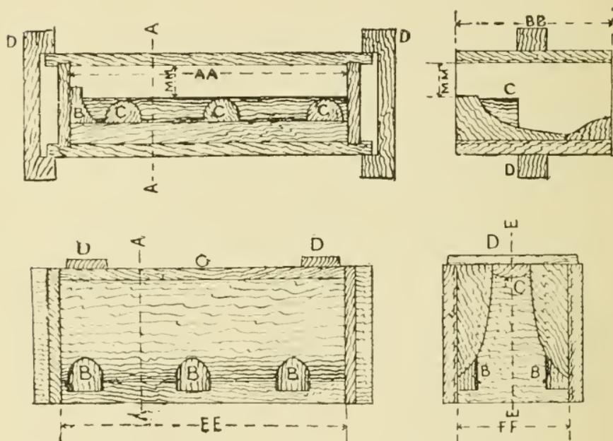
Figs. 49 and 50. Core Boxes for the Cylinder Foot.
