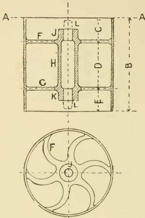
Fig. 12. Casting of Double Armed Pulley.
