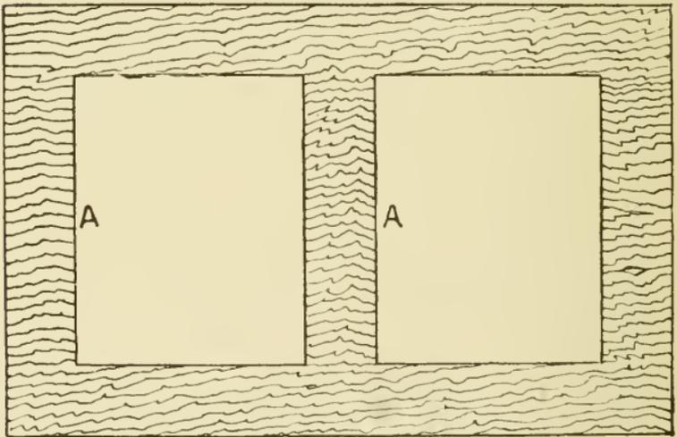
Fig 28. Frame cut from the solid.
