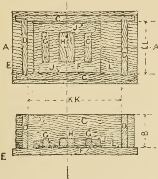
Fig. 46. Core Box for Steam Chest.
