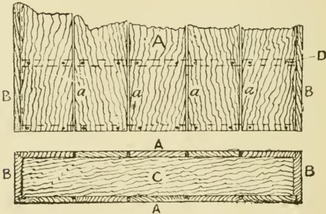
Fig. 20. Open Joints and Boxing-up.
