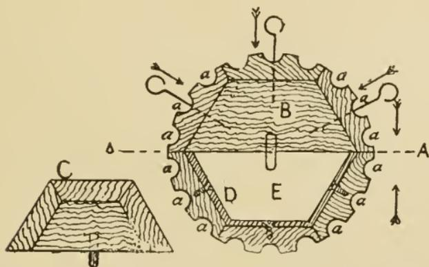
Fig. 25. Example of Loose Lagging for Moulding.
