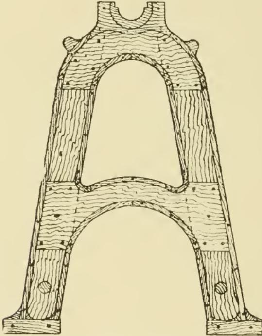
Fig. 30 Pattern of Pump Standard.
