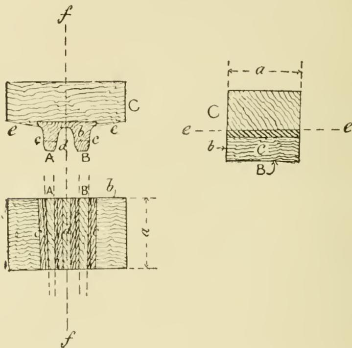
Fig. 63. Tooth Block for Spur Wheel.
