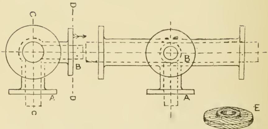
Fig. 13 Casting of Branch Pipe.
