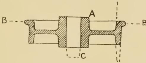
Fig. 7. Casting of a Trolley Wheel.
