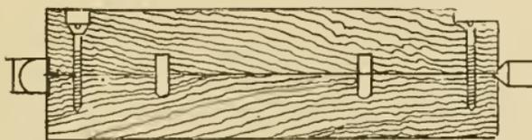
Fig. 99. Jointing for Turning.
