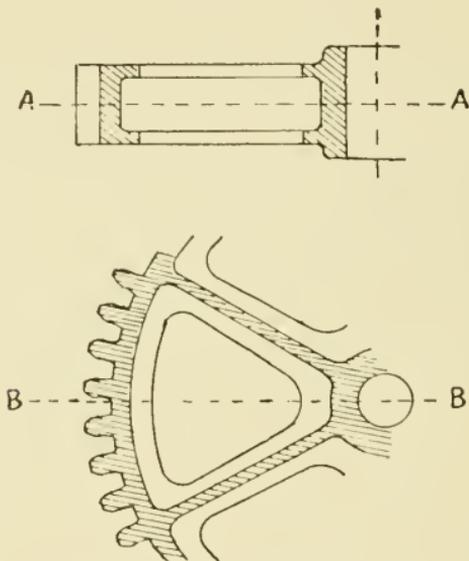
Fig. 64. Wheel with Arms of H Section.
