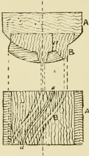
Fig. 72. Tooth Block for Angle Wheel.
