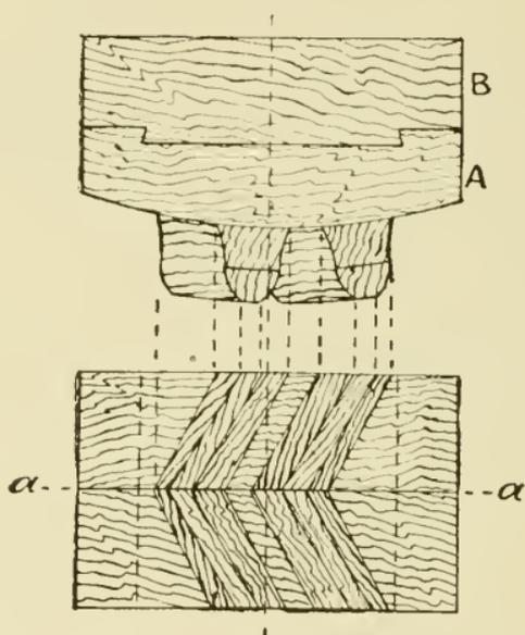
Fig. 71. Tooth Block for Helical Spur.
