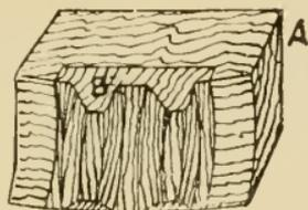
Fig. 73. Tooth Block for Worm Wheel.
