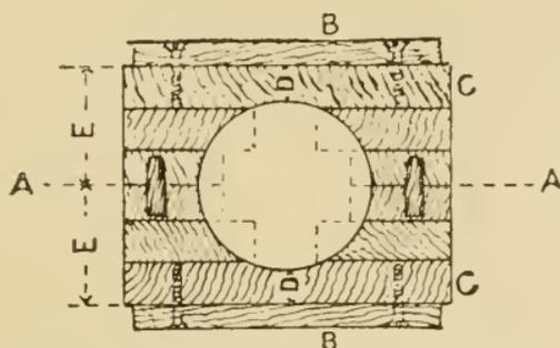
Fig. 26. Section of built up Core Box.
