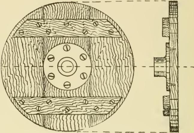
Fig. 97. Face Plate with Battens.
