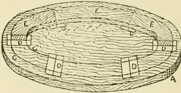
Fig. 53. Method of Building up Segments.
