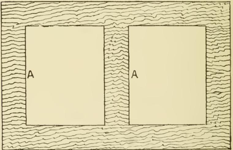
Fig 28. Frame cut from the solid.
