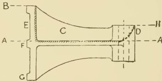
Fig. 6. Casting of a Double Bracket.
