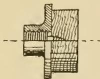
Fig. 93. Taper Screw Chuck.
