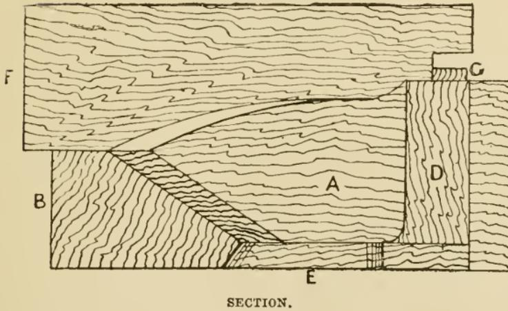
Fig. 70. Core Box for Bevel Wheel.
