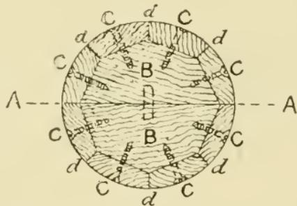
Fig. 24. Example of "Lagging up."
