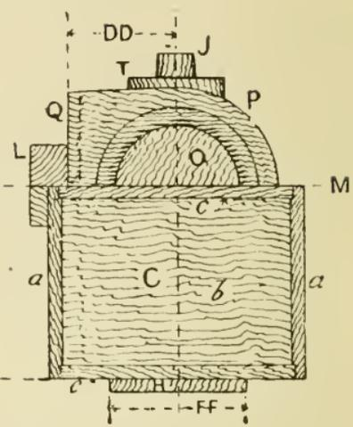
Fig. 43. Cylinder Pattern—Cross
