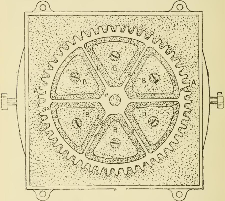
Fig. 66. Cored up Mould of Wheel.
