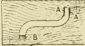
Fig. 47. Core Box for Steam Passage.
