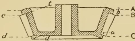
Fig. 11. Casting of Bevel Wheel.
