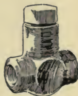
Fig. 35. Ammonia fittings; the cross and the pop safety valve
