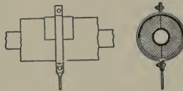
Fig. 84. Typical insulation—brine pipe and hanger
