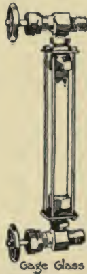
Fig. 42. Ammonia fittings: the gage glass fitted with four rods for protection against accident
